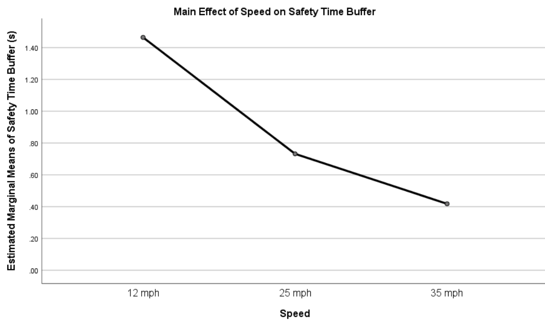
Figure 3.5 The main effect of vehicle speed on safety time buffer, study 2.
