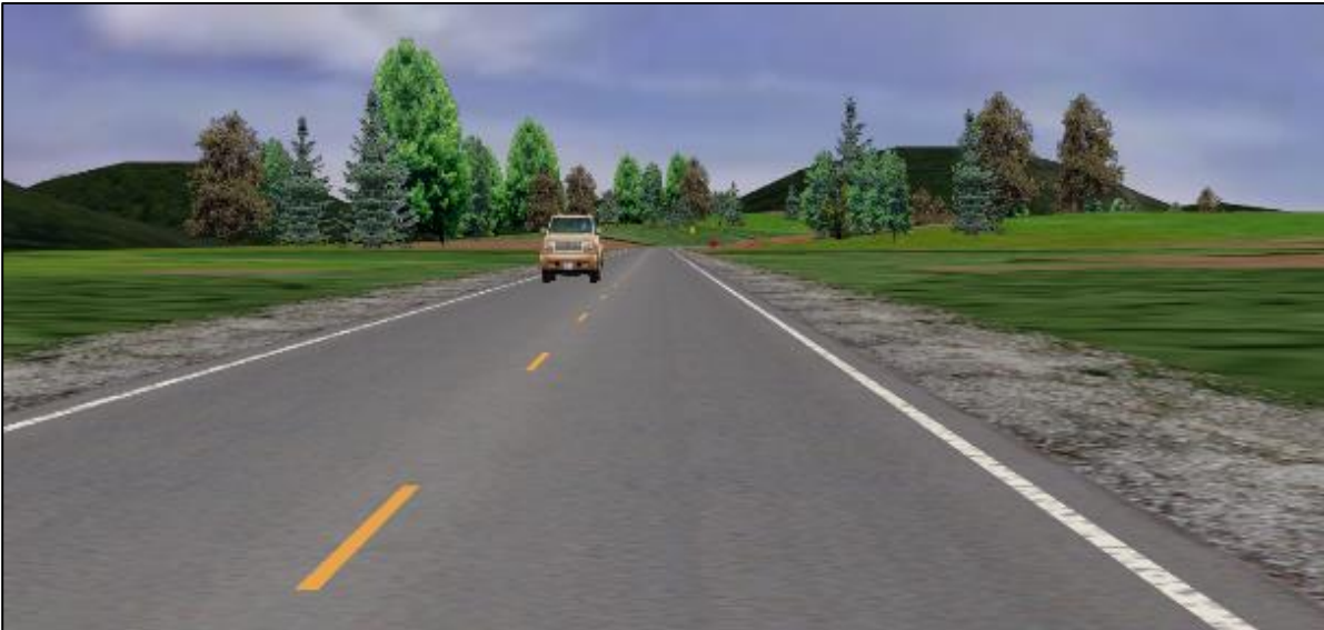
Figure 22: Driver simulation graphic - 6-in edgeline with 25% deterioration
