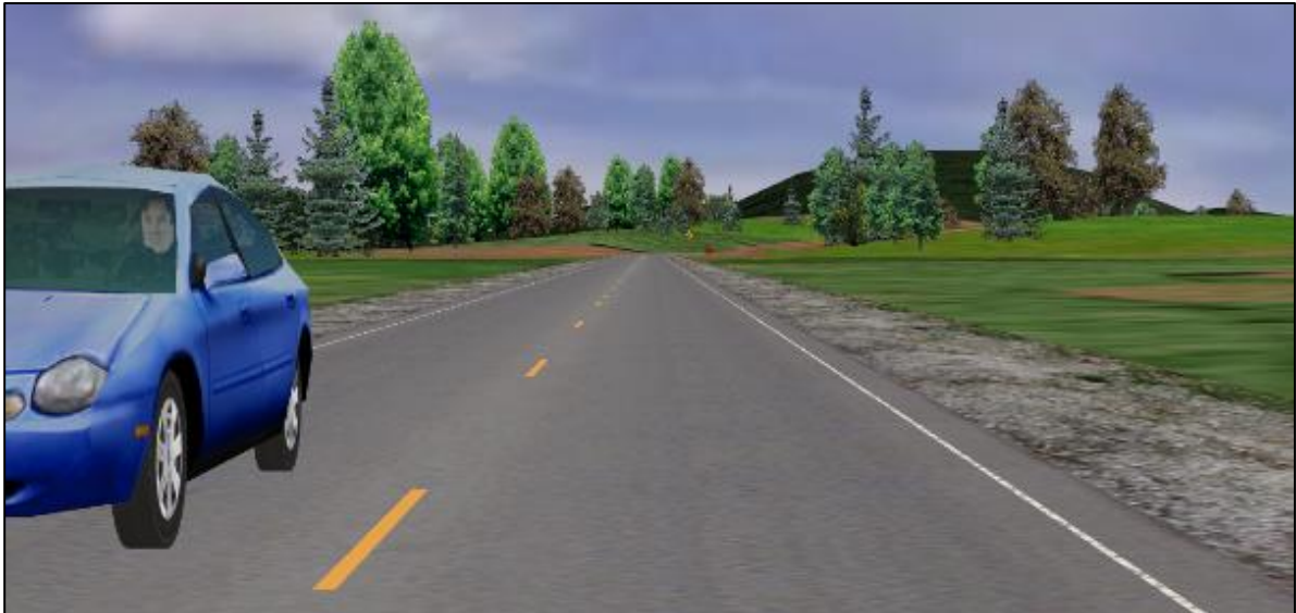
Figure 14: Driver simulation graphic - 2-in edgeline with 25% deterioration
