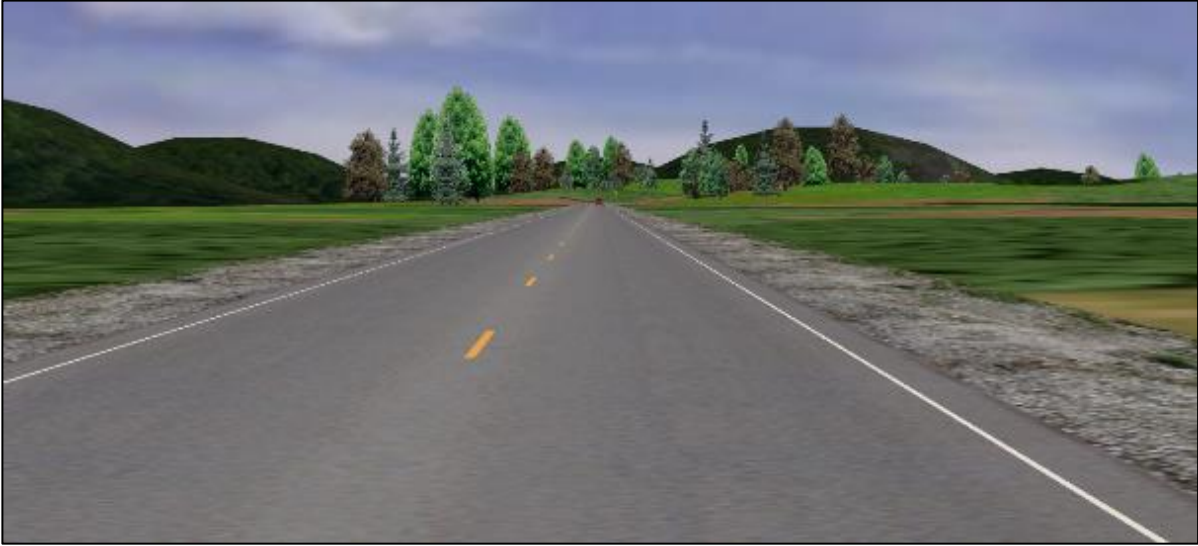
Figure 13: Driver simulation graphic - 2-in edgeline with 0% deterioration
