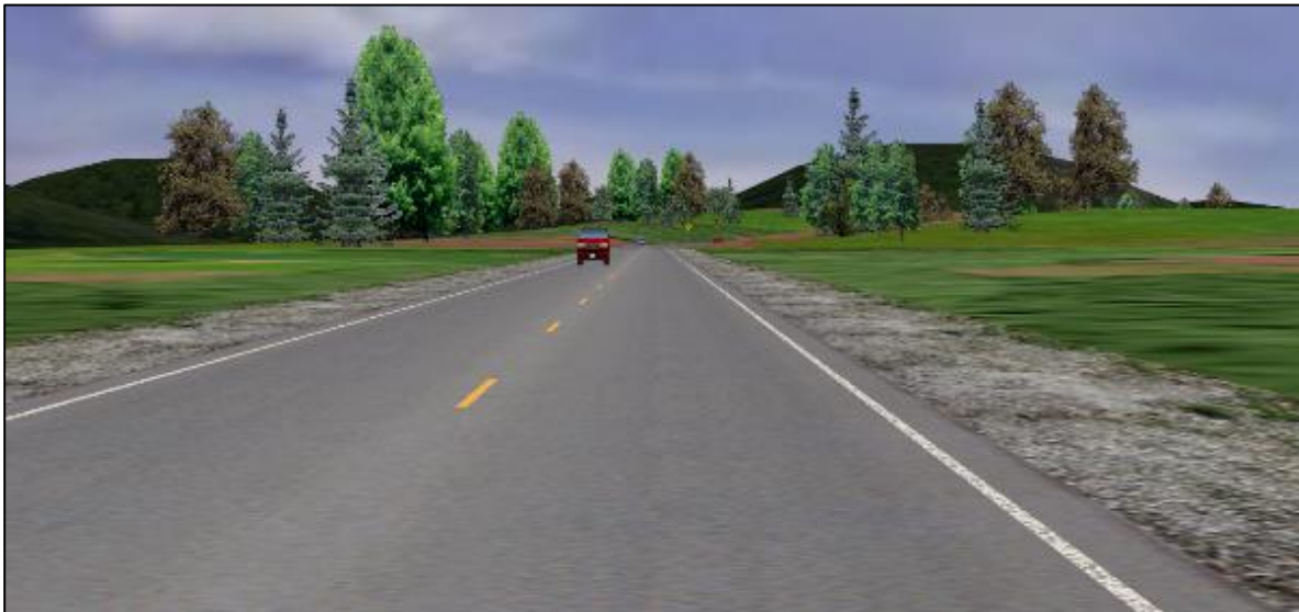
Figure 19: Driver simulation graphic - 4-in edgeline with 50% deterioration
