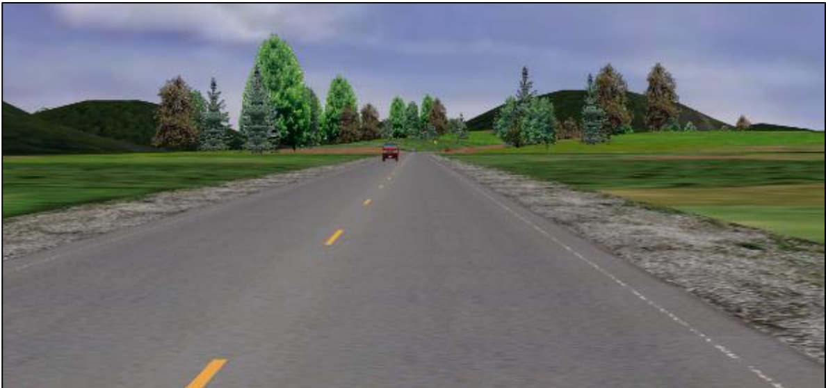
Figure 16: Driver simulation graphic - 2-in edgeline with 75% deterioration
