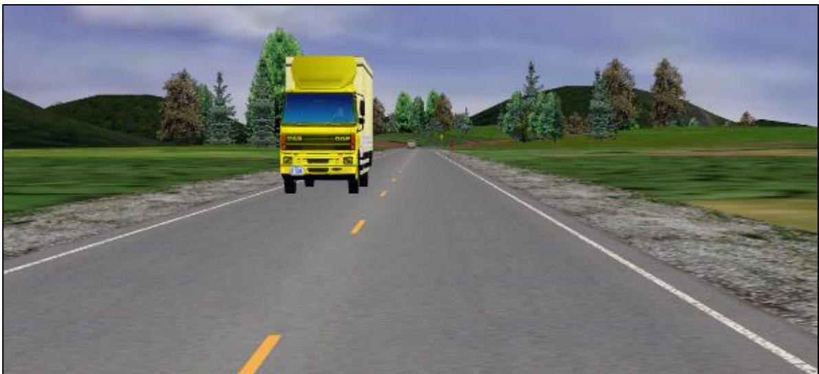
Figure 18: Driver simulation graphic - 4-in edgeline with 25% deterioration
