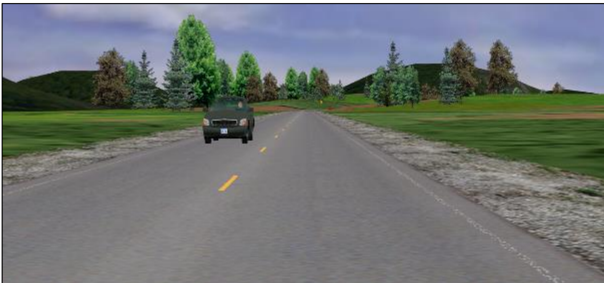
Figure 20: Driver simulation graphic - 4-in edgeline with 75% deterioration
