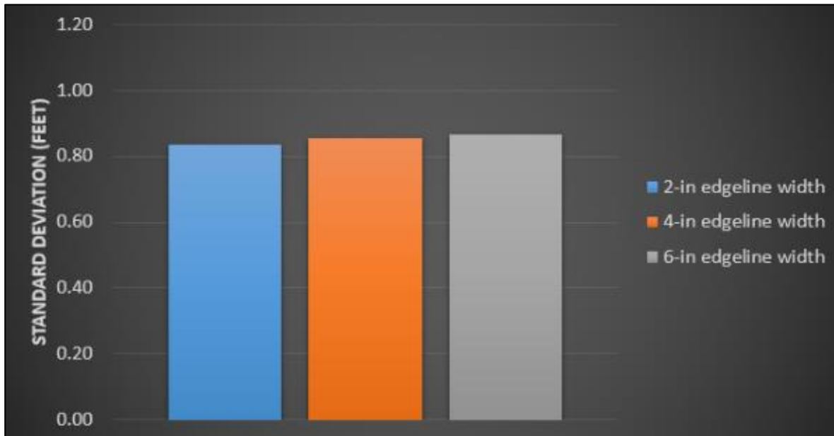
Figure 37: Impact of edgeline widths on lane deviation (standard deviation)
