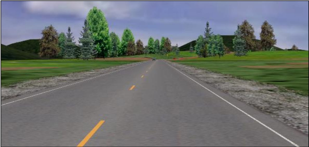
Figure 15: Driver simulation graphic - 2-in edgeline with 50% deterioration
