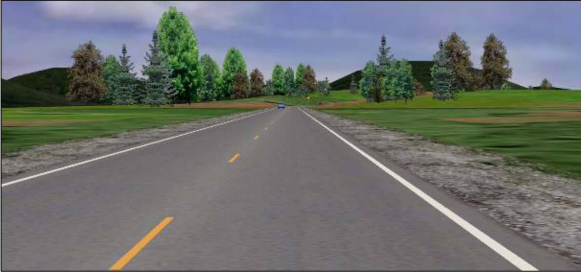
Figure 21: Driver simulation graphic - 6-in edgeline with 0% deterioration
