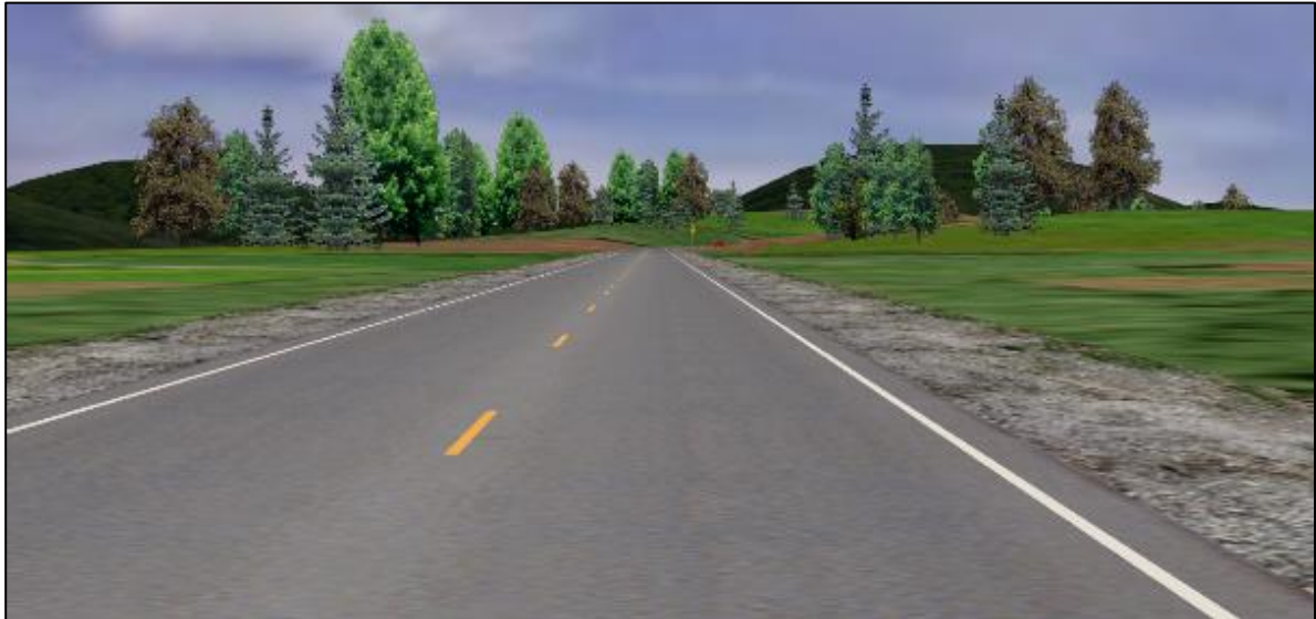
Figure 17: Driver simulation graphic - 4-in edgeline with 0% deterioration
