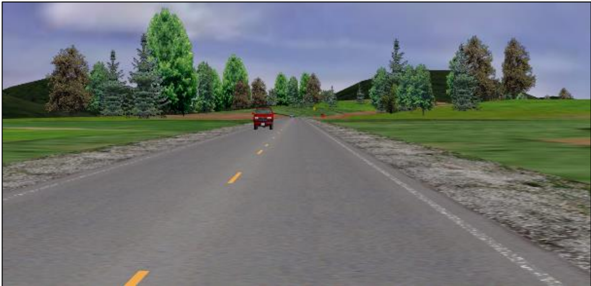
Figure 24: Driver simulation graphic - 6-in edgeline with 75% deterioration
