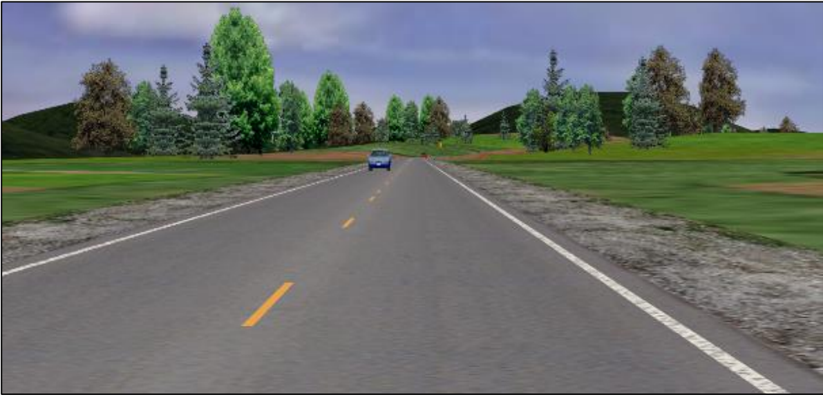
Figure 23: Driver simulation graphic - 6-in edgeline with 50% deterioration
