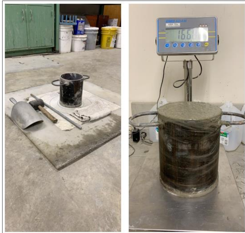
Figure 3-6: (Left) Unit Weight Test Set-Up, (Right) Measuring Unit Weight of Concrete Mix
