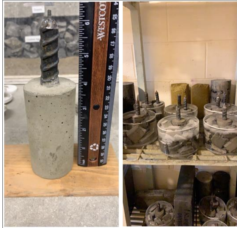
Figure 5-4: (Left) Demolded Macrocell Sample; (Right) Curing of Samples
