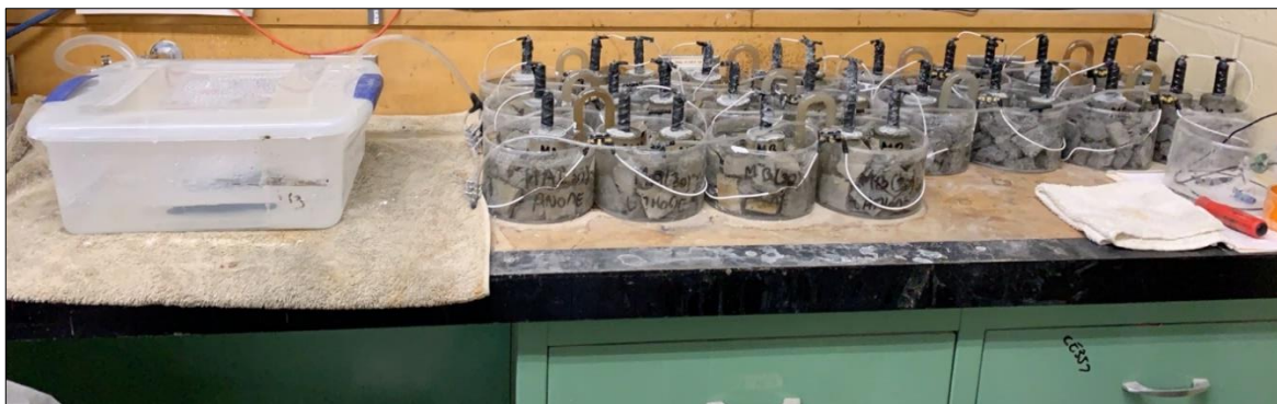
Figure 5-9: Experimental Rapid Macrocell Set-Up
