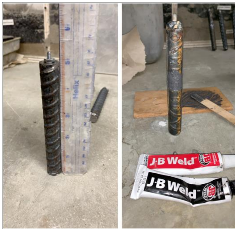
Figure 5-1: (Left) Steel Reinforcement, (Right) Two Part Epoxy Applied on Reinforcement
