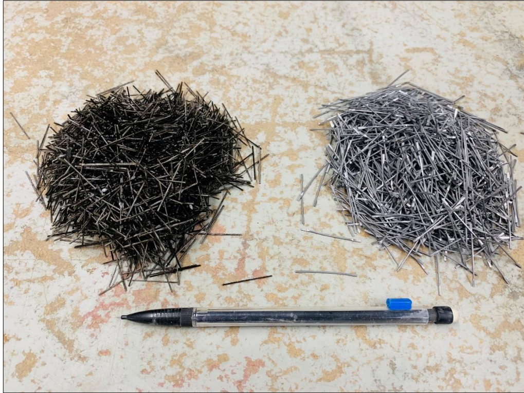
Figure 3-1: (Left) Basalt Fiber, (Right) Steel Fiber (SikaFiber Force XR)
