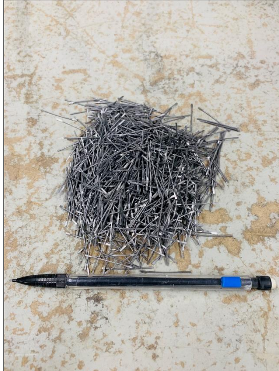
Figure 2-1: Steel Fibers (Authors Figure)
