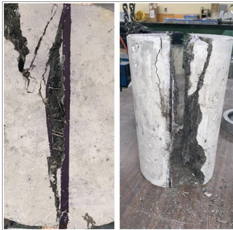
Figure 2-14: (Left) Fiber Bridging, (Right) Typical FRC Cross-Section (Authors Figure)
