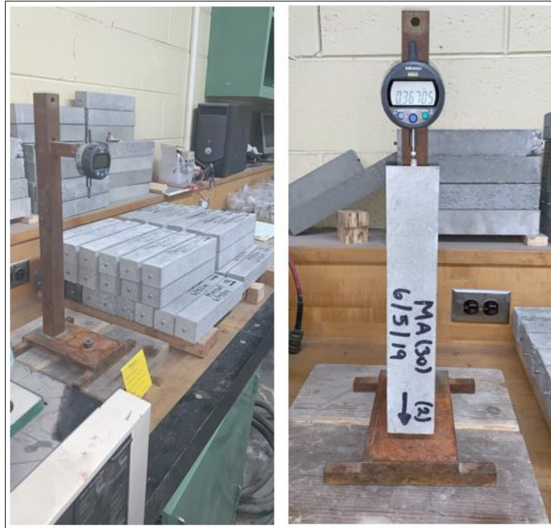
Figure 3-12: (Left) Unrestrained Drying Strength Test Set-Up, (Right) Unrestrained Drying Shrinkage Test Reading
