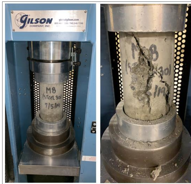
Figure 3-7: Compressive Strength Test Set-Up, (Right) Typical Failure Mode of a Concrete Cylinder Under Compression
