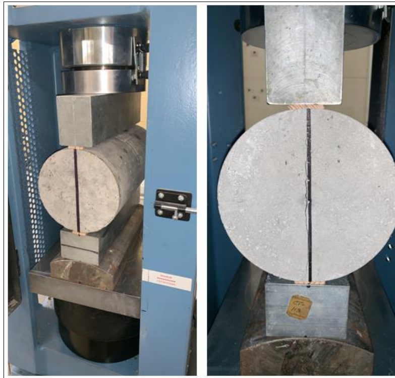
Figure 3-8: (Left) Splitting Tensile Strength Test Set-Up, (Right) Typical Failure Mode of a Concrete Cylinder Under Tension
