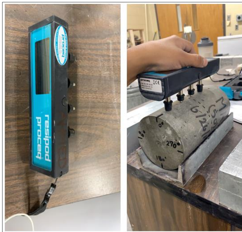
Figure 3-11: (Left) 4-Pin Wenner Probe, (Right) Surface Resistivity Test Set-Up
