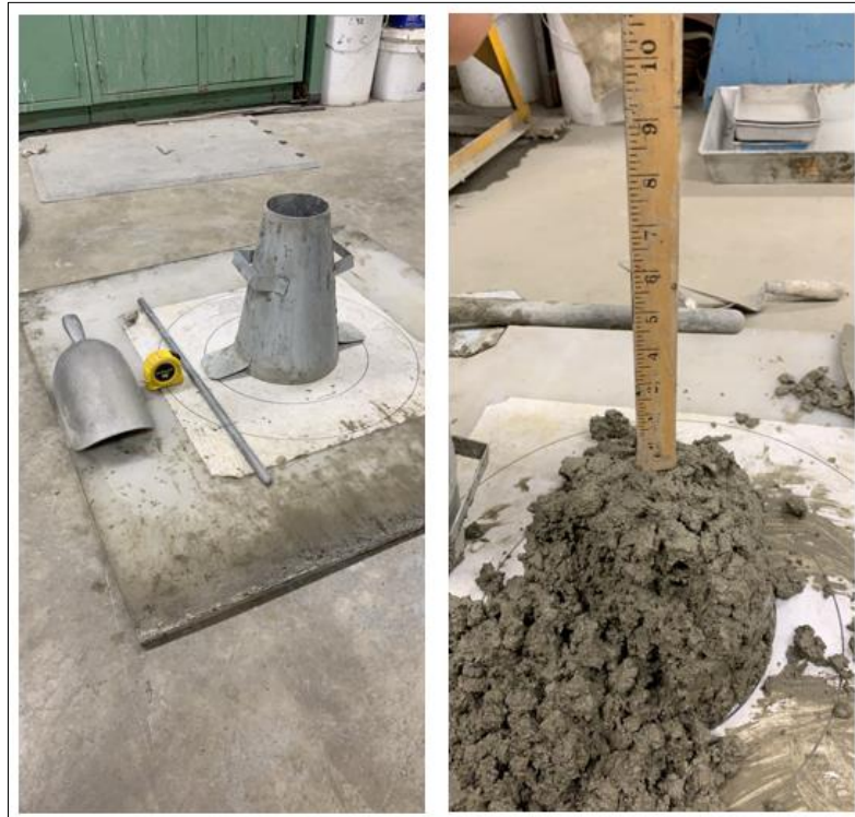
Figure 3-5: (Left) Slump Test Set-Up, (Right) Measuring Slump of Concrete Mix
