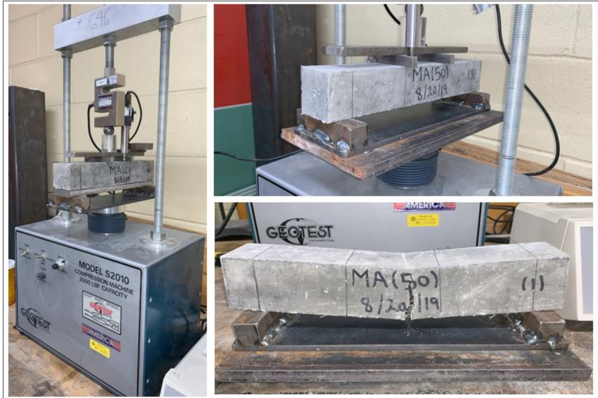
Figure 3-10: (Left) ARS Initial Loading Test Set-Up, (Top Right) ARS Reloading Test Set-up (Bottom Right) Typical Failure Mode of ARS Beam Under Third-Point Loading
