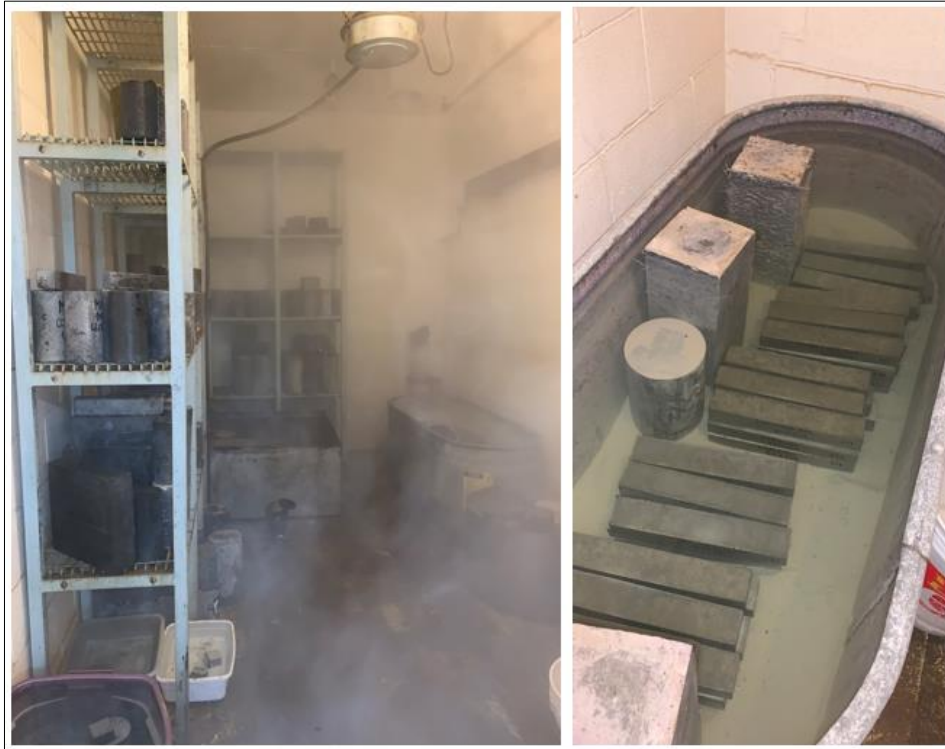
Figure 3-2: Curing Room and Concrete Samples Being Cured in Water Tank
