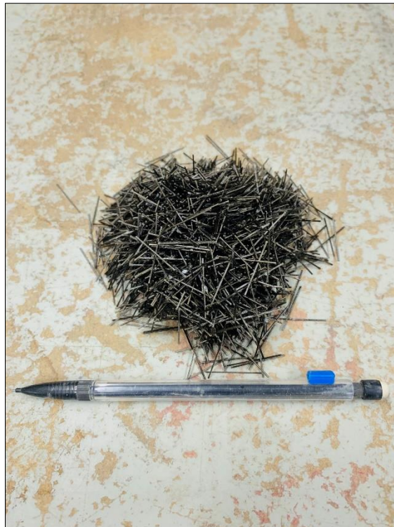
Figure 2-6: Basalt Fibers (Authors Figure)
