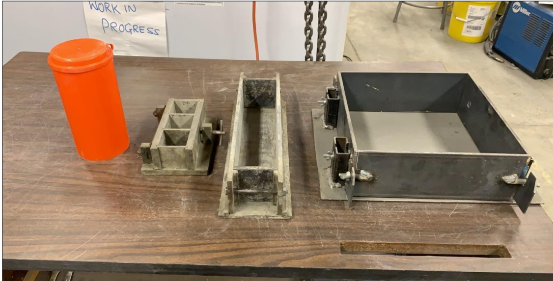
Figure 2-13: Typical Standardized Formwork (Authors Figure)
