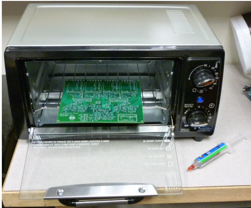
Figure 6.19: Solder Applicator and Solder Reflow Toaster Oven Used for In-House PCB Population
