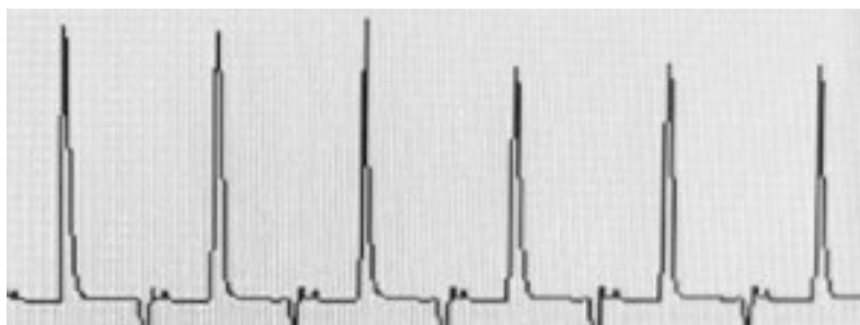
Figure 2.16. Chromatogram of sinalbin hydrolyzed by B. juncea myrosinase. The three peaks on the left are the initial measurements and the three lower peaks on the right are the final measurements.
