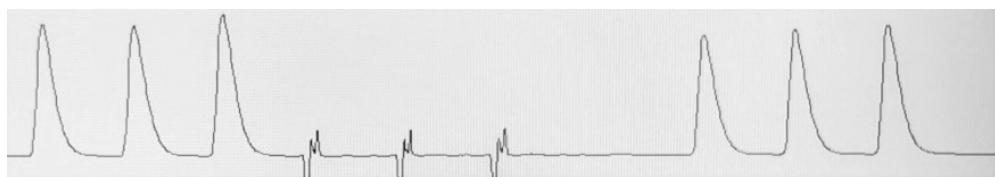
Figure 2.17. Chromatogram of glucolimnanthin hydrolyzed by B. juncea myrosinase. The three peaks on the left are the initial measurements and the three lower peaks on the right are the final measurements.
