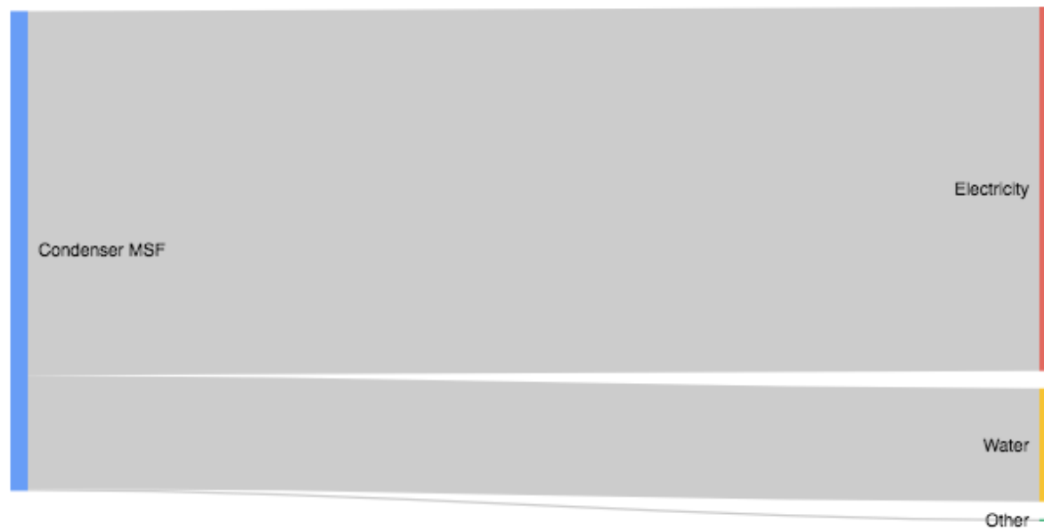
Figure 3.11: The Mass exergy allocation in the configuration with the MSF system after the condenser made using Google Charts
