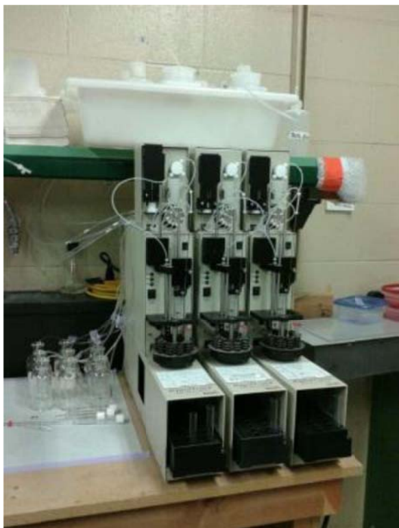
Figure 2: RapidTrace SPE System
