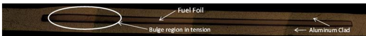
Figure 14. Plate L1P784 montage illustrating bulge in the region near the edges of the fuel foil resulting from fuel relocation caused by fuel creep. The fuel region is 0.75 in. (19 mm) across and the plate average fission density is 5.70 \times 10^{21} fissions/cm 3 .
