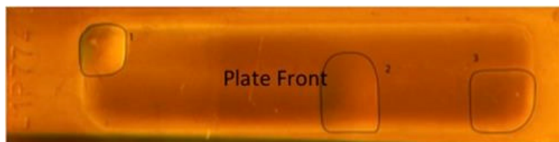
Figure 18. Larger T2 blister types shown for plates L1P774 with an average fission density of 4.78 \times 10^{21} fissions/cm 3 .
