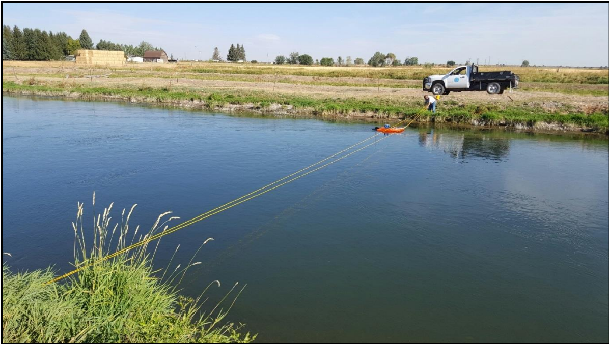
Figure 3.1: Pulley system employed over the Main Canal.
