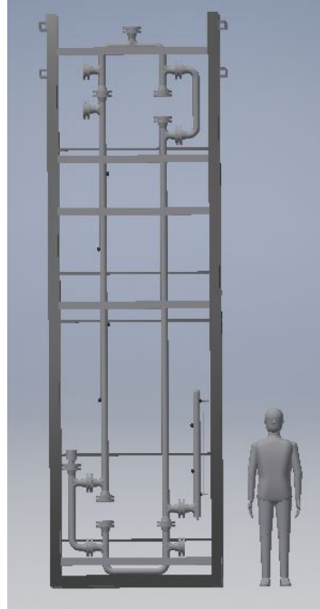
Figure 3.1: Drawing of natural circulation loop and rack.
