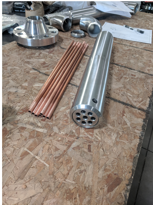
Figure 3.9: Jacket, tube, and bundle plate pieces of heat exchanger prior to welding.
