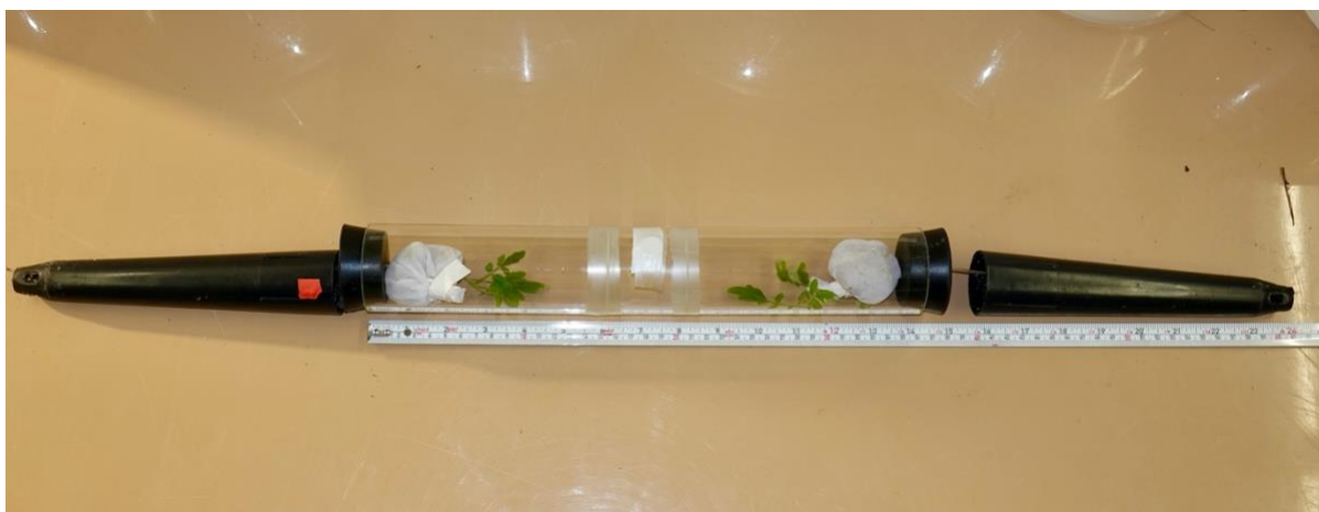
Figure 3. Top view of a two-way choice-test of TSSM olfactometers containing tomato plants, red label indicates the position of the RKN inoculated plants.
