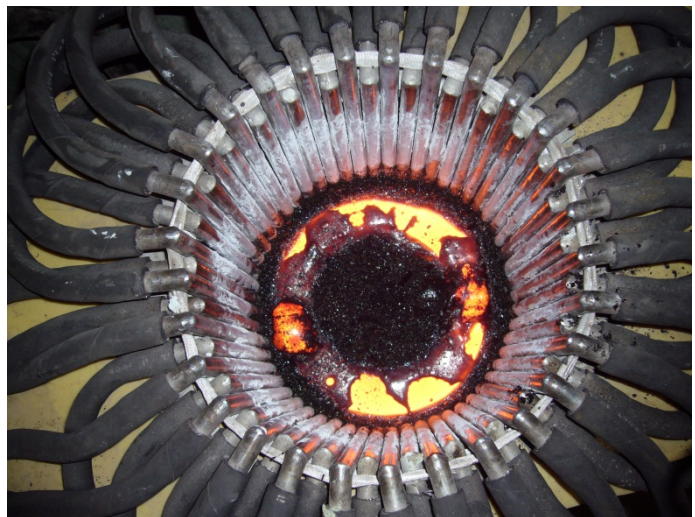
Figure 5-1. Graphite initiator ring during melt start-up.
