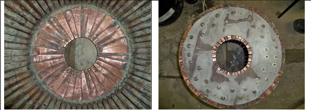
Figure 11-30. Top and bottom views of the new bottom with 32 segments, during assembly.
