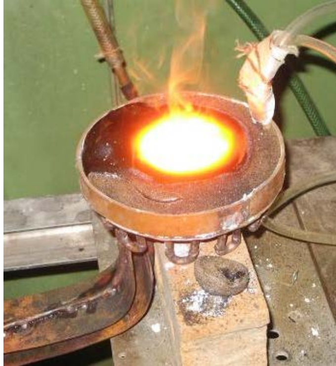
Figure 8-24. View of drain assembly during melt initiation for Drain Test #8.
