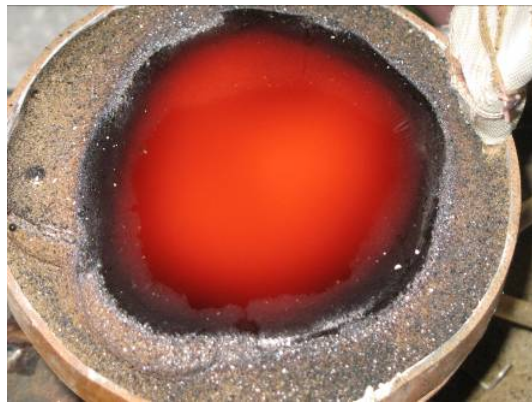
Figure 8-25. View of maximum melt pool achieved during Drain Test #8.
