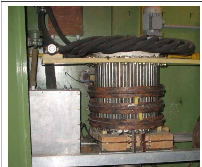
Figure 2-10. Three-turn CCIM test platform.
