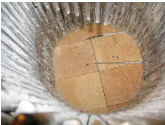
Figure 7-13. CCIM Test #5 thermocouple placement on the bottom surface.
