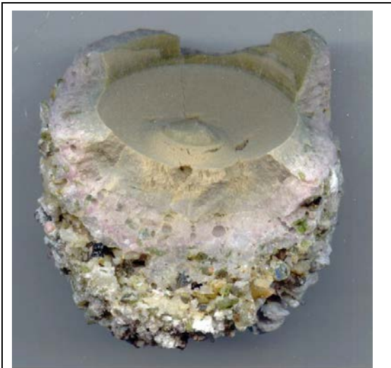
Figure 8-4. ZrO_2 ingot resulting from Drain Test #2.
