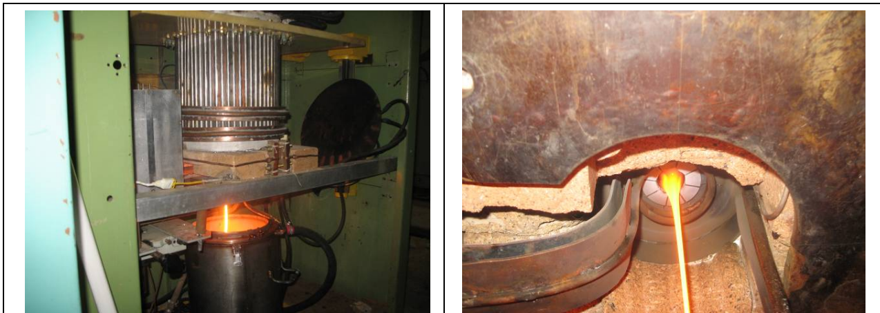
Figure 9-26. Comparison of pour stream diameter at high power (left) and low power (right) settings on 27 MHz generator.
