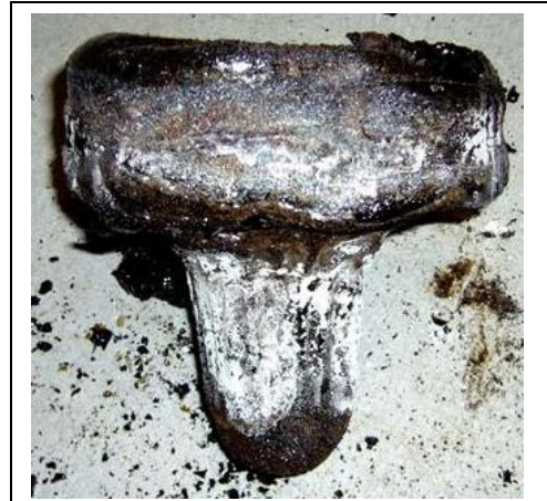
Figure 8-20. Ingot from Drain Test #7.
