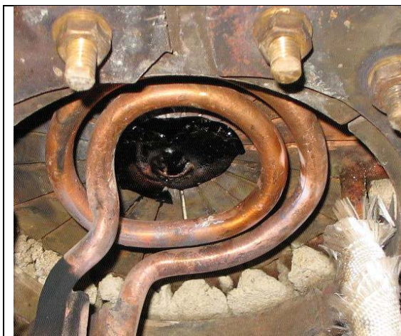
Figure 11-18. View of softened bulging from drain opening after third casting attempt.
