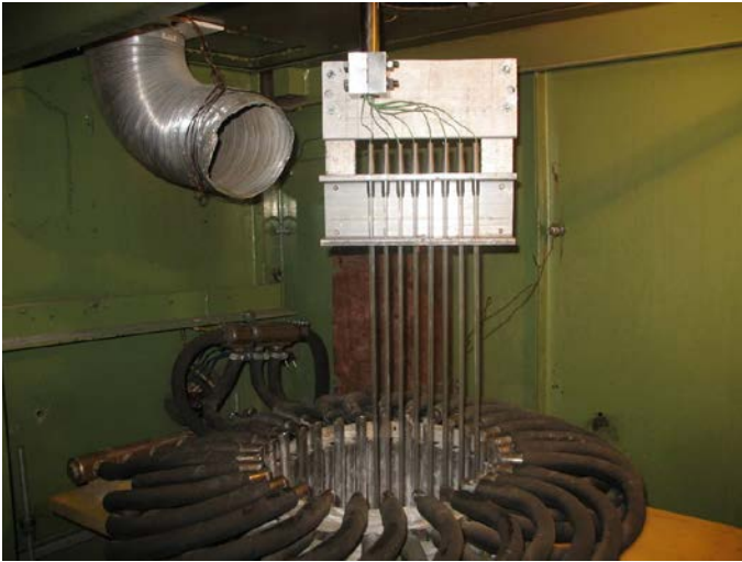
Figure 7-12. CCIM Test #5 Pt-Pt/Rh thermocouple array.
