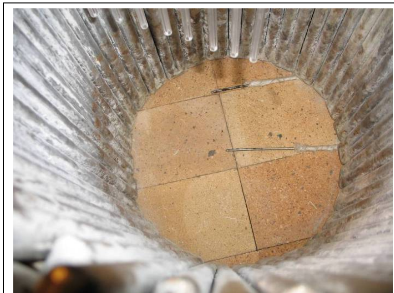
Figure 2-8. Placement of thermocouples in melter bottom to determine heat flux.
