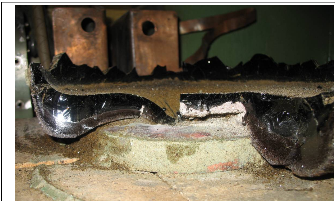
Figure 9-9. Ingot after disassembly showing three phases of glass product.
