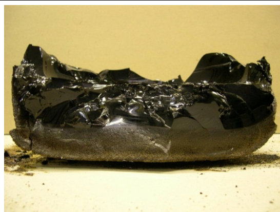
Figure 7.3b. Cross-section of ingot from CCIM Test #1.
