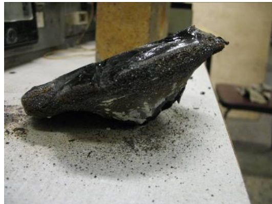
Figure 8-26. View of ingot obtained during Drain Test #8.
