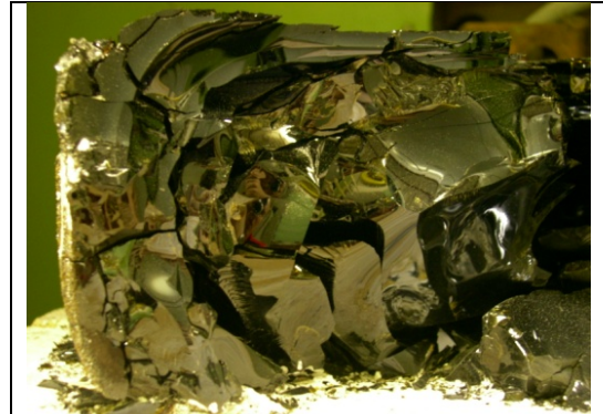
Figure 3-29. Crystalline phase resulting from interaction with ceramic base.
