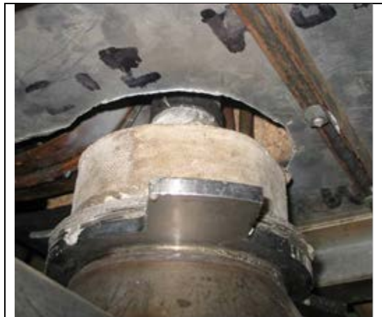
Figure 10-5. Ceramic tube reducer connecting drain opening to receipt container in a leak-tight environment.
