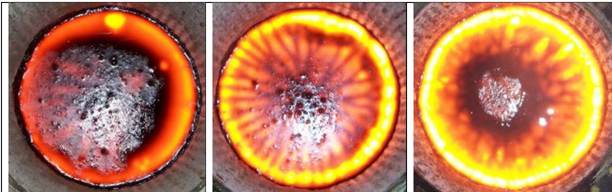
Figure 2-17. Comparison of three different steady state modes established for emissivity determination. Notice the obvious difference in average surface temperature (see Table 2-8).
