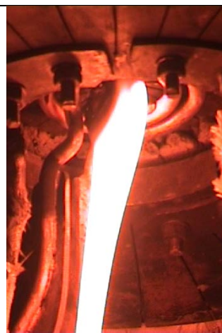
Figure 11-19. Pour stream during second casting contacting inductor.
