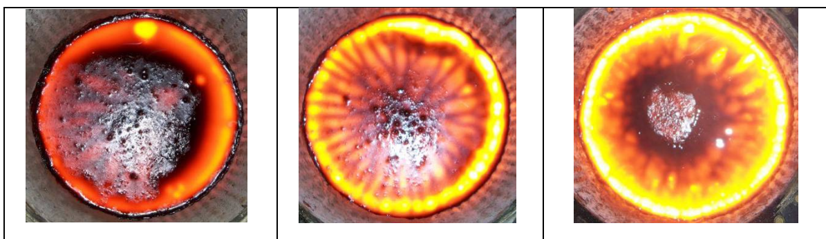
Figure 11-4. Steady state modes evaluated during System Optimization Test #1a. Left - 1,030°C, Center - 1,190°C, Right - 1,230°C
