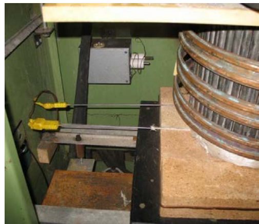
Figure 7-13. CCIM Test #5 thermocouple placement on the bottom surface.
