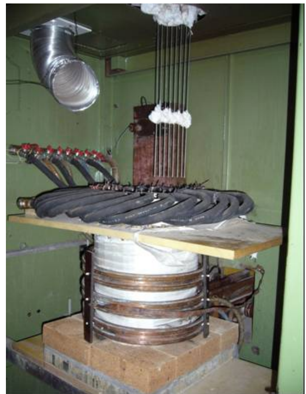
Figure 3-30. Three-turn inductor test configuration with eight thermocouple array.
