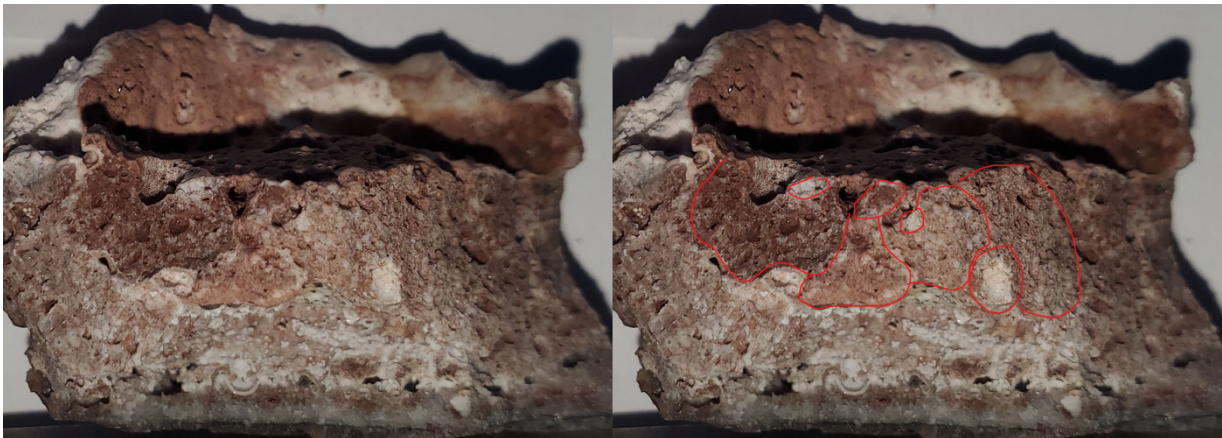
Figure 4.11: A larger view of the color variations within sample C. On the right is a duplicate picture, with markings identifying different zones of color.
