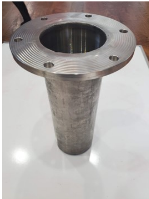
Figure 3.1: Initial melting vessel, constructed from a nickel-200 pipe with a nickel plate welded to the bottom, and a SS-316 flange welded to the top.
