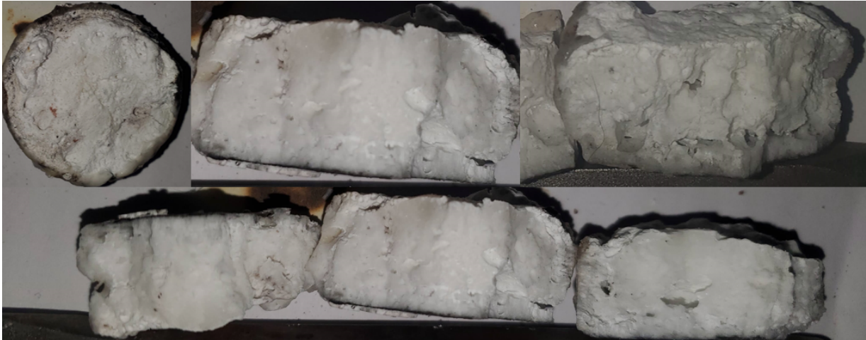
Figure 4.9: Pictures of extracted samples A and AA. The top right photo is sample AA, and the remaining photos are sample A. These samples were both pure Flinak, with no added corrosion products.
