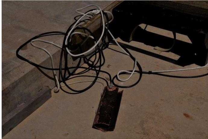
**Figure 2.10:** Copper plate used to create desired electric fields
