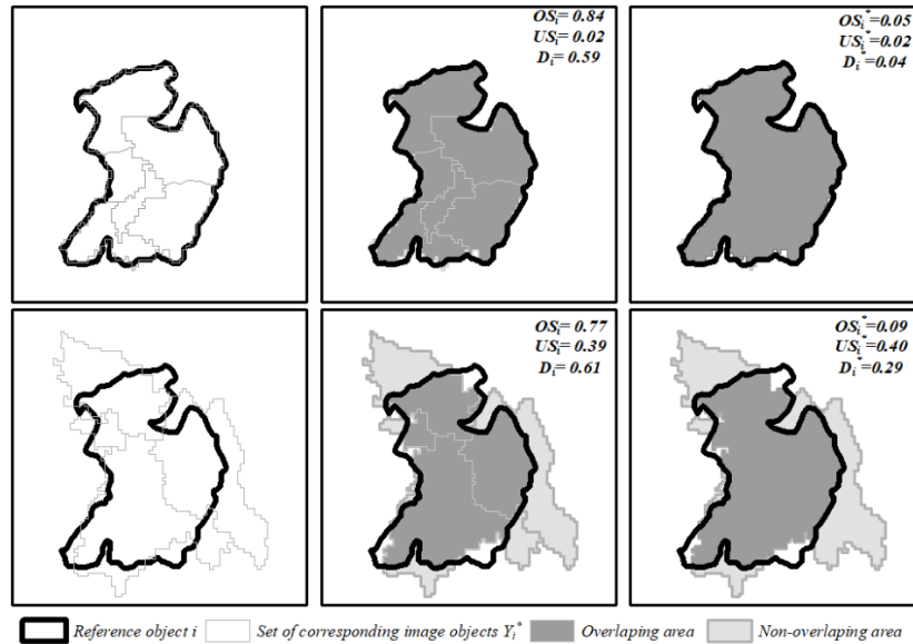
Figure 1.5. Illustration of the area-based dissimilarity metrics ( OS_i, US_i, D_i ), and of the modified metrics ( OS_i^*, US_i^*, D_i^* ). A reference object x_i , (black vectors) is displayed together with its corresponding set of image objects (gray vectors): The top row shows an example where the reference object is oversegmented, but not undersegmented (i.e., it is closely matched by the union area \cup_{y_j \in Y_i^*} y_j ); the bottom row shows an example where the reference object is both oversegmented, and undersegmented. The center column illustrates the traditional oversegmentation ( OS_i ), undersegmentation ( US_i ) and summary score D_i for that single reference object, metrics that consider each individual corresponding image object. The right column illustrates the modified OS_i^*, US_i^* , and D_i^* metrics, that consider instead the union area of all corresponding image objects. The summary score D does not report a significant difference between the two classifications (top: D_i = 0.59 , bottom: D_i = 0.61 ), whereas the modified summary score D^* indicates that through post-processing the top row segmentation could result in a near-perfect match with the reference object ( D_i^* = 0.04 ), whereas significant errors will remain in the bottom row segmentation ( D_i^* = 0.29 ).
