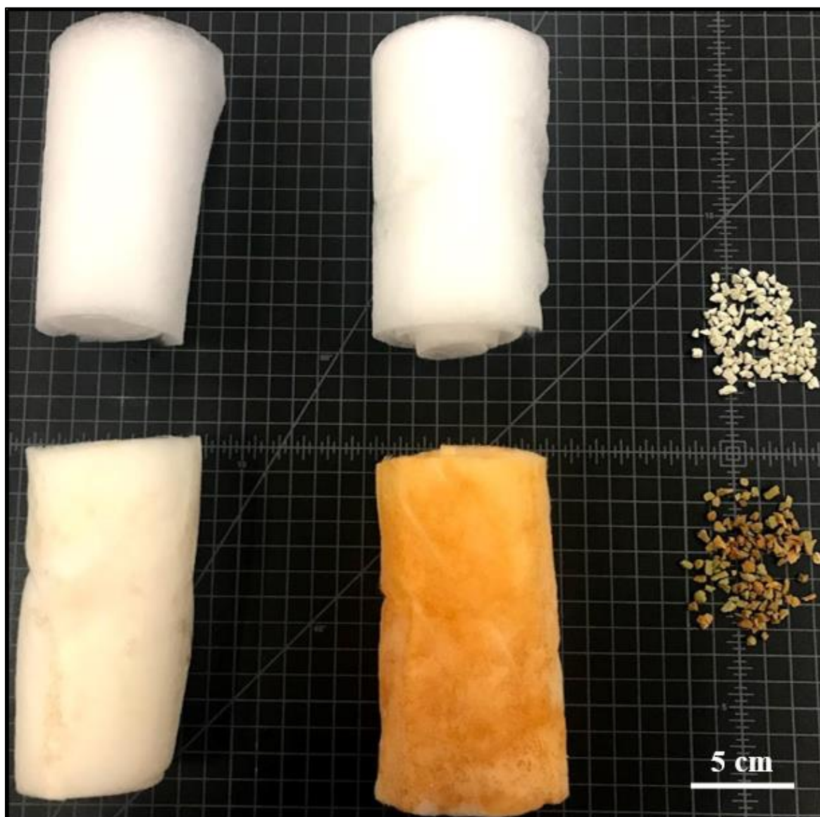
Figure 2.9. (Left to right) 12 g of Si, 12 g of Si+APTES, and 5.4 g of clinoptilolite before (top row) and after (bottom row) batch sorption experiments. Orange color is due to sorbed/precipitated iron-(oxyhydr)oxides.
