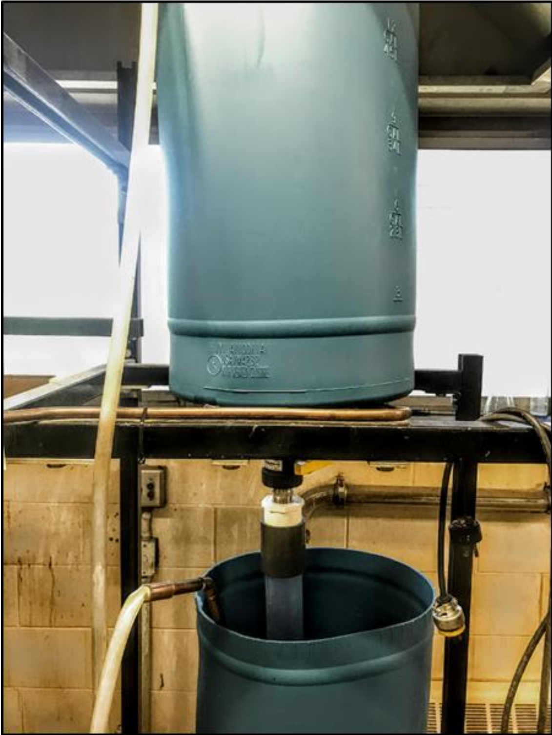
Figure 2.4. Laboratory setup for permeability column experiments.
