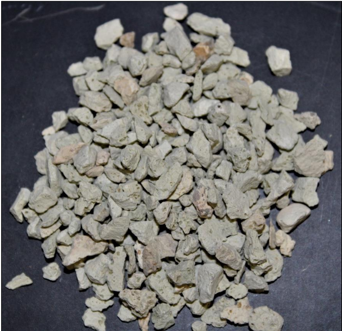
Figure 2.3. Clinoptilolite grains, 2.4 to 4.8 mm diameter (4×8 mesh).
