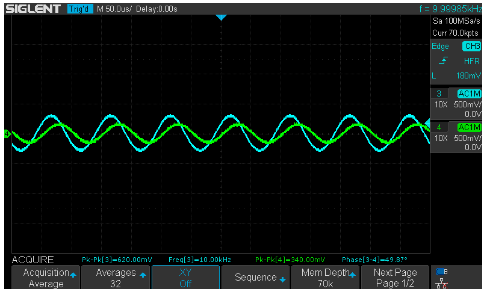
Figure B.9: 41 Turn, 50mm diameter, Test Reactor Module with 10Ω Current-Sensing Resistor in-series.
