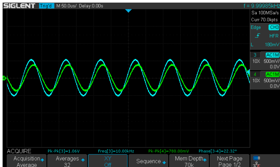
Figure B.16: 41 Turn, 50mm diameter, Test Reactor Module with 10Ω Current-Sensing Resistor in-series, with turn 21 shorted. |V_{pk-pk}| = 1.06V , f = 10kHz , |I_{pk-pk}| = 78.0mA , \Phi_{V-I} = 22.32^\circ
