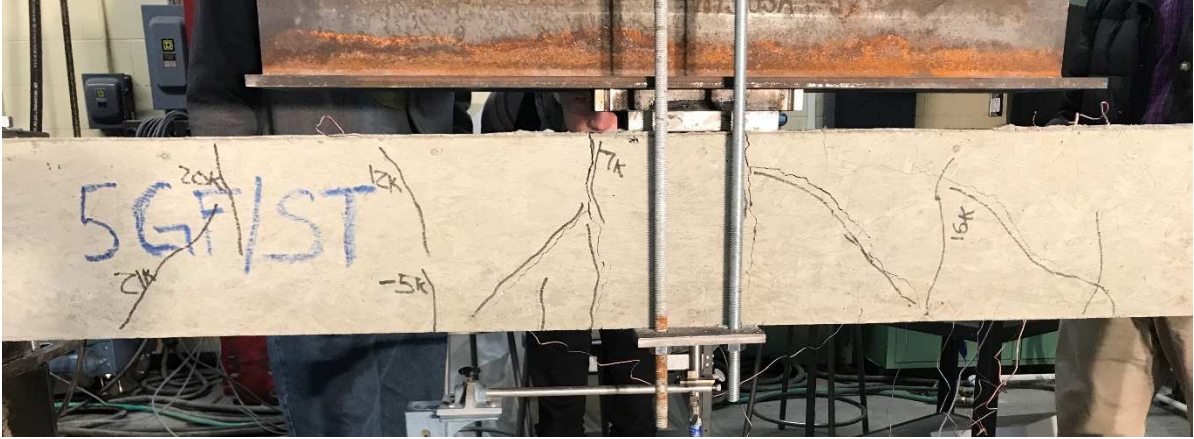
Figure 4-14: Beam 5 GF/ST Hybrid Cracked
