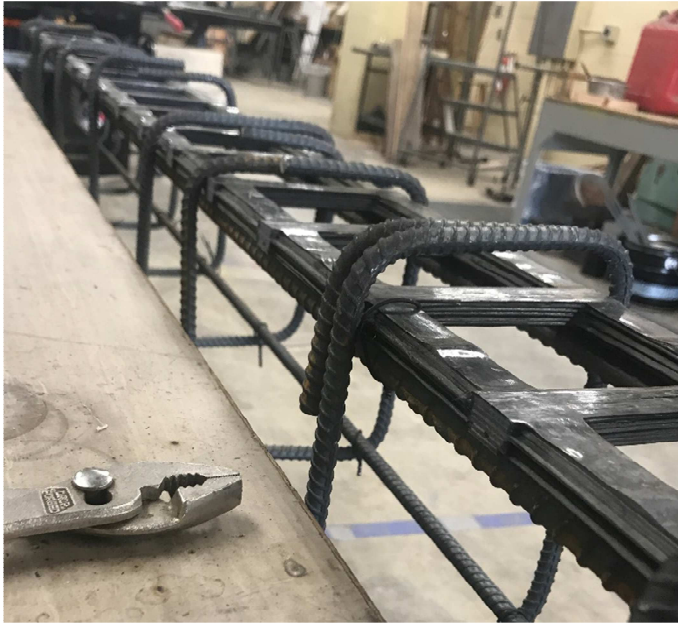
Figure 3-4: 4 CF/ST Hybrid Reinforcement Cage Close-up
