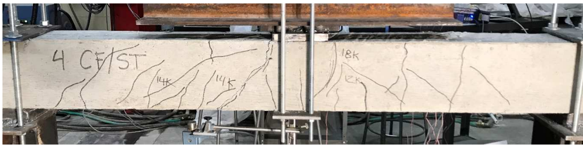
Figure 4-11: Beam 4 CF/ST Hybrid Cracked
