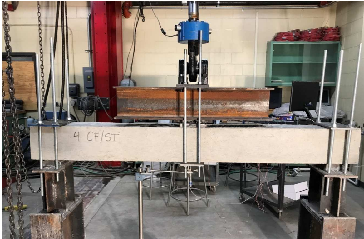
Figure 3-12: Set-up for One Concrete Specimen (Beam 4 GF/ST)
