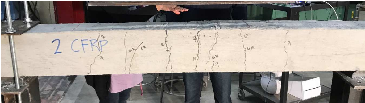
Figure 4-5: Beam 2 CF Cracked
