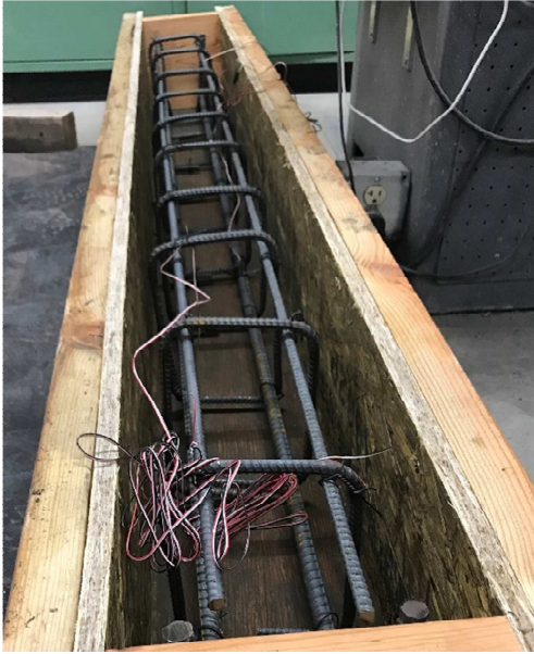
Figure 3-1: Installation of Steel Strain Gauges and Reinforcement Cage for 1 Control Beam
