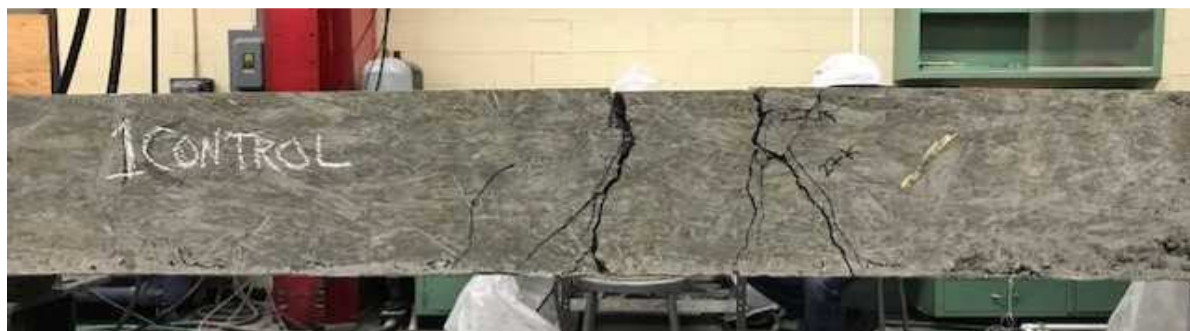
Figure 4-2: Beam 1 CONT Cracked
