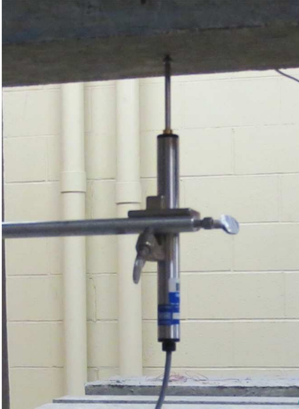
Figure 3-14: LVDT Installed at the Bottom of Beam Mid-span
