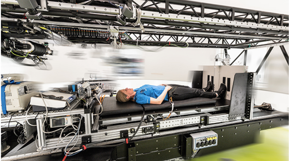
Figure 5.3. The Short Arm Human Centrifuge located at the :envihab research facility. The centrifuge has a radius of 3.8 m and spun at subject-specific rotational speed to generate an acceleration of 1 g at the center of mass and 2 g at the feet to simulate gravity for the iAG and cAG study groups. Image source: DLR (German Aerospace Center), Cologne, Germany.
