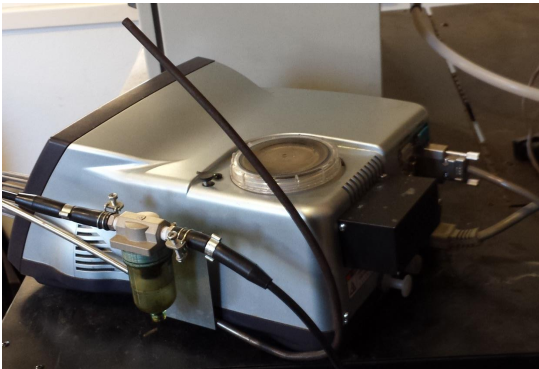
Figure 17: Horiba emissions analyzer.
