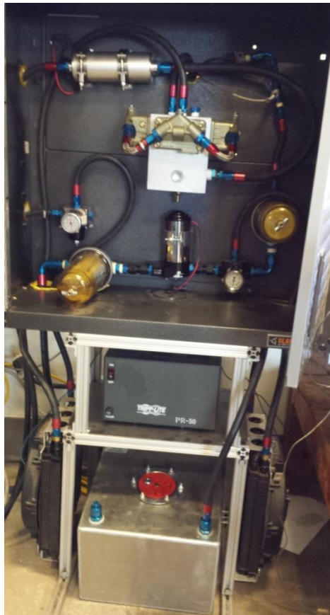
Figure 15: Starter system for SuperFlow.
