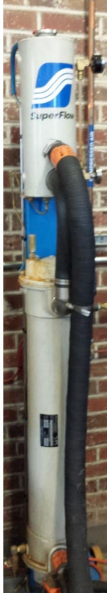
Figure 18: SuperFlow cooling tower for engines.
