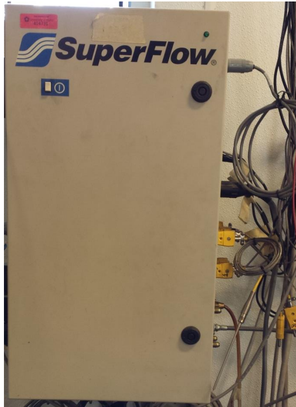
Figure 14: SuperFlow data acquisition box.
