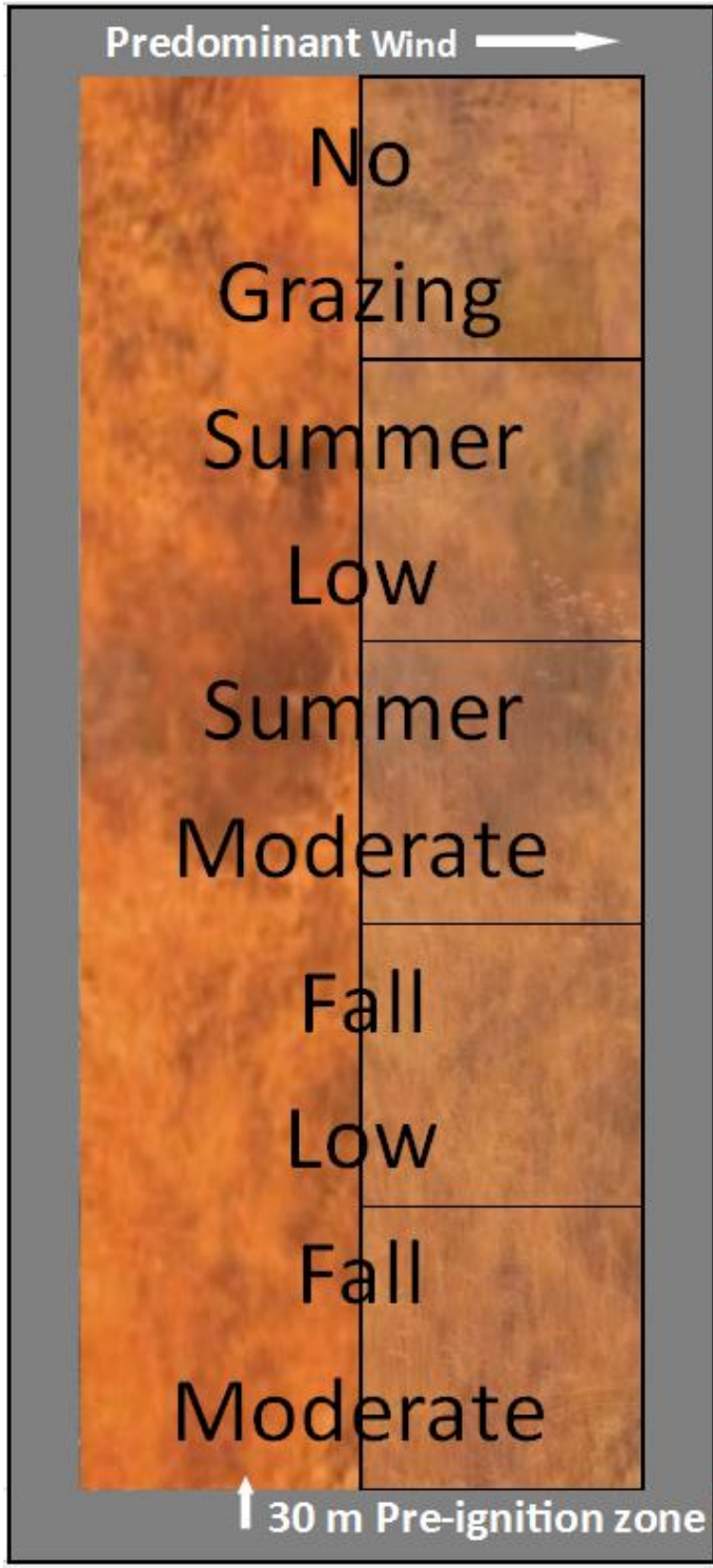
Figure 1 Study block diagram for study in Reynolds Creek, ID. Five 30 x 30 m plots were randomly given a treatment (no grazing, and combinations of summer and fall seasons and low and moderate utilizations) and a 30 m preignition zone was left ungrazed for two years to create wildfire conditions as the prescribed burn spread into the study area.
