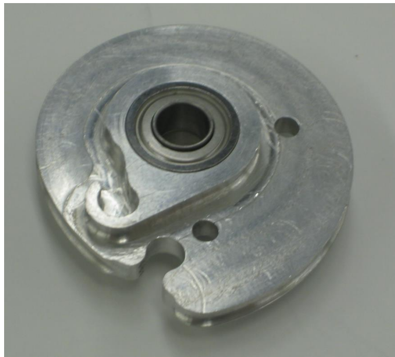
Figure 39. The spring cam. The drive pulley is visible on the top face of the cam. A standoff the same width as the drive pulley exists on the other side of the cam, but it is not visible in this picture.
