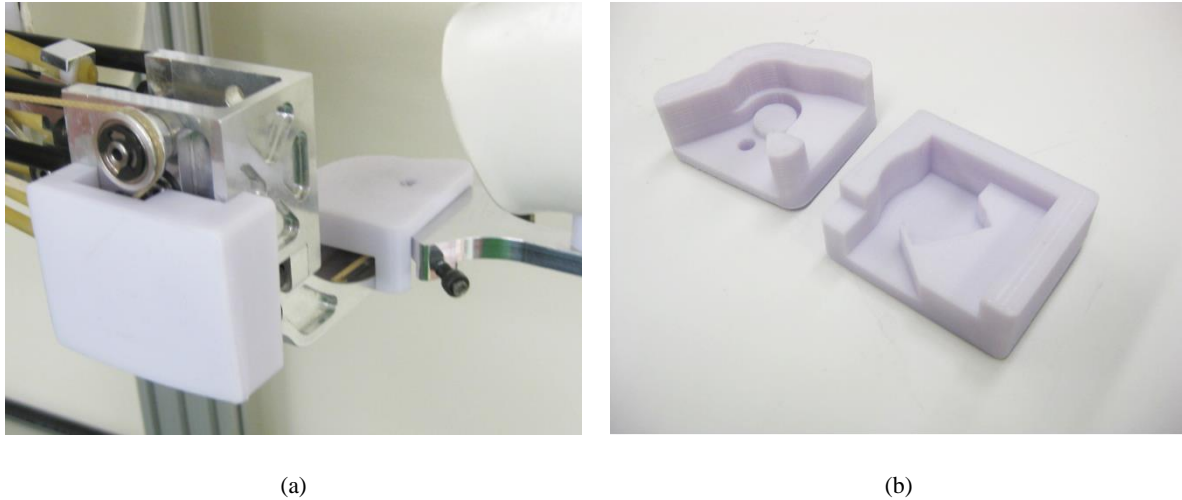
Figure 40. The 3D printed jigs used for adjustment of the antagonistic drive rope of the simultaneous displacement cams. (a) The jigs in use for adjustment. (b) The inside of the jigs. The top left jig constrains the elbow joint to be fully extended. The bottom right jig fixes the simultaneous displacement cams in their correct orientation.
