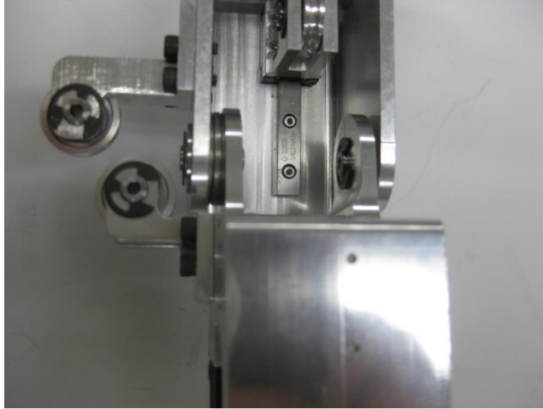
Figure 33. The horizontal joint next to the shoulder with two pins used to provide clearance for the drive rope of the spring cam.
