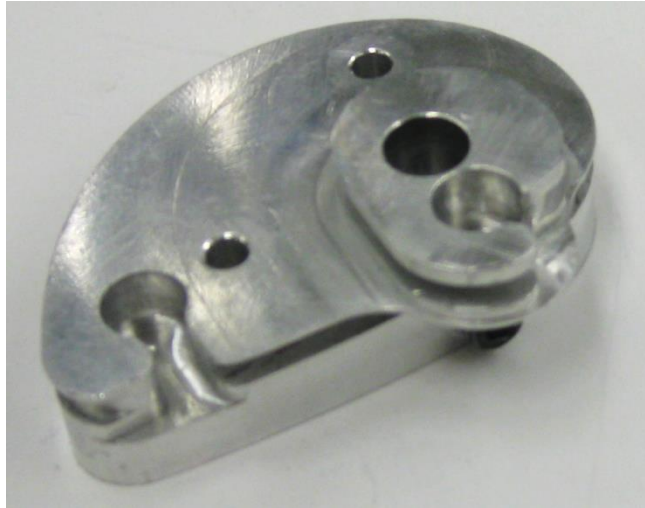
Figure 15. The series cam after machining.
