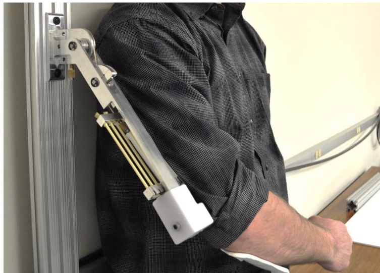
Figure 14. The prototype arm support featuring the series cam mechanism shown supporting a user's arm.
