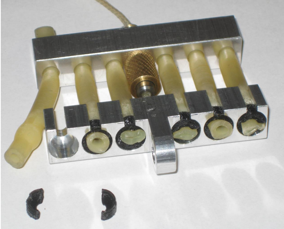
Figure 18. The custom spring built from latex tubing. The tube on the left is shown removed from the end plate to show the hemispherical cup in the endplate. A slight bulge in this tube is visible where the nylon ball sits. Two of the 3D printed wedges are visible on the bottom left.
