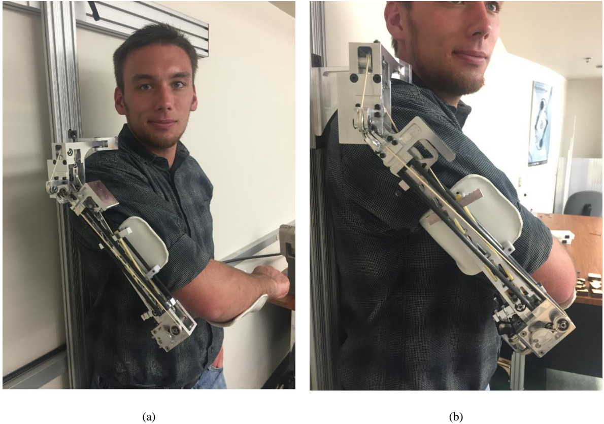
Figure 28. The simultaneous displacement arm support prototype in use. (a) Isometric view of the entire device. (b) Side view of the links next to the upper arm and the shoulder.
