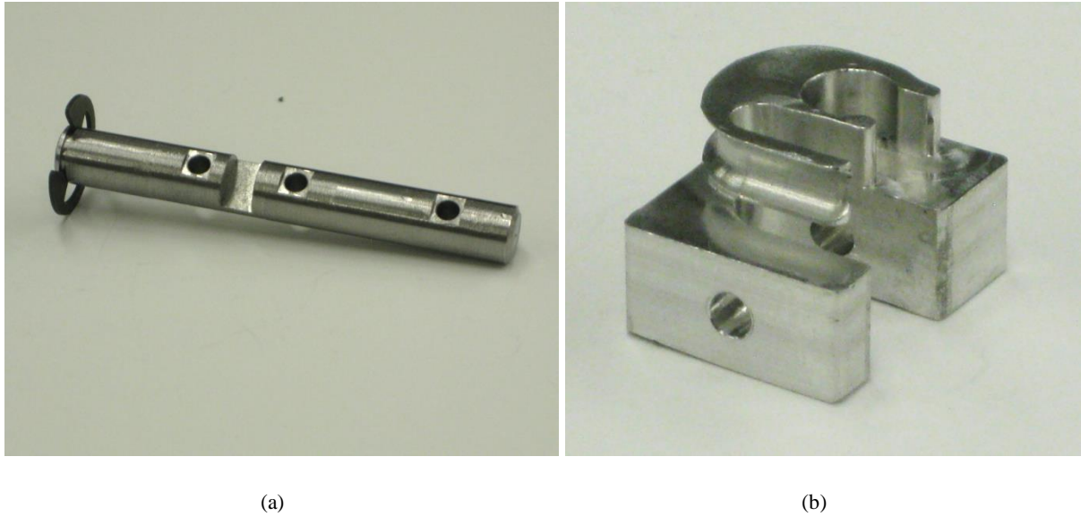
Figure 38. The cam and support shaft machined to allow rope clearance near the rotation axis. (a) The simultaneous displacement cams' support shaft. (b) The cam that actuates the upper arm carriage.
