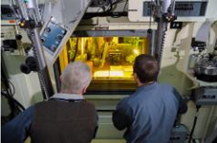
Figure 3.2 Example of HFEF window and performing work using master slave manipulators.
