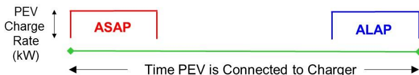
Figure 2.4: All PEV charging is bound by ASAP and ALAP charging. ASAP charging is when the PEV is charged as soon as possible. ALAP charging is when the PEV is charged as late as possible.
