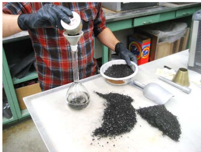
Figure 4.6 Pouring of SSD samples for de-airing
