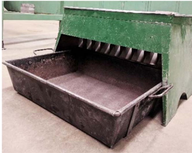
Figure 3.2 Splitter used to reduce samples to test size
