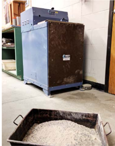
Figure 3.3 Sieve shaker used for sieving
