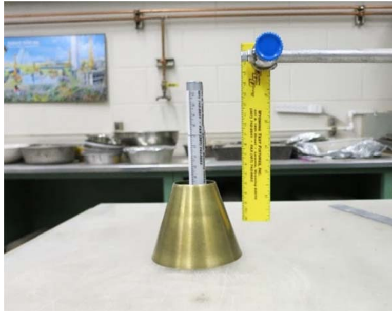
Figure 4.8 Test for tamper drop height
