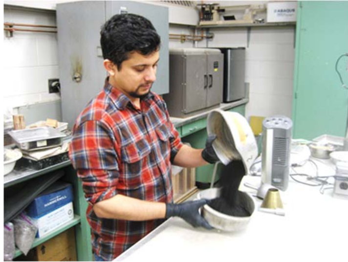
Figure 4.2 Drying of sample using pans
