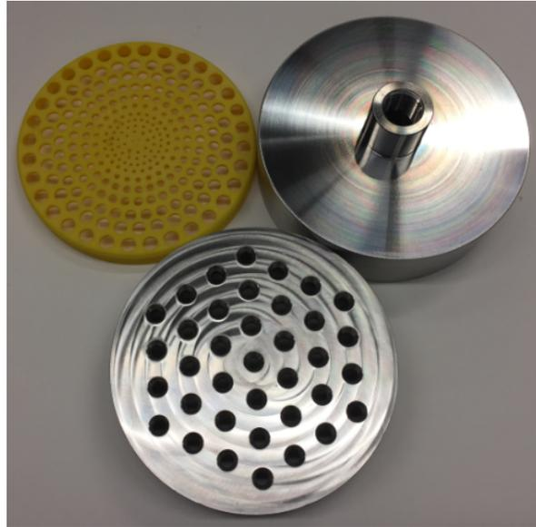
Figure 5.12: Header components - top connector, baffle, and bottom connector
