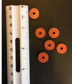
Figure 5.14: Ring gaskets used to create a tight seal around the test section tubes
