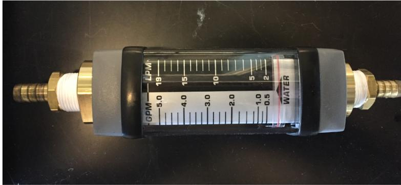
Figure 5.11: Variable area flowmeter for water
