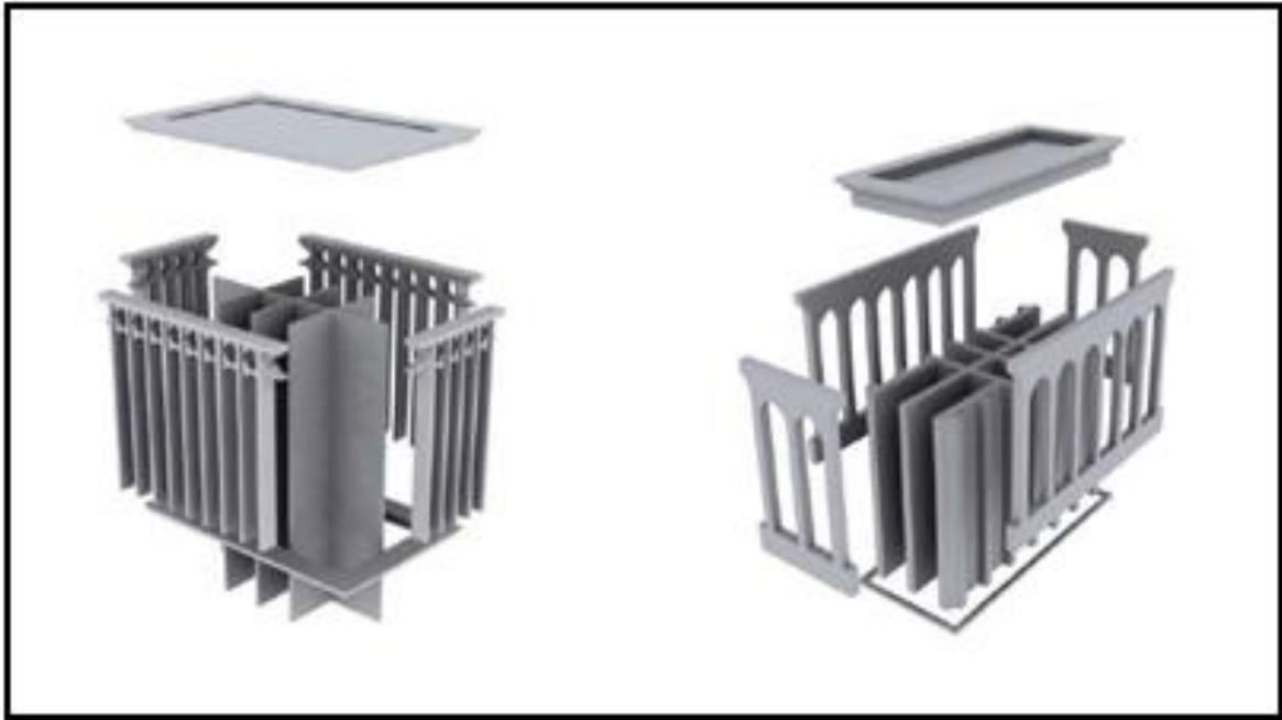
Figure 3-10: 3D Model of a Wind Catcher with Equal Canals [55] (Left), 3D Model of a Wind Catcher with Different Canals [55] (Right)
