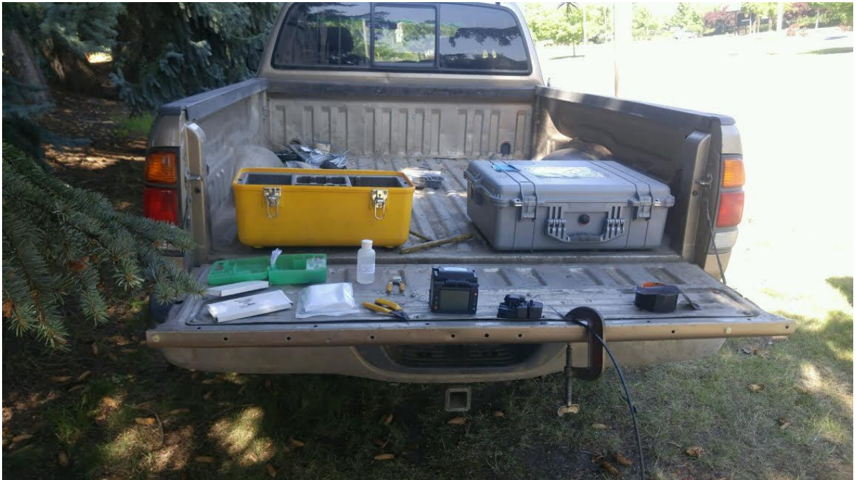
Figure 4.4. Photograph of equipment needed for splicing the fiber-optic cable.
