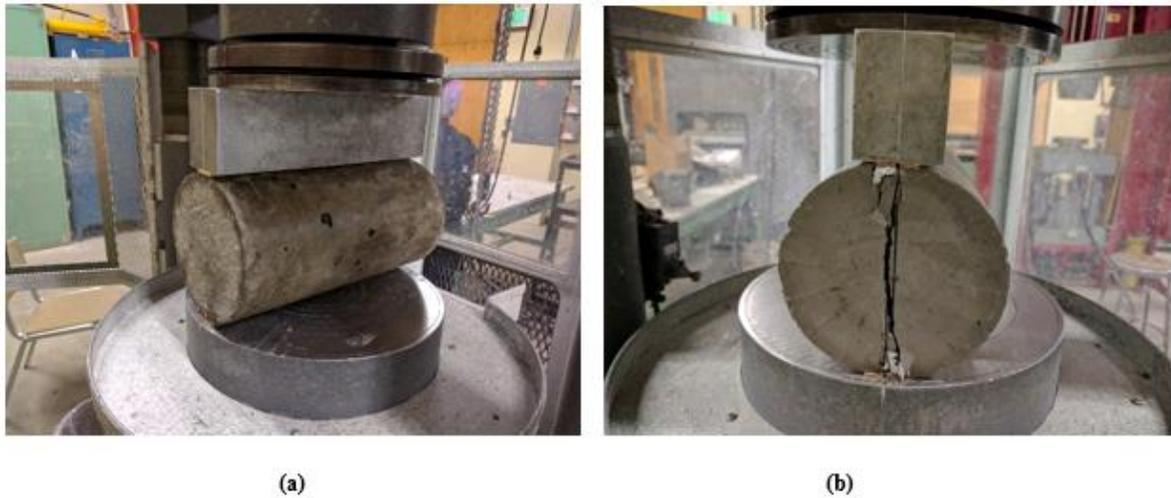
Figure 4.8: (a) Splitting tensile strength test set-up and (b) Typical failure mode of a concrete cylinder under tension.
