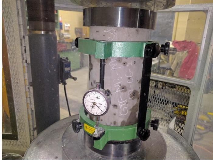
**Figure 4.7: Modulus of elasticity test set-up**
