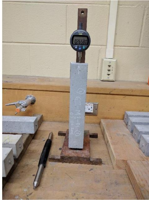
**Figure 4.9: Unrestrained shrinkage test set-up and a concrete prism being tested**
