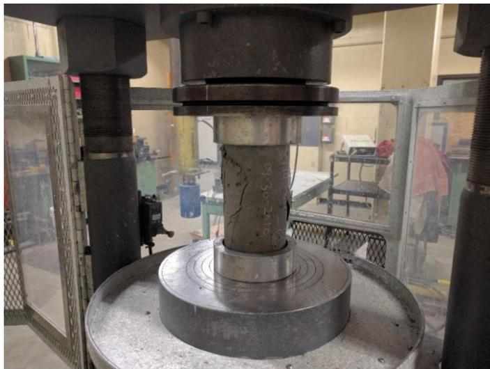
Figure 4.6: Compressive strength test set-up and a typical failure mode of a concrete cylinder under axial compression
