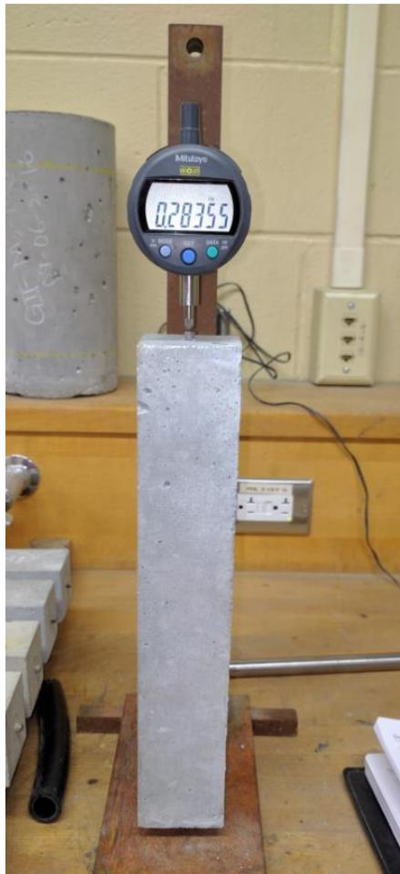
Figure 7.5: Experimental determination of drying shrinkage based on length change
