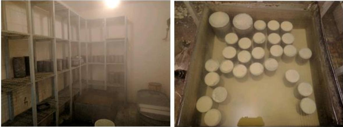
Figure 4.3: Concrete being cured in the curing room and in water tank
