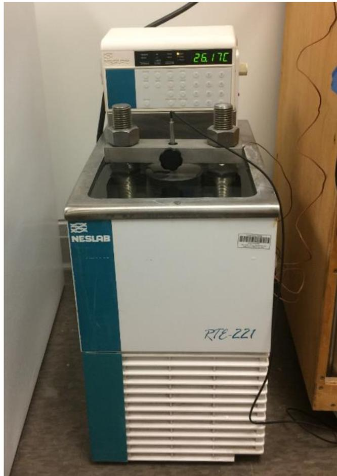
Figure 7.4: Photo showing the temperature-controlled water bath used for CTE testing (WSU).
