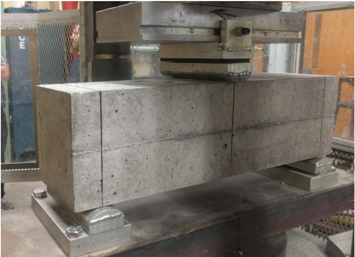
Figure 7.3: Modulus of rupture testing experimental setup
