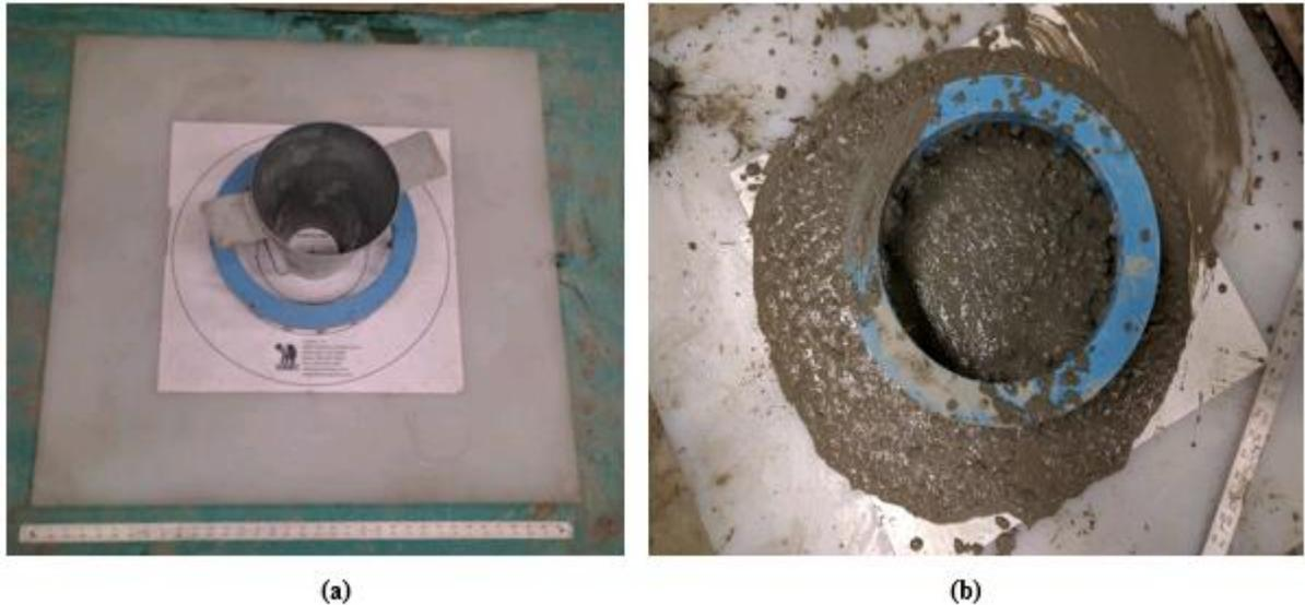
Figure 4.5: (a) J-Ring test setup (b) Typical concrete spread using the J-Ring test
