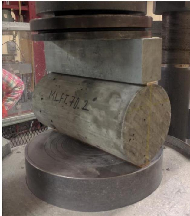
**Figure 7.2: Indirect split tensile strength experimental setup**
