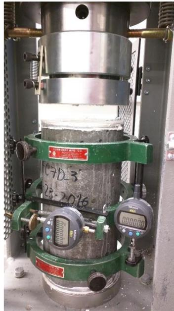
Figure 7.1: Compressometer setup for modulus of elasticity and Poisson's ratio testing
