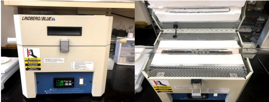
Figure 2.5: Lindberg/Blue tube furnace setup for solution heat treatment (SHT) of 5xxx alloys.
