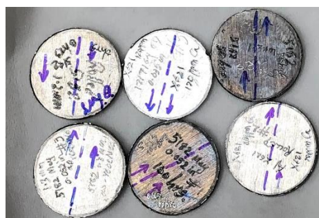
Figure 2.2: Rolled Al working electrode samples.
