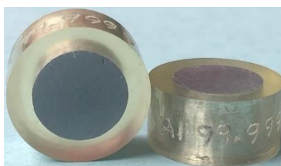
Figure 2.1: Pure Al (99.999%) working electrode sample.
