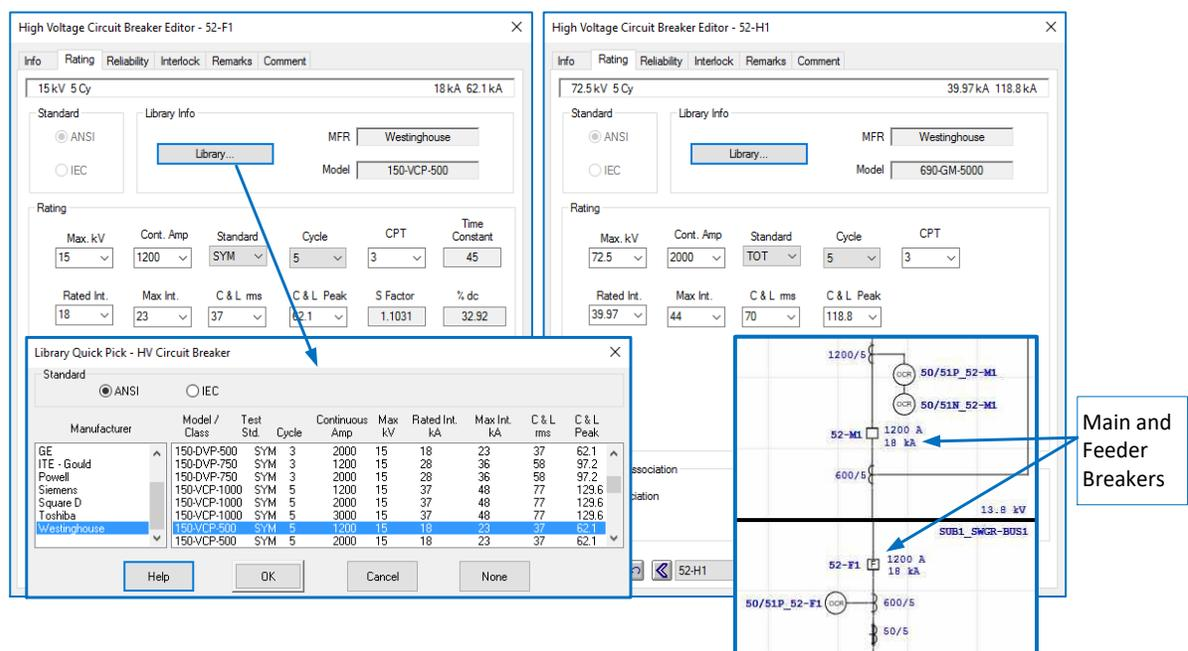
Figure 4.8 – Single-Line View and Parameters for Circuit Breaker Model
