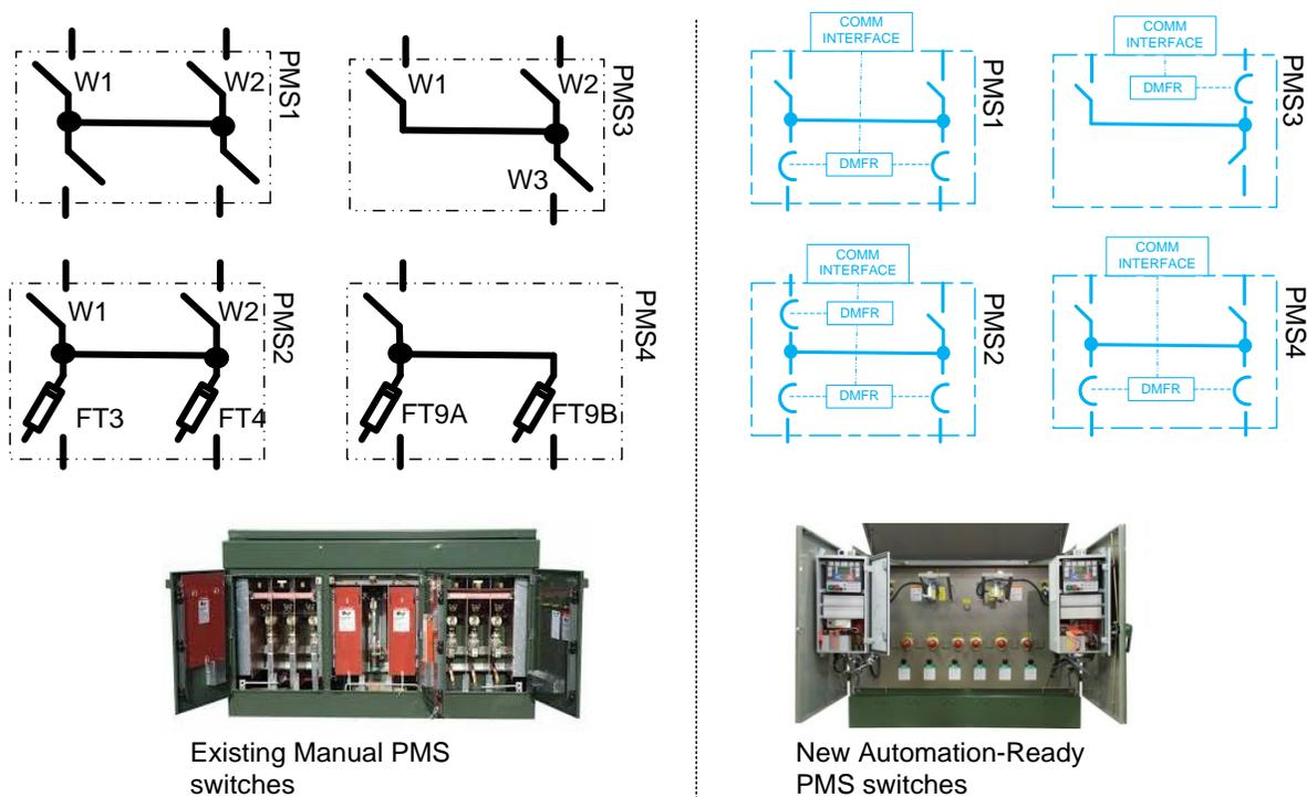
Figure 4.3 – Comparison between Existing and Upgraded PMSs
