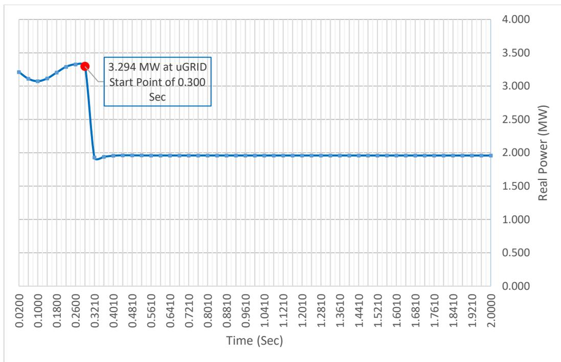
Figure 5.11 – Generator Real Power Output when uGRID1 is formed under Minimum Loading Conditions
