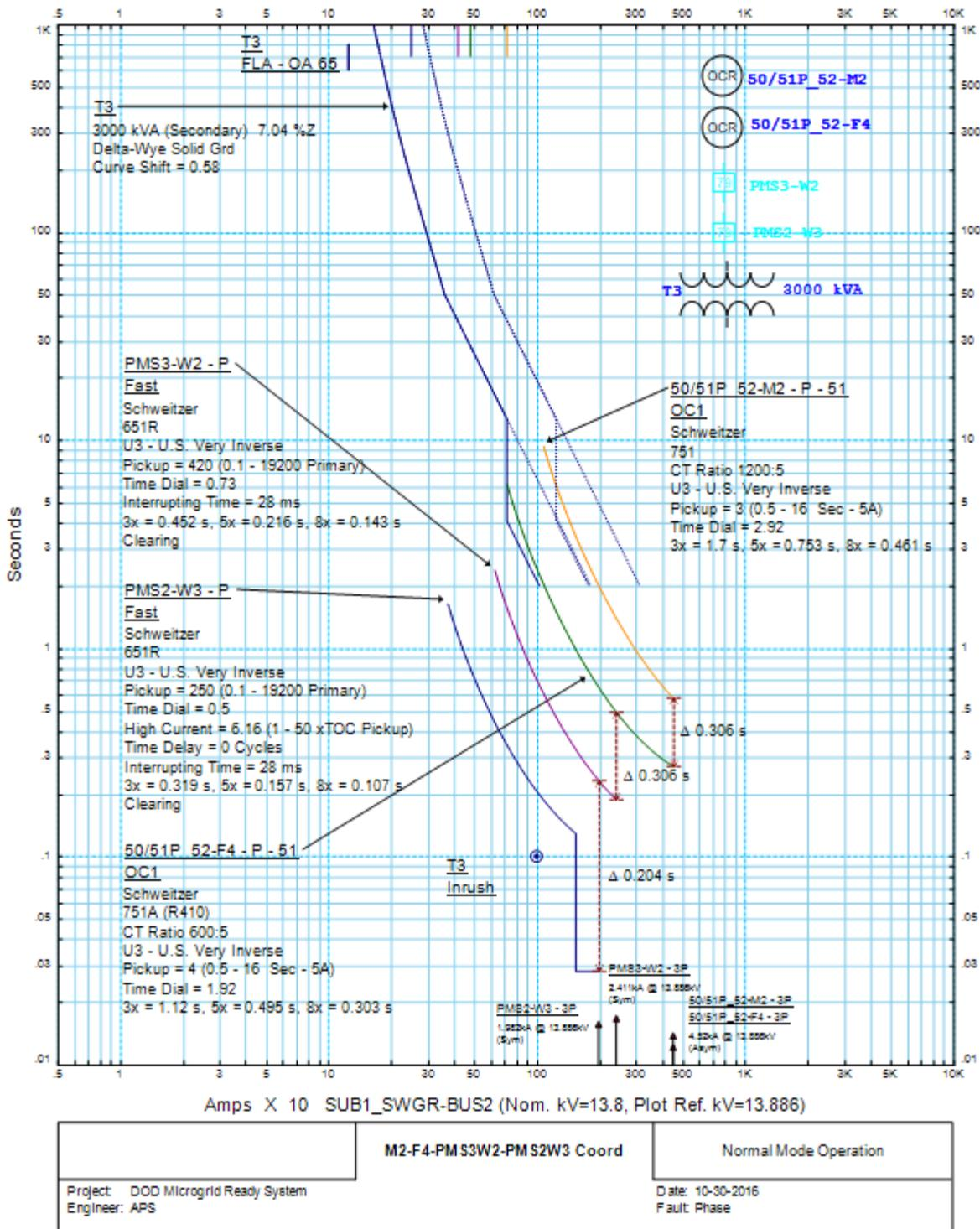
Figure 5.5 – An Example Phase TOC Coordination between PMS-W2 VFI Relay, PMS-W3 VFI 52-F4 Relay, and 52-M2 Relay for Microgrid-Ready System under Normal Mode
