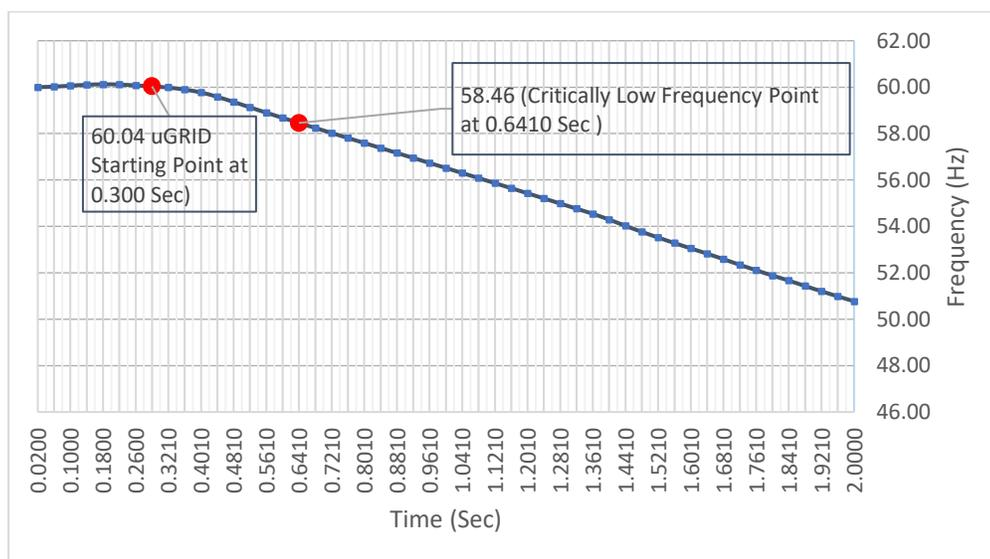
Figure 5.8 –Frequency Response when uGRID1 is formed under Maximum Loading Conditions
