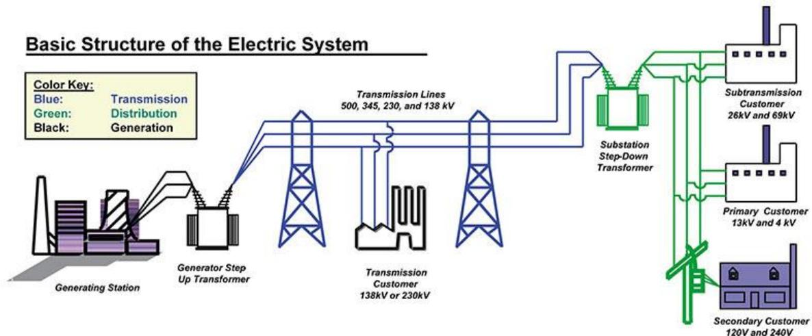
Figure 2.1 – Basis Structure of Electrical Grid System [9]
