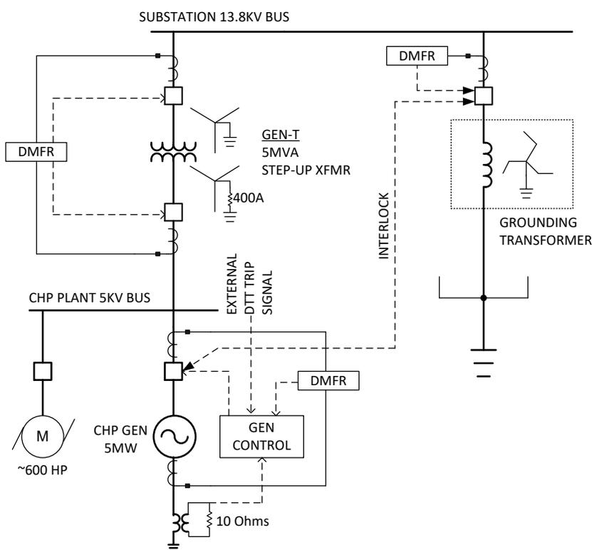
Figure 5.16 – An Example Single-Line Diagram of Grounding Transformer Application to Representative Microgrid-Ready System
