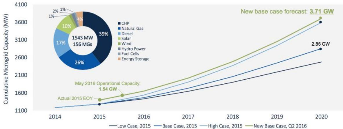
Figure 2.3 – Operational Microgrids in the US as of Q3 2016 and Projected Growth [14]
