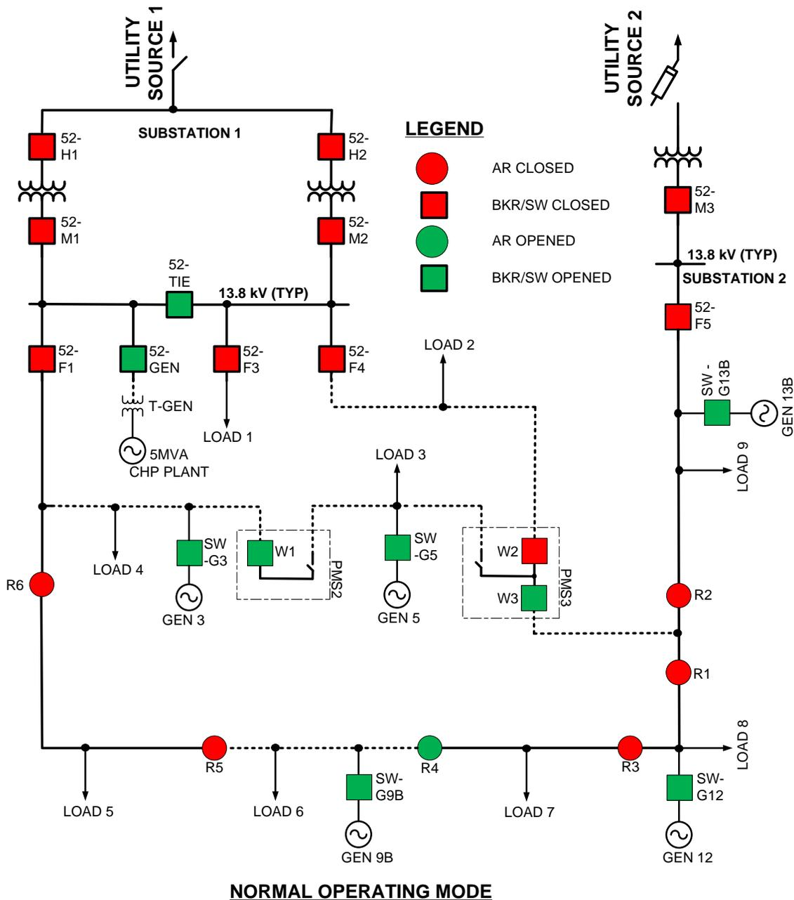
Figure 5.1 – Simplified Normal Mode Switching Configuration of Representative Microgrid-Ready System
