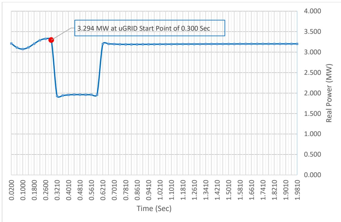
Figure 5.15 – CHP Generator Real Power Profile as uGRID1 forms and Load is added under Minimum Loading Conditions
