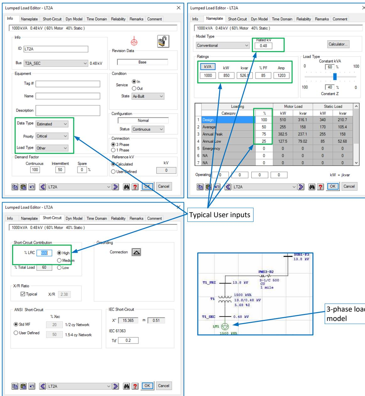
Figure 4.18 – Single-Line View and Parameter Dialogs for Typical Lumped Load Model
