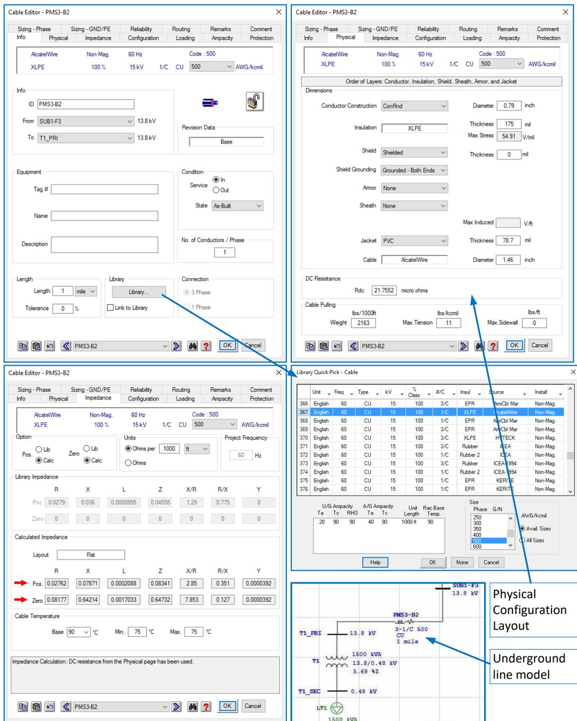
Figure 4.11 – Single-Line View and Parameter Dialogs for Underground Line Model
