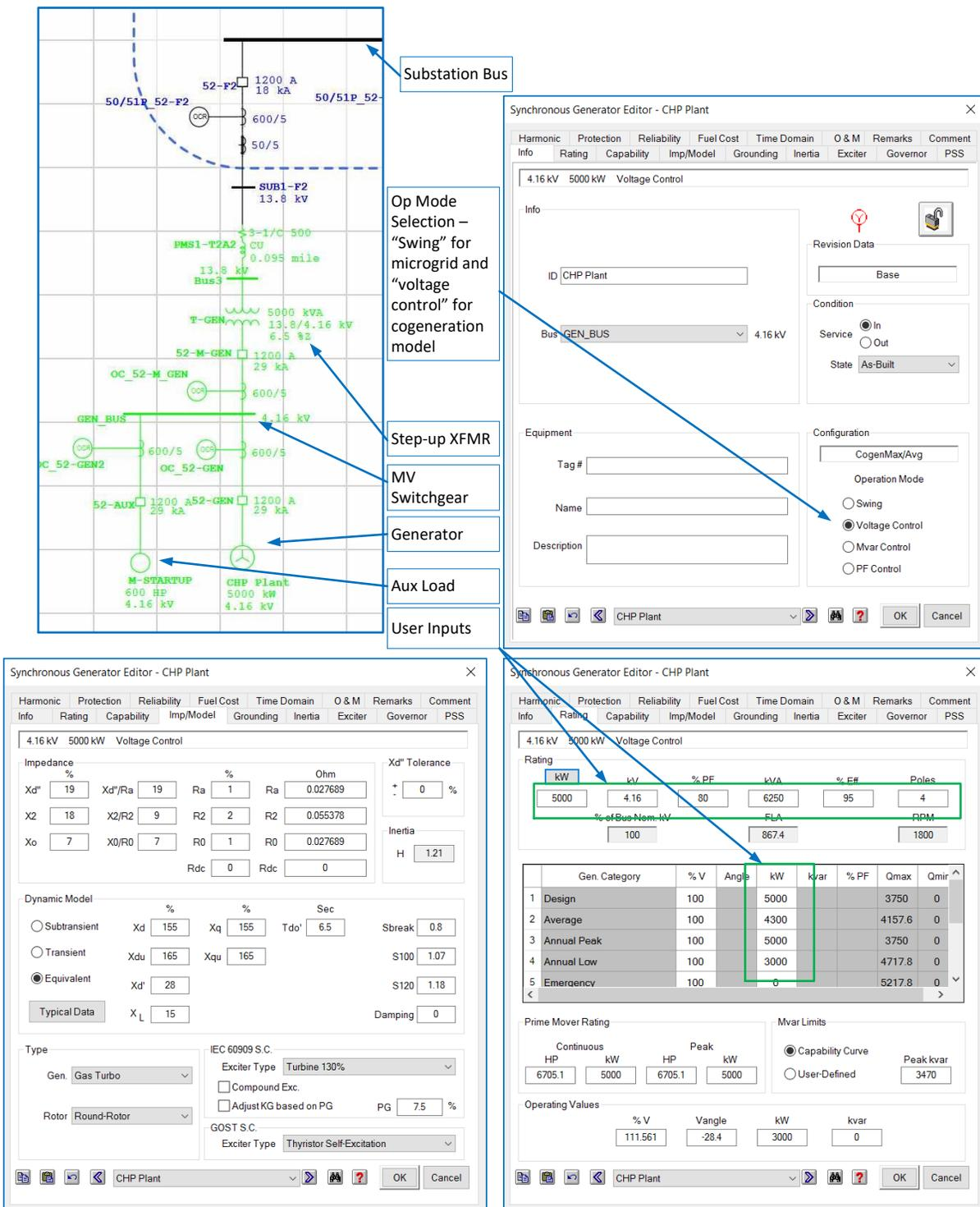
Figure 4.16 – Single-Line View and Parameter Dialogs for CHP Generator Model
