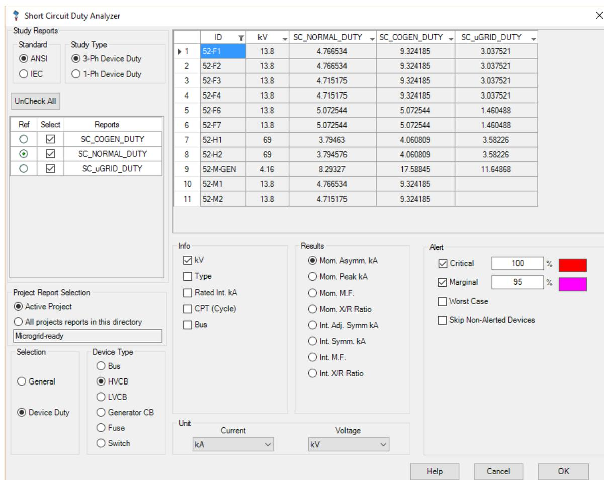
Figure 5.3 – ANSI Device Duty Fault Comparison for Circuit Breakers for Different Operating Modes
