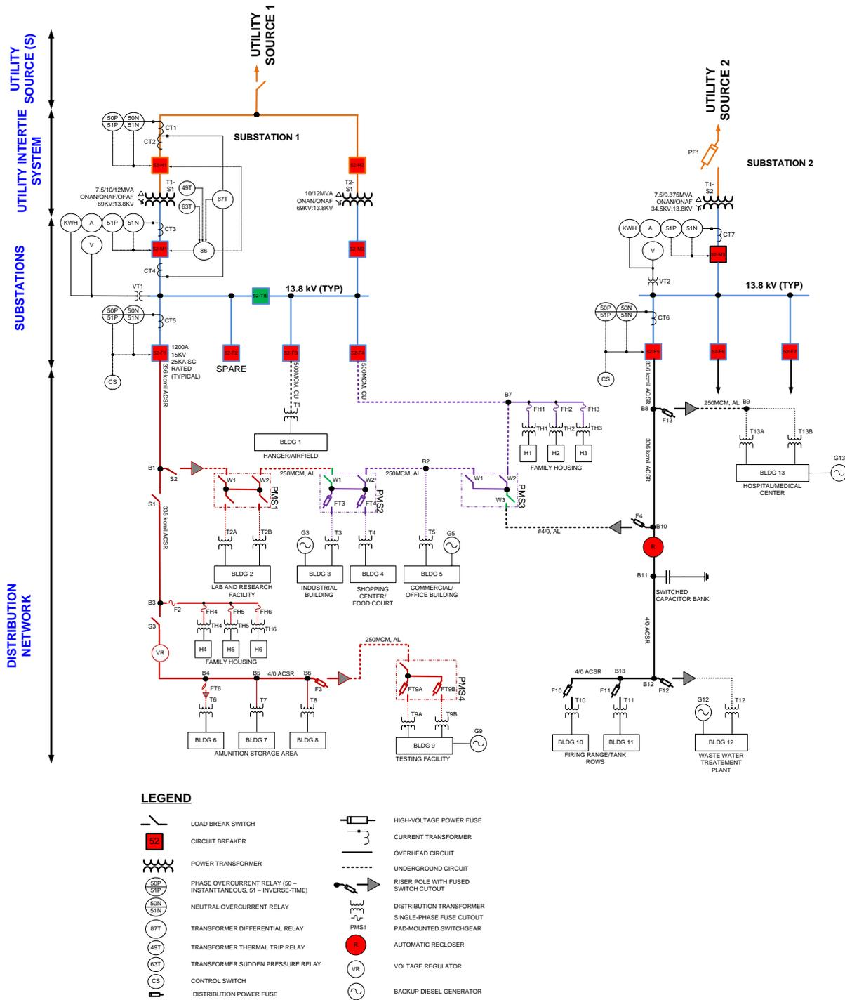
Figure 3.2 – Representative Single Line of Typical DOD Electrical Systems
