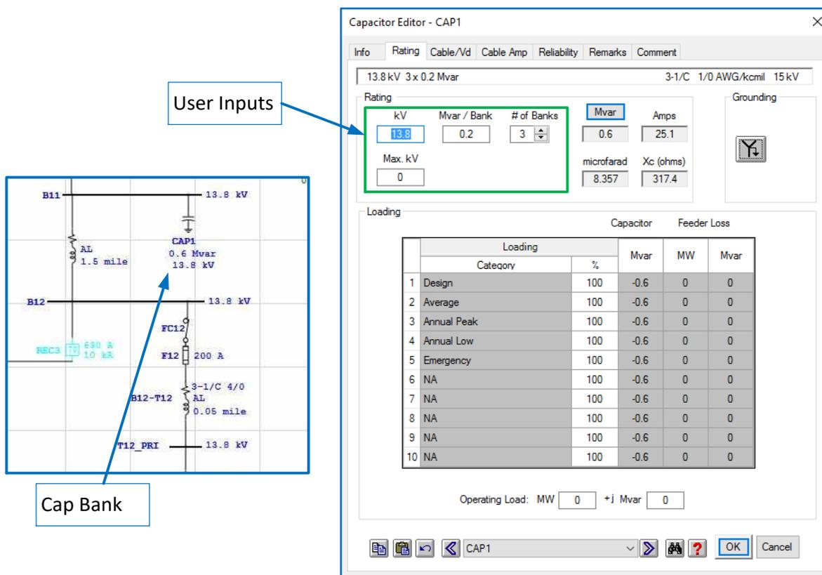
Figure 4.15 – Single-Line View and Parameter Dialogs for Typical Capacitor Bank Model
