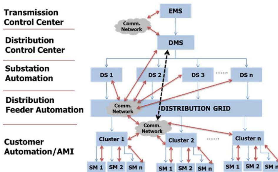
Figure 6.2 – Typical Four-Tier Distribution Communication System Architecture [41]
