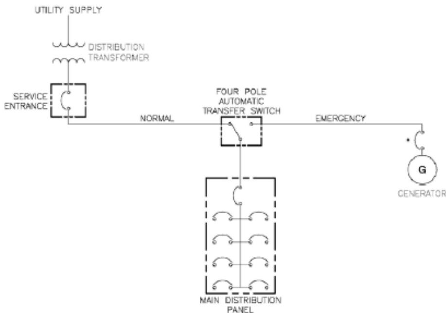
Figure 1.4 – Single Engine Generator Configuration for Whole Building Supply [4]
