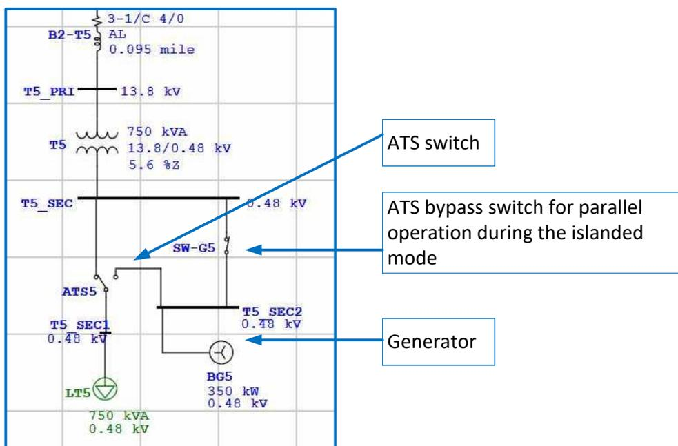
Figure 4.17 – Single-Line View of a Backup Generator Model
