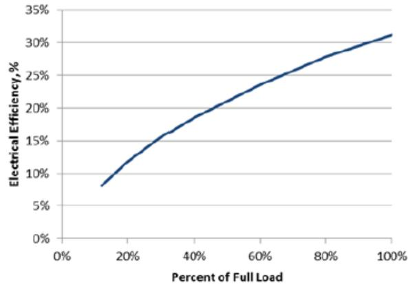
Figure 5.2 – Effect of Partial Load Operation on Efficiency of Typical Gas Turbine Generator [32].
