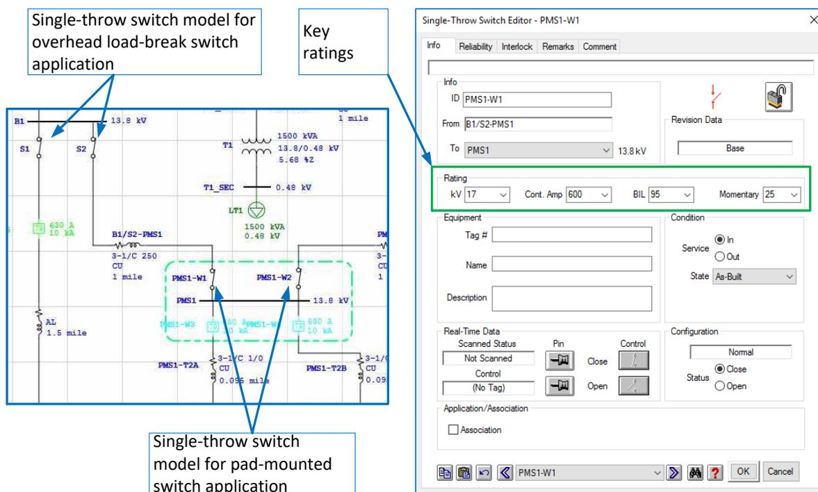
Figure 4.12 – Single-Line View and Parameter Dialogs for Single-Throw Switch Model
