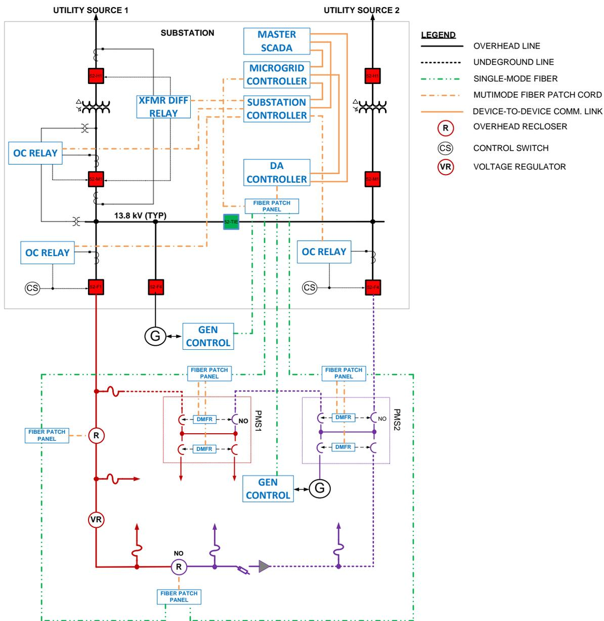
Figure 3.7 – Simplified Conceptual Microgrid Ready System Single Line
