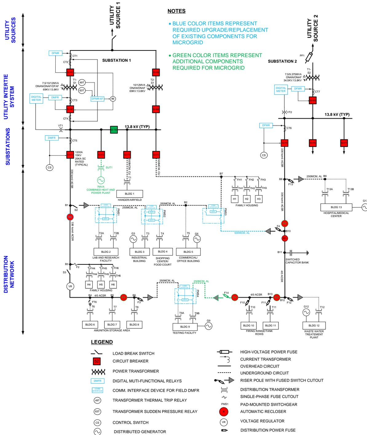
Figure 3.8 – Representative Microgrid-Ready System Single Line Diagram
