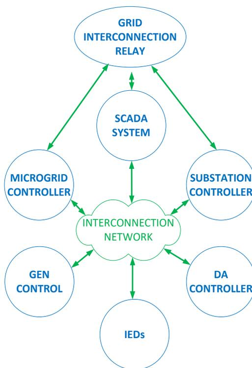
Figure 6.1 – Conceptual Communications Network for the DOD Representative Microgrid System
