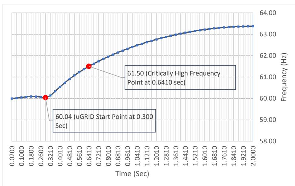
Figure 5.10 – System Frequency Response when uGRID1 is formed under Minimum Loading Conditions
