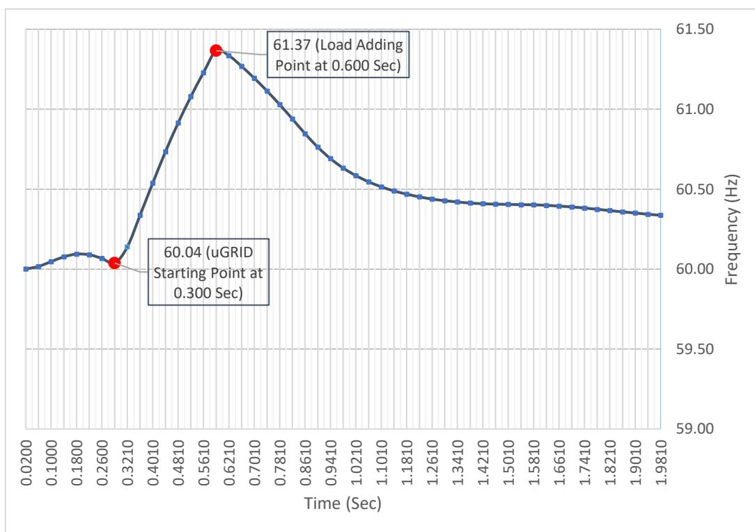
Figure 5.14 – Frequency Response as uGRID1 forms and Load is added under Minimum Loading Conditions
