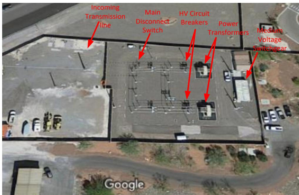
Figure 3.3 – Substation Layout of One of the Air Force Bases [26]
