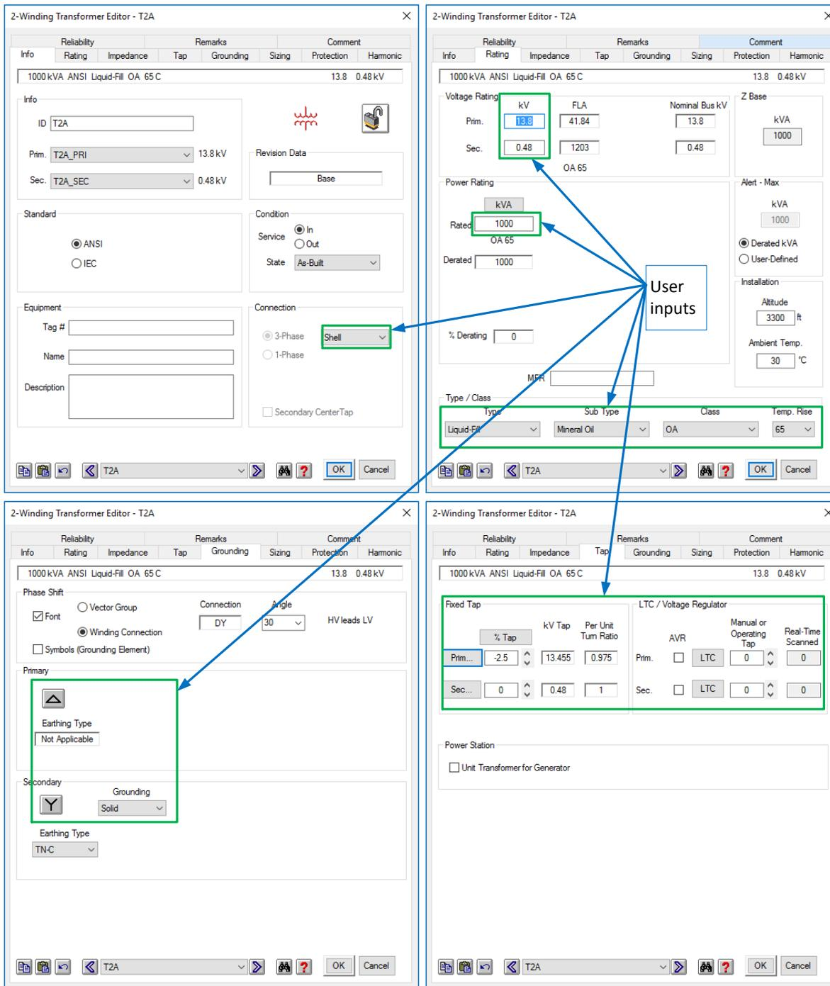
Figure 4.14 – Single-Line View and Parameter Dialogs for Typical Service Transformer Model
