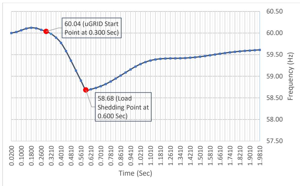
Figure 5.12 – Frequency Response as uGRID1 forms and Load is shed under Maximum Loading Conditions
