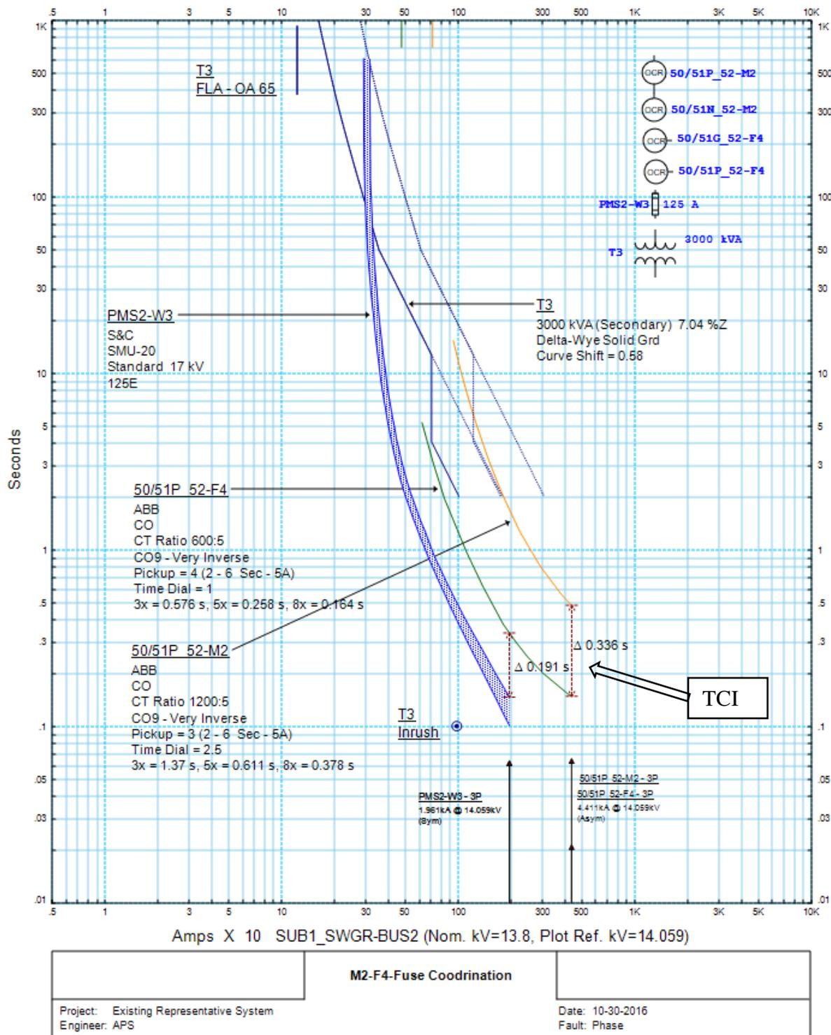
Figure 5.4 – An Example Phase TOC Coordination between PMS2-W3 Fuse, 52-F4 Relay, and 52-M2 Relay for Existing Representative System
