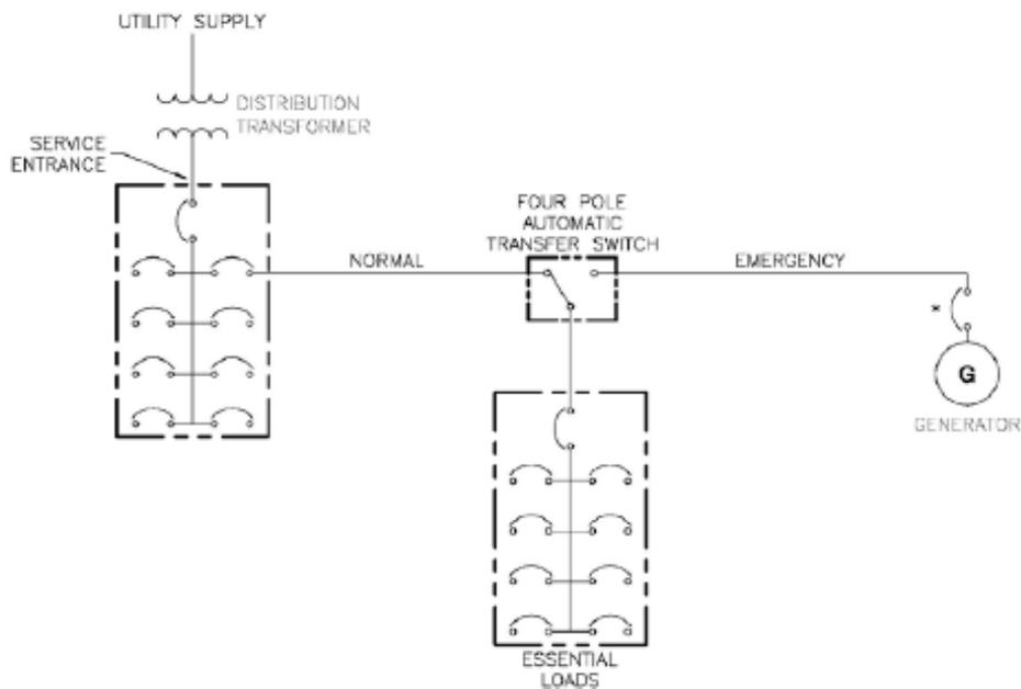
Figure 1.3 – Single Engine Generator Supply to Essential Loads [4]
