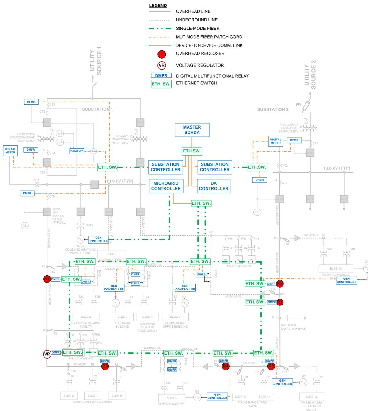
Figure 6.5 – Conceptual Communication Architecture for the Representative Microgrid-Ready System.
