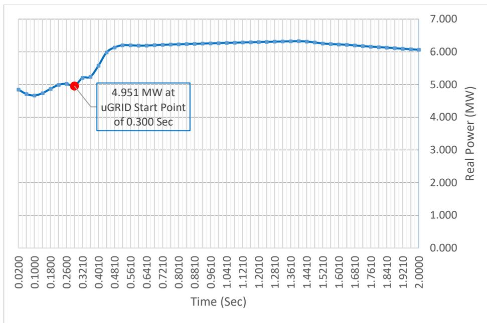
Figure 5.9 – CHP Generator Real Power Output when uGRID1 is formed under Maximum Loading Conditions
