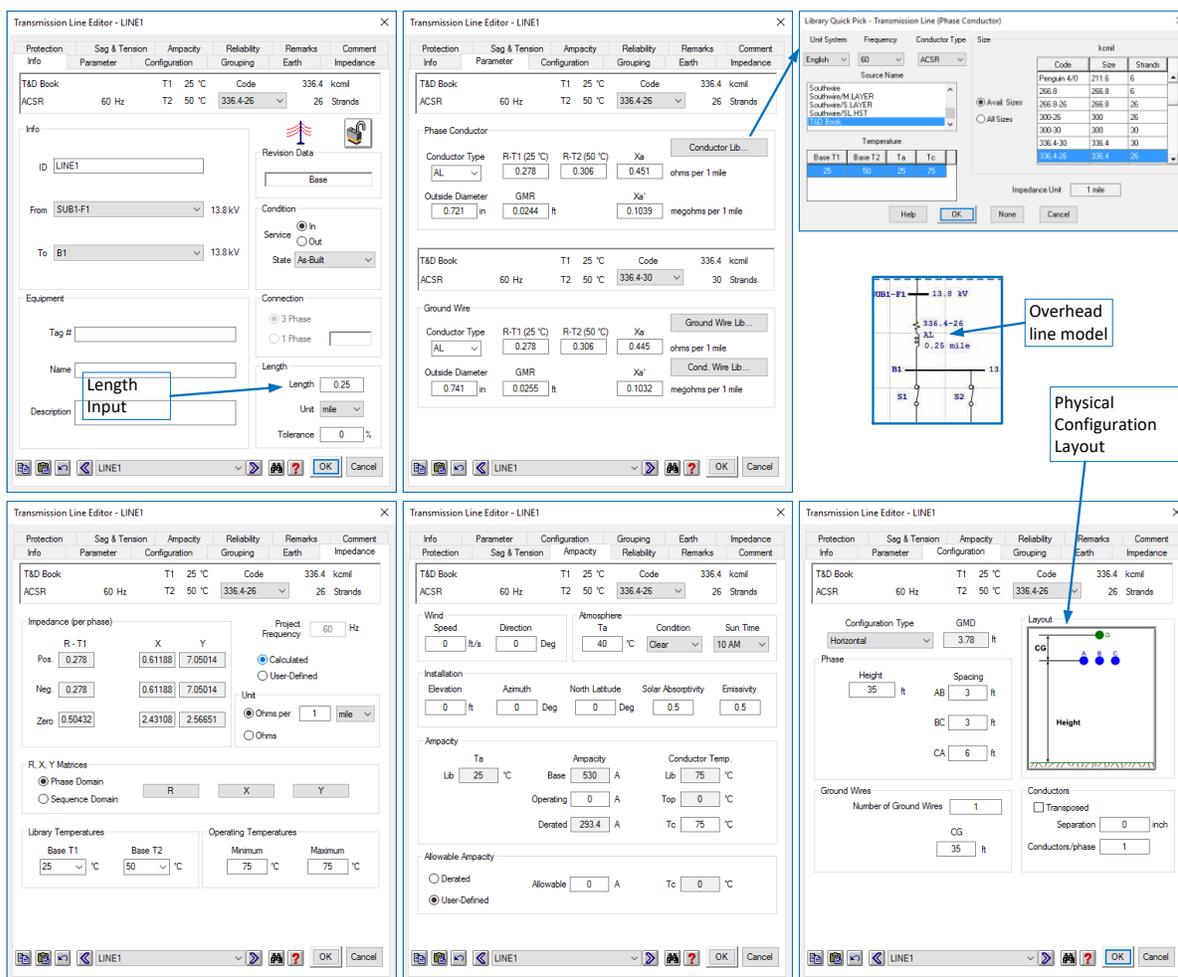
Figure 4.10 – Single-Line View and Parameter Dialogs for Overhead Line Model
