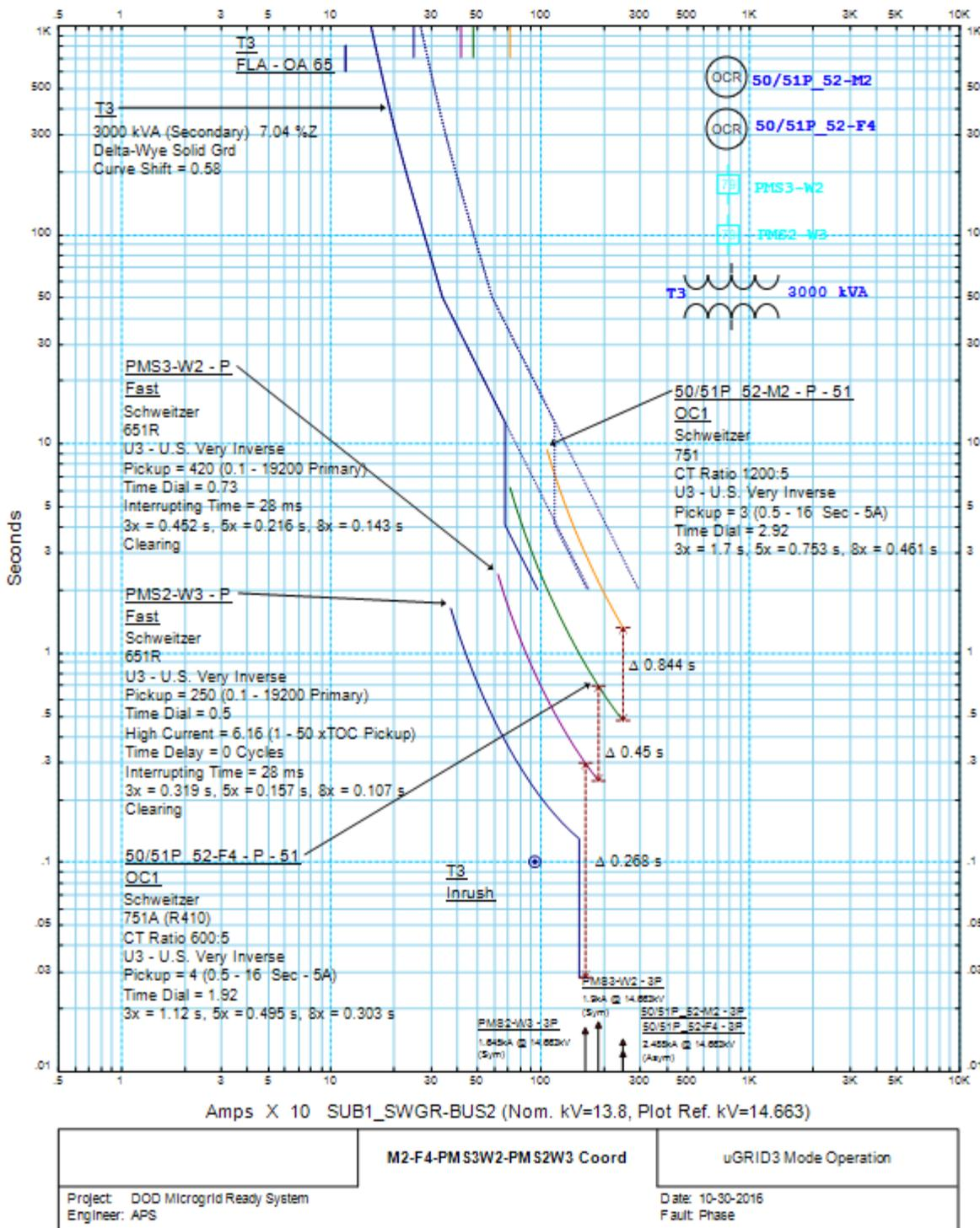
Figure 5.7 – An Example Phase TOC Coordination between PMS-W2 VFI Relay, PMS-W3 VFI 52-F4 Relay, and 52-M2 Relay for Microgrid-Ready System under uGRID3 Mode
