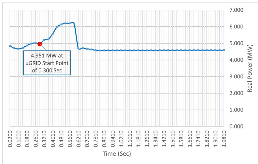
Figure 5.13 – CHP Generator Real Power Profile as uGRID1 forms and Load is shed under Maximum Loading Conditions
