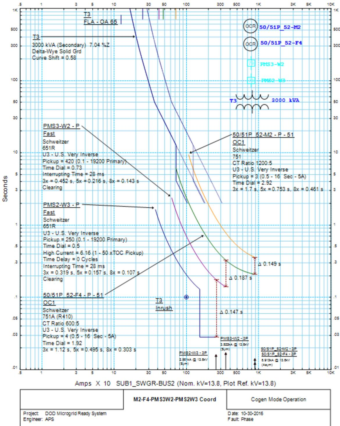
Figure 5.6 – An Example Phase TOC Coordination between PMS-W2 VFI Relay, PMS-W3 VFI 52-F4 Relay, and 52-M2 Relay for Microgrid-Ready System under Cogen Mode
