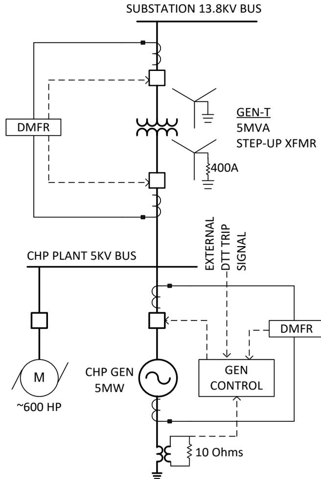
Figure 4.4– Single-Line Configurations of New CHP Generator System
