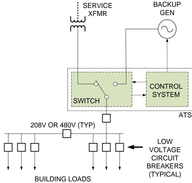
Figure 3.5 – Typical Emergency Backup Generator and ATS Configuration for Critical Load
