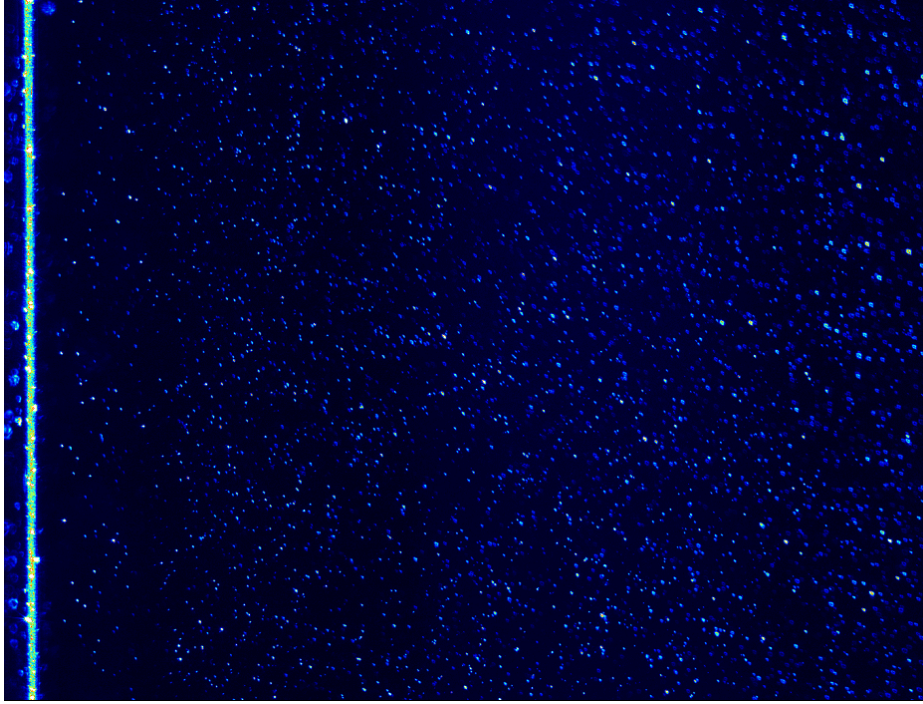
Figure 5.2: An example image frame of particles being moved from the wall boundary (bright strip of light near the left side of the figure).
