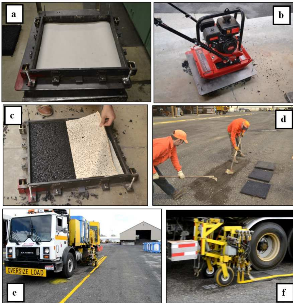
Figure 3.2: (a, b, c) Slab preparation, (d) Slab placement for striping, (e,f) Striping of slabs
