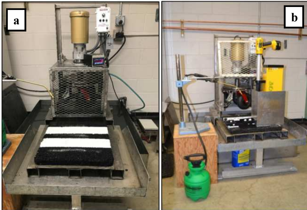
Figure 3.3: (a) TWPD, (b) Taking readings on test slab
