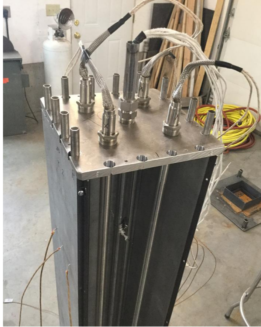
Figure 3.5: Cask with slab S1 taken off showing the insertion heaters and central thermocouple tube
