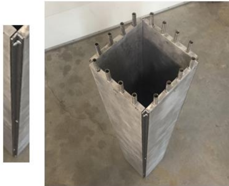
Figure 3.2: Figure showing basic frame of Sakae experimental cask constructed with 0.25-in angle irons
