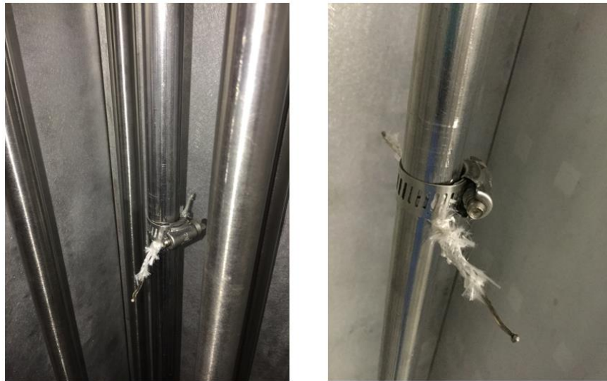
Figure 3.6: Image of internal thermocouple setup
