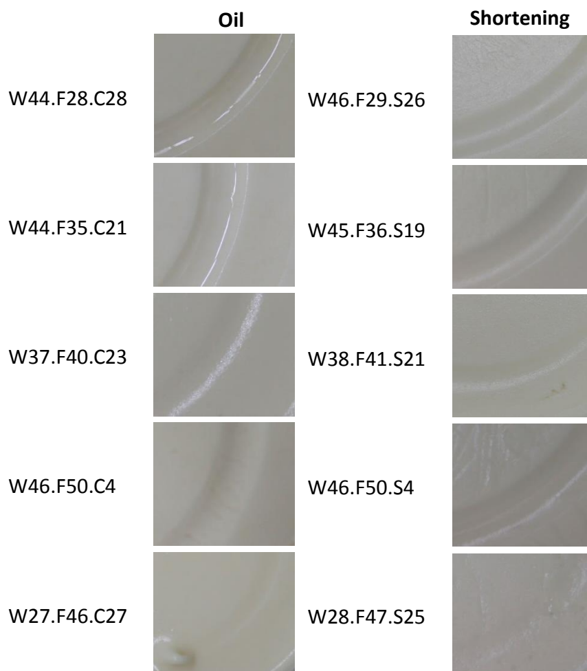
Figure 3.4. Selected images of wear tracks for oil and shortening formulations.
