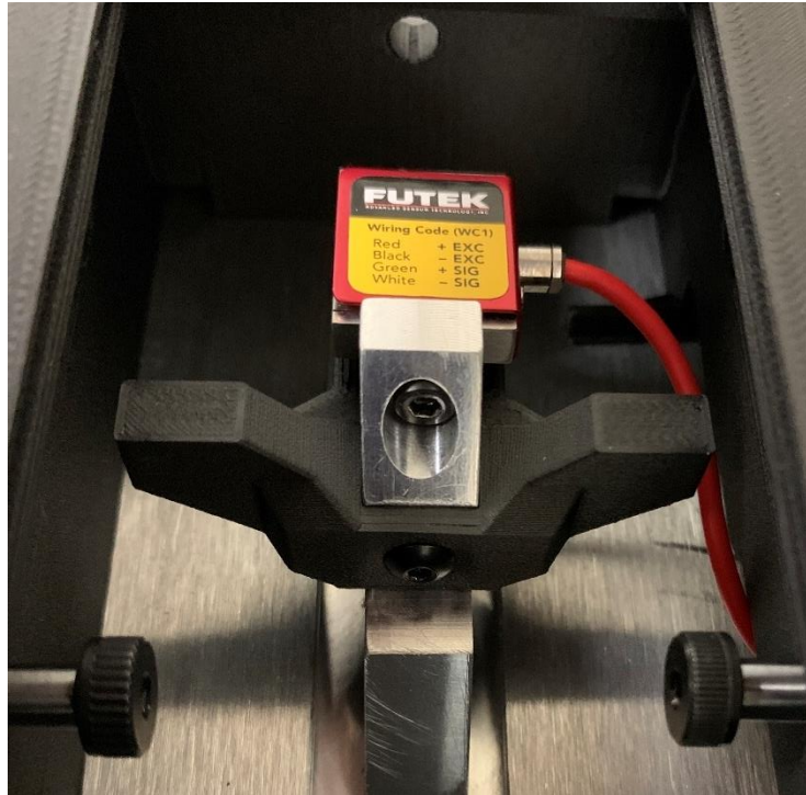
Figure 2.74 Load cell secured to load cell mount with screw.
