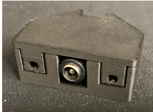
Figure 2.44 Top cover of DC panel mount part added.
