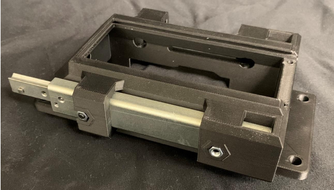
Figure 2.9 Slider moved forward and nut inserted in cutout.
