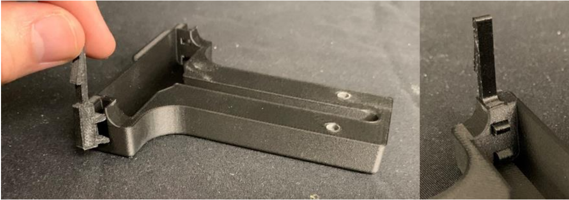
Figure 2.36 (Left) Placement for compliant clip on load cell wire cover. (Right) Fully seated compliant clip.
