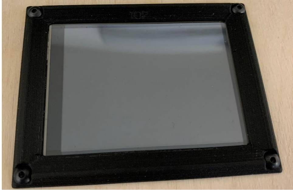
Figure 2.47 Touch screen frame with screws mounted to top cover.
