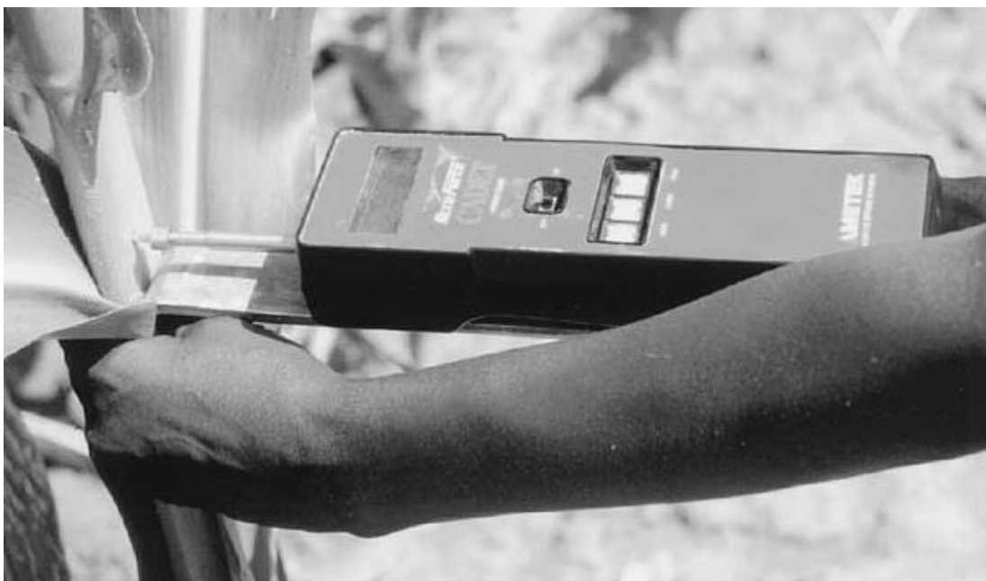
Figure 1.5 [22] Rind puncture resistance device.
