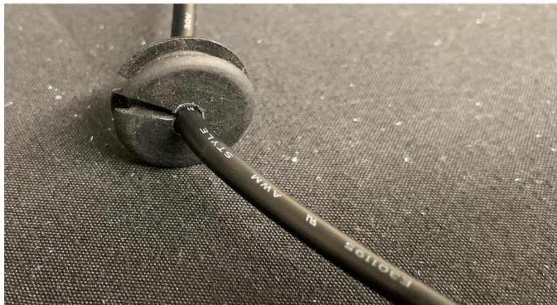
Figure 2.54 Cut grommet placed on USB splitter cable.
