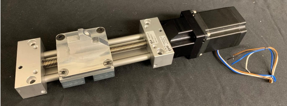
Figure 2.19 Linear system with load cell mount attached.
