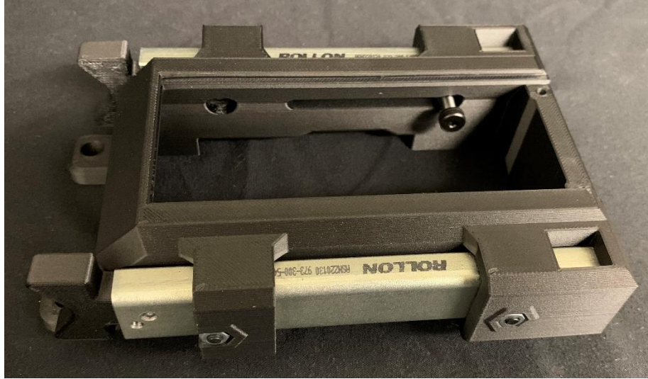
Figure 2.13 Load cell cover with both sliders installed.
