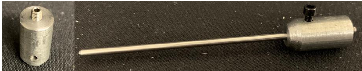
Figure 2.71 Needle chuck being assembled.
