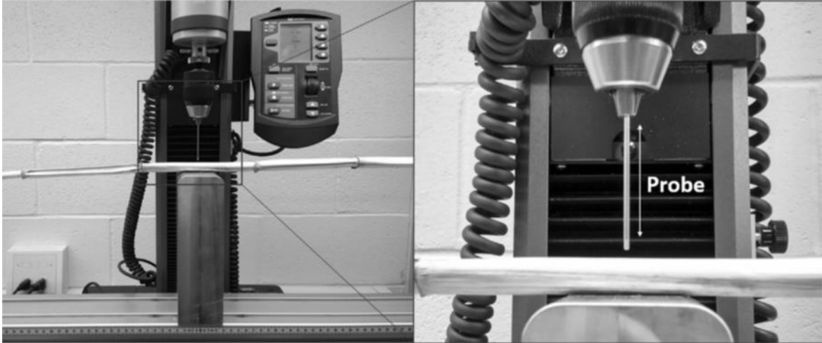
Figure 1.7 [29] Puncture test being run on Instron.
