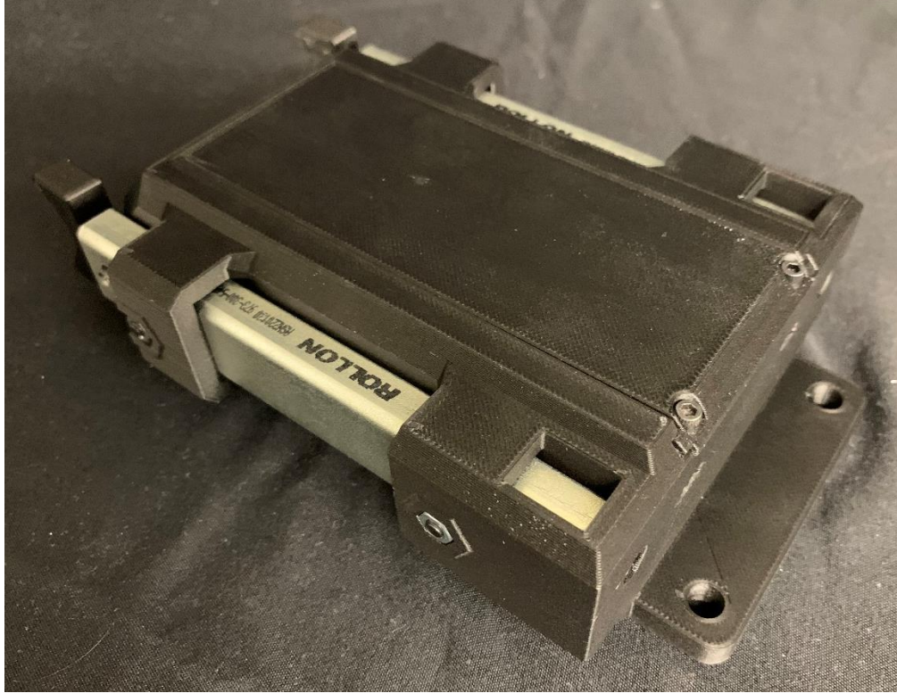
Figure 2.15 Fully assembled load cell cover.
