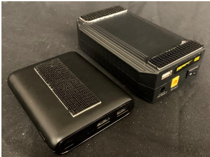
Figure 2.68 Hook and loop tape applied to batteries.
