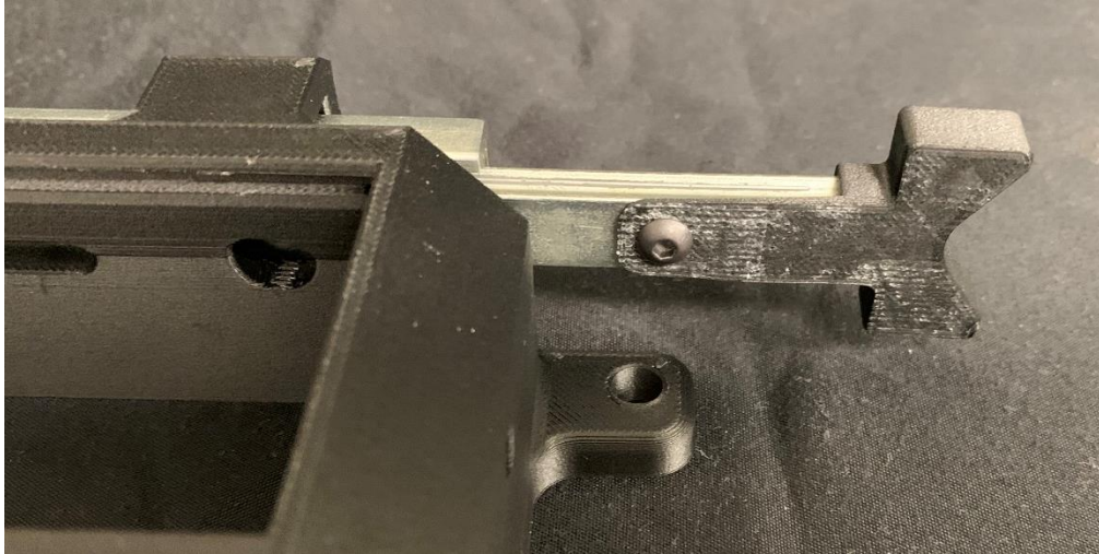
Figure 2.11 Slide pushed forward with holder head attached.
