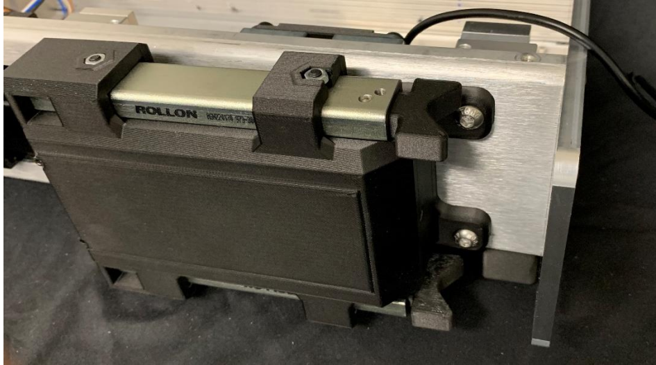
Figure 2.25 Front bolts attaching load cell cover and linear system to case.
