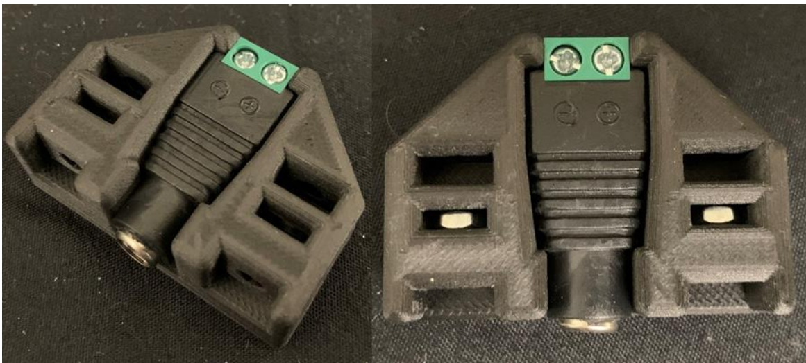
Figure 2.43 DC plug to discreet wire part and nuts set into mount.
