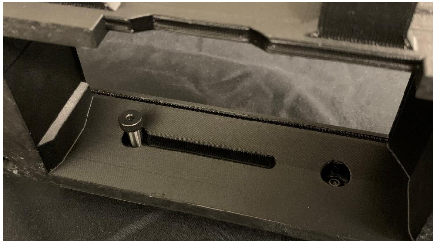
Figure 2.12 Shoulder bolt threaded into interior of slide.
