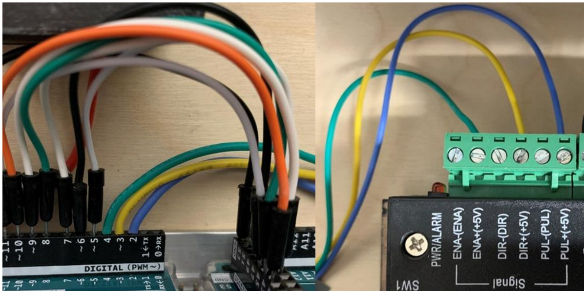
Figure 2.58 Wiring Arduino Uno to motor driver.
