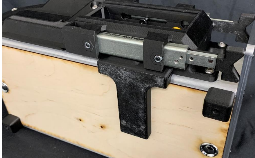
Figure 2.38 Load cell wire cover snapped in place.
