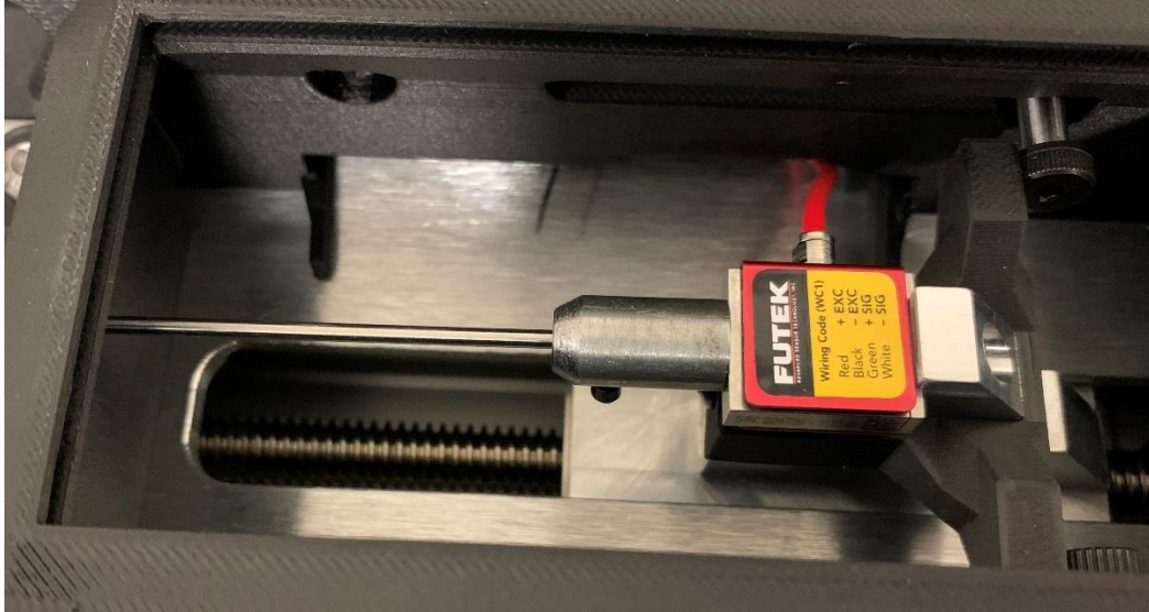
Figure 2.75 Needle chuck threaded onto loadcell.
