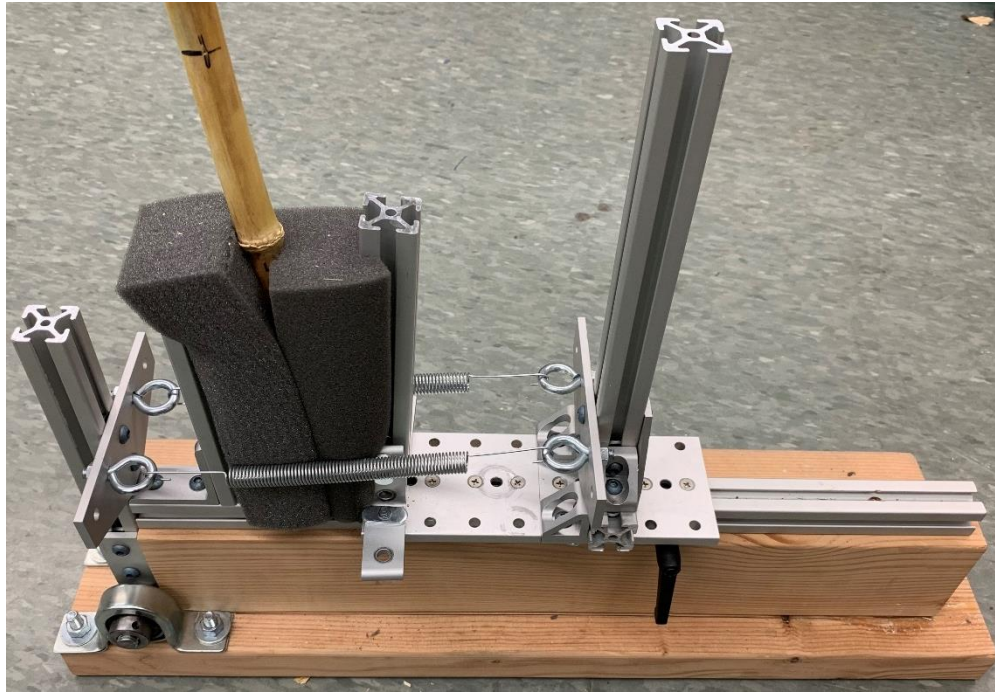
Figure 2.90 Stalk holder for validation tests.
