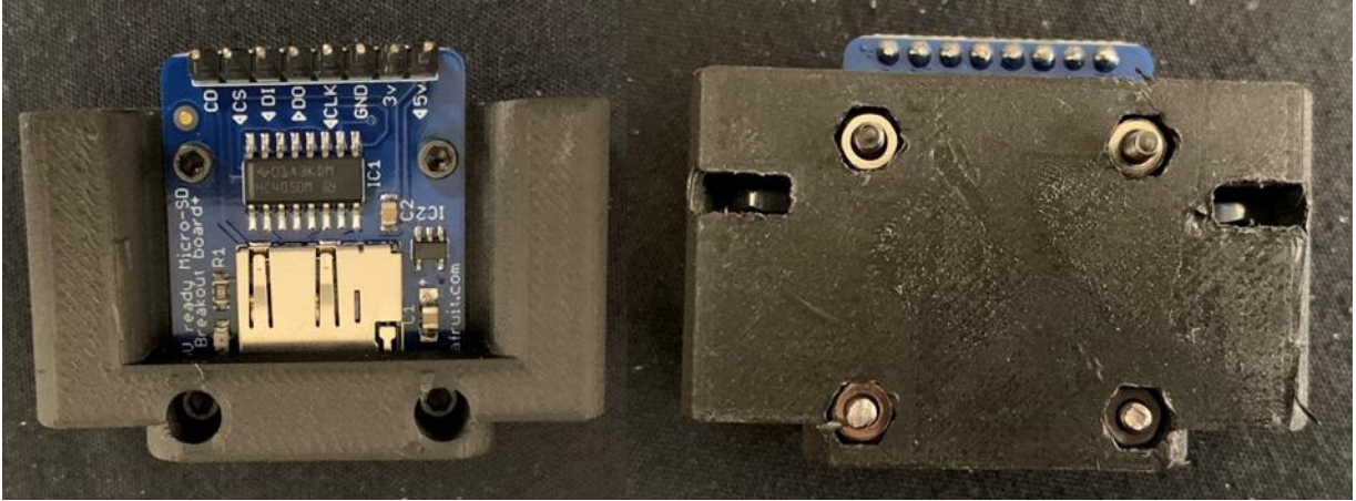
Figure 2.51 SD breakout board bolted to mounting part.
