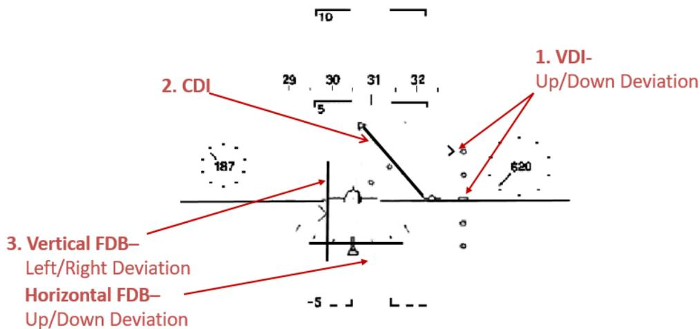
**Figure 1.1:** MIL-STD 1787 B Head-up Display. ‘A’ indicates the course deviation indicator (CDI). ‘B’ indicates the vertical deviation indicator (VDI).
