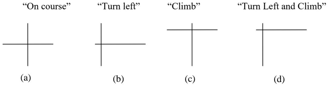
**Figure 1.3:** The flight director bars of the Mil-STD 1787B instrument landing system. Here is a depiction of what each basic position could mean.
