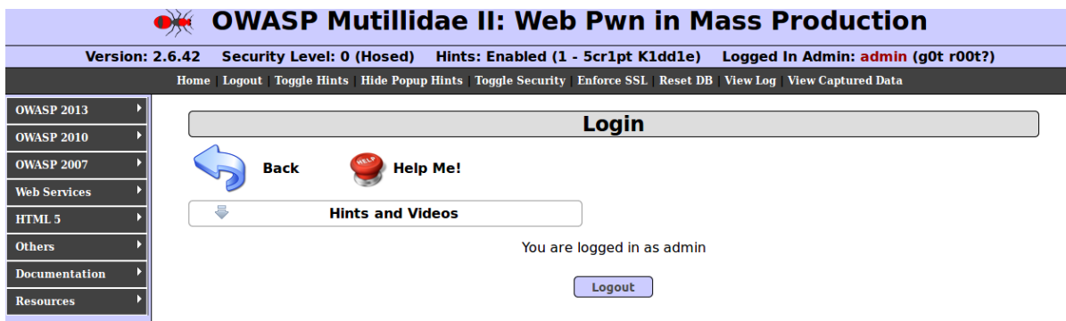
Figure 10.3: Unsecured Mutillidae Web Application Example: The tautology attack was successful. The malicious actor is logged in as admin.
