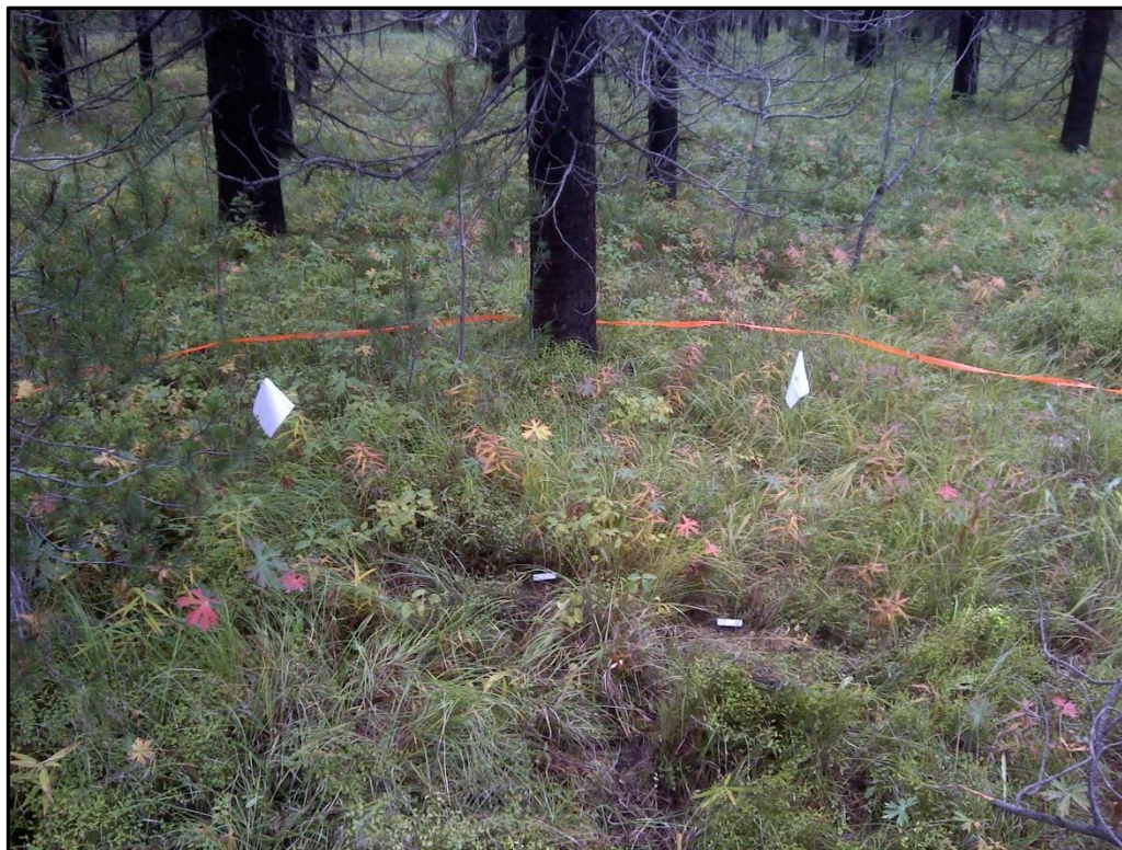
Figure 1-6 View of the understory at the north site following the installation of two soil heat flux sites. White tops of Campbell 616 soil moisture probes are visible. These mark the approximate locations of heat flux plates.
