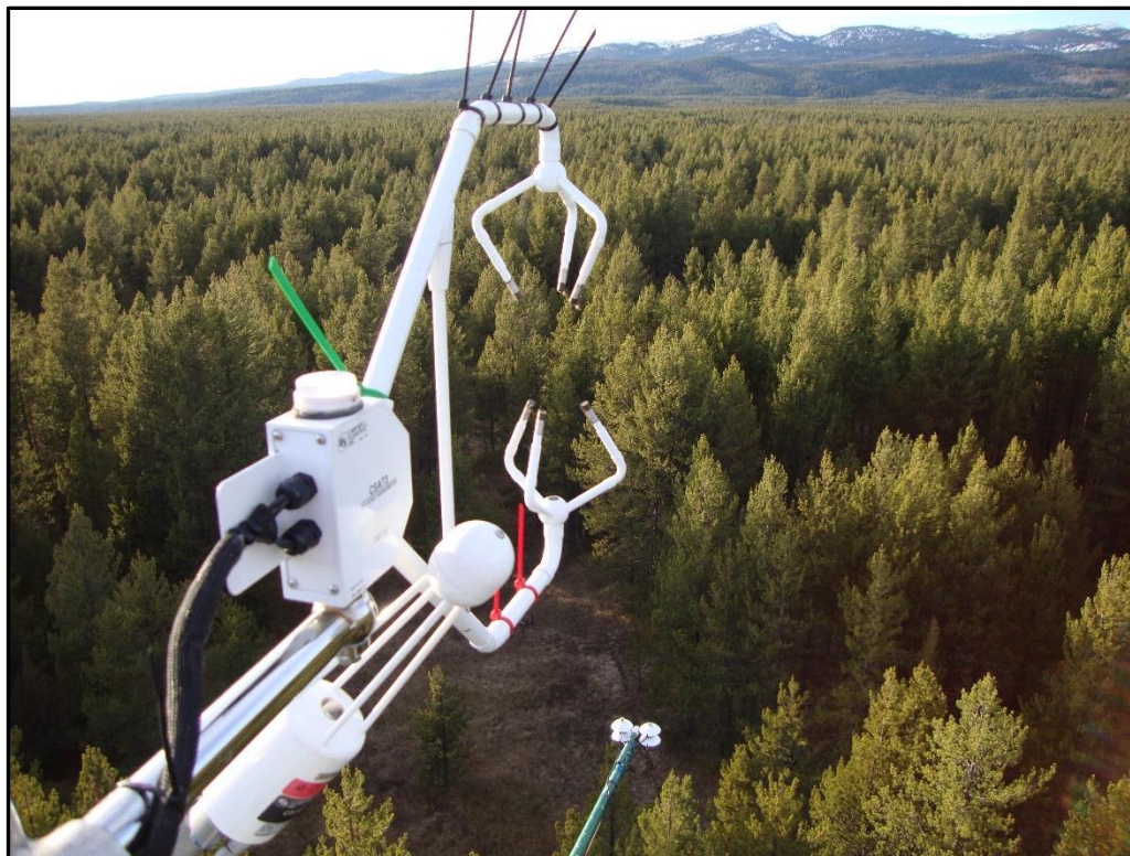
Figure 1-4. Photograph from the Island Park south tower showing typical forest canopy and the LI-COR 7500 infrared gas analyzer, CSAT 3-D sonic anemometer, and Hukseflux NR01 net radiometer mounted on the tower.
