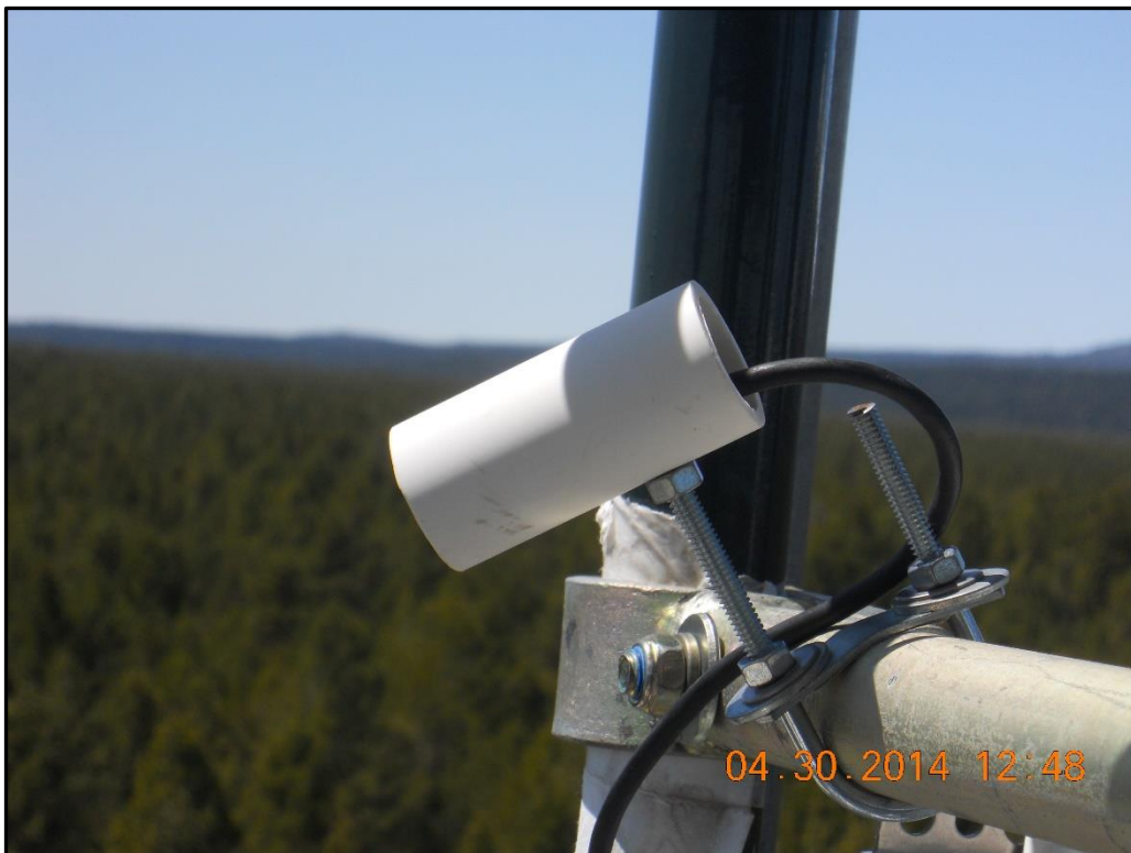
Figure 1-9. View of the infrared camera at the south site used to measure the canopy temperature to estimate canopy heat storage.
