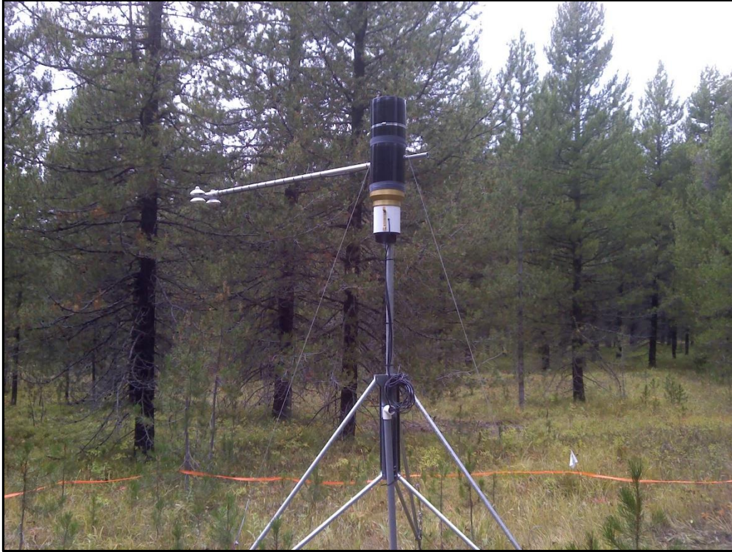
Figure 1-10. View of the Campbell Scientific TE 525WS 8-inch tipping rain gauge at the Island Park north site. A Hukseflux NR01 four-way net radiometer is also visible.
