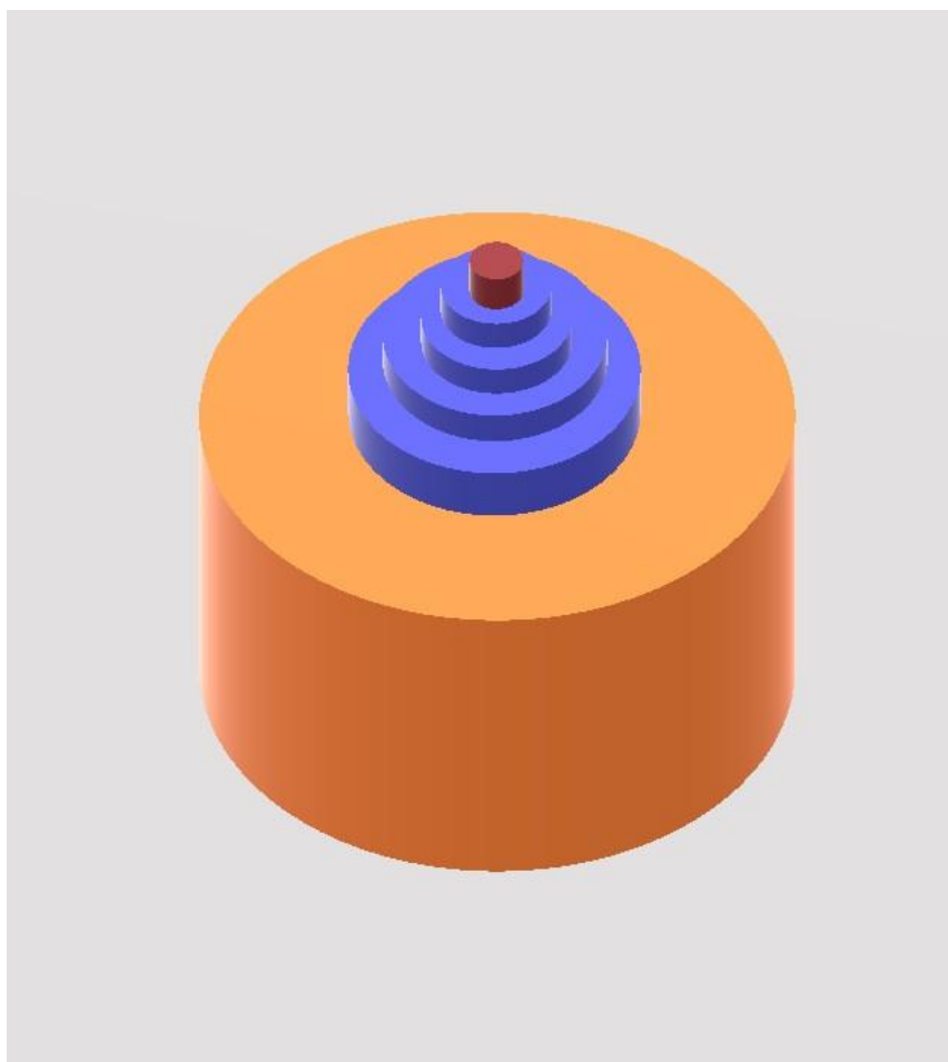
Figure 2.1: A graphical representation of drilosphere sampling scheme. The central red cylinder represents the earthworm burrow biopore (approximately 6 mm diameter, on average). Blue rings represent sampled distances (0-3, 3-6, 6-9, and 9-12 cm). The orange cylinder represents transitional soil that was not sampled (12-25 cm), and the outer edge of the orange cylinder represents the location of drilosphere sampling (bulk soil).
