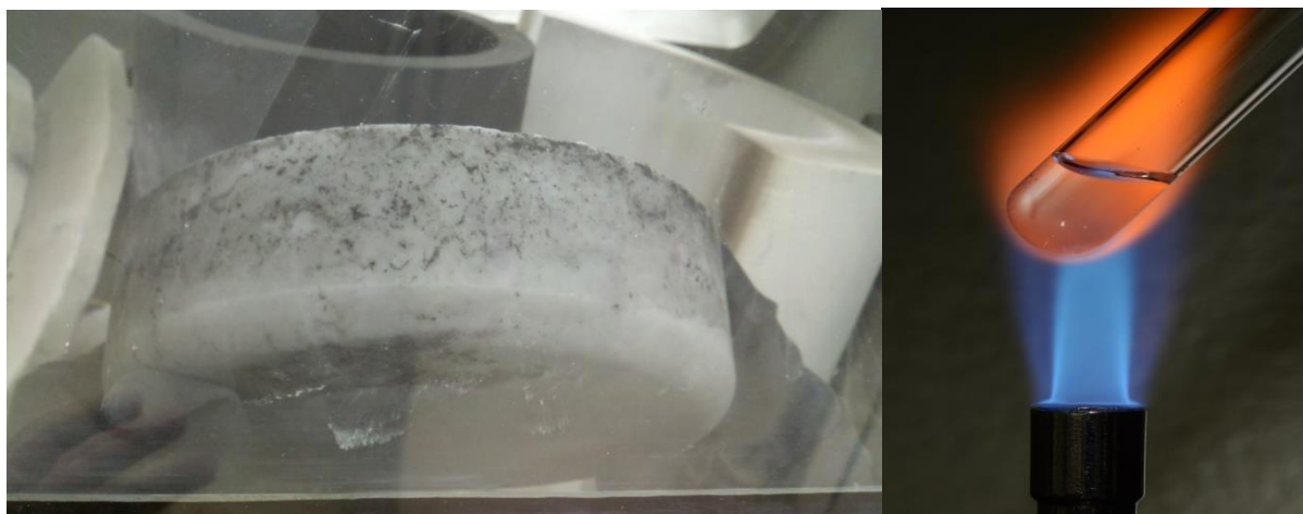
Figure 1–1 – FLiNaK Solid Castings (Left) - Molten Liquid (Right)
