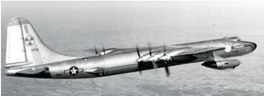
Figure 1-4 – The NB-36 – Nuclear Aircraft Powered by the ARE MSR
