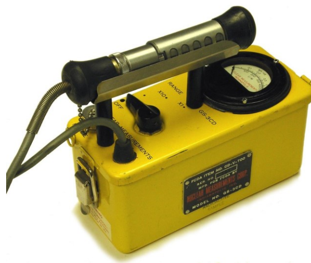
Figure 2.3 Geiger-Muller counter for radiation detection.
