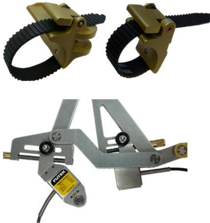
Figure 2.6. Finger cups with ratcheting straps for the middle phalanx (top left) and the proximal phalanx (top right) and finger length adjustment (bottom)
