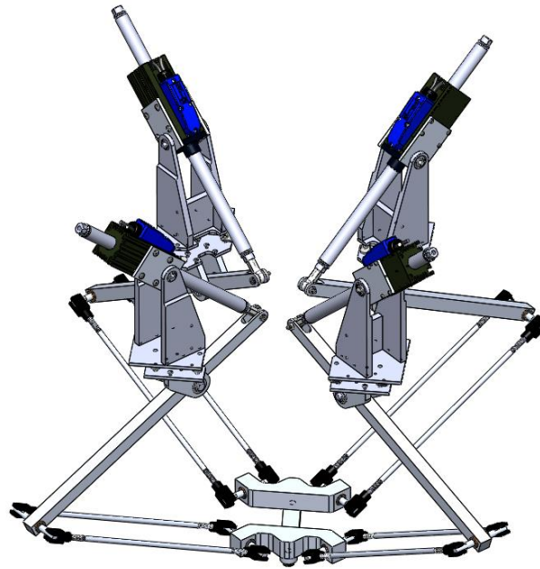
Figure 4.4. One of the kinematic chains of the robot and the counter-balance mechanism. The counter-balance torque is provided by the weight of the actuator thrust rod and the extension of Link1.
