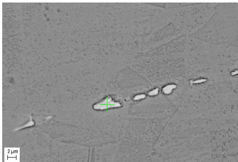
Figure 3.3. SEM SE image showing Nb rich MX precipitates found in the as-received Alloy 709
