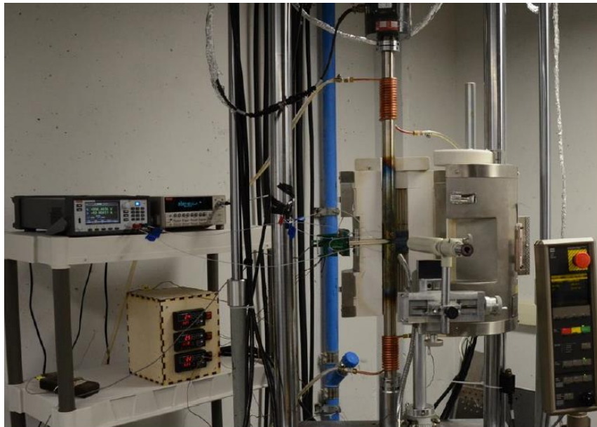
Figure 4.2. The servo-hydraulic MTS test frame used for FCG and CFCG tests.
