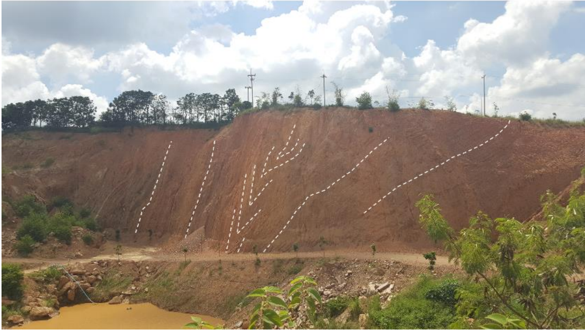
Figure 1.1 Slope face of a rock quarry in Thailand. The dashed white lines denote the bedding planes.
