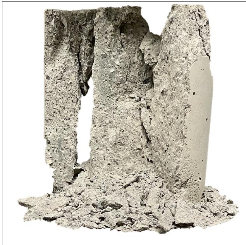
Figure 3.13 The sample failure after the compressive test.
