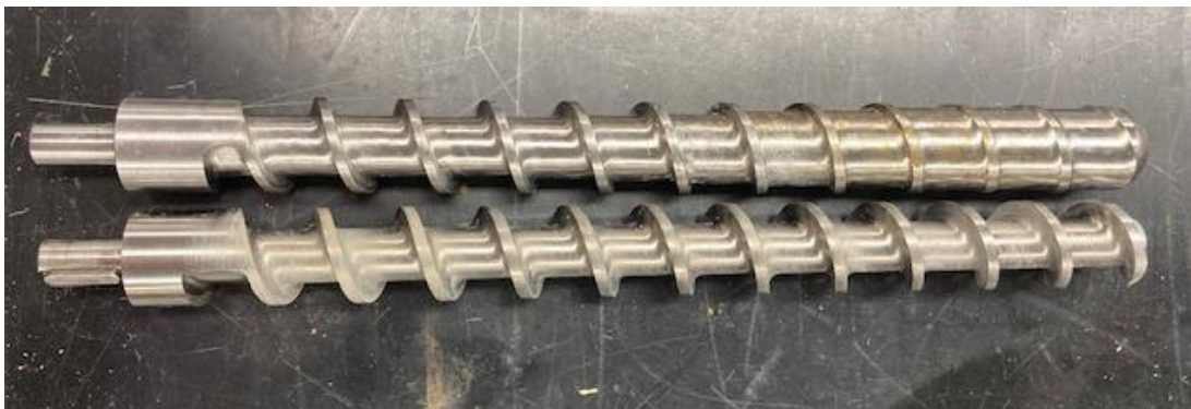
Figure 3-4: High compression screw (top) zero compression screw (bottom).
