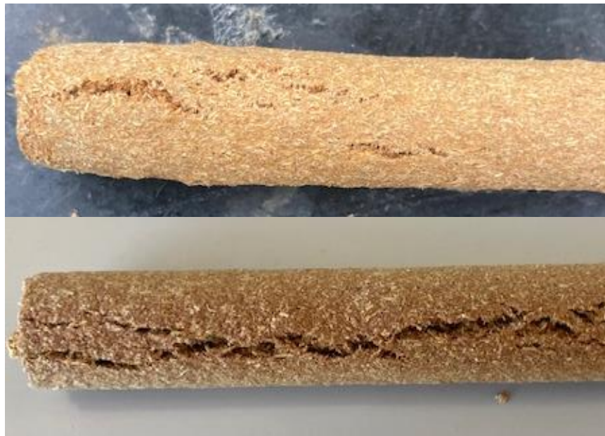
Figure 4-5: Cracked wood-resin composite samples.
