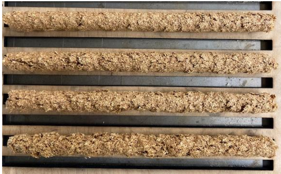
Figure 4-3: Extruded composite with wood element size of 20-40 mesh.
