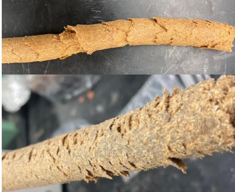
Figure 4-2: Sharkskin effect on wood-based composite.
