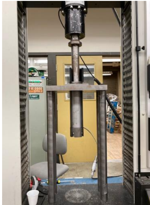
Figure 3-9: Custom rheology frame assembly.
