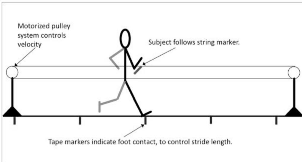
**Figure 2.1. Experimental set up.** The experimental set-up used for the stride-length manipulation trials. Subjects followed a string marker that was pulled at the correct velocity by a motorized pulley system. Stride length was controlled by having subjects match their footfall to tape markers placed on the floor.
