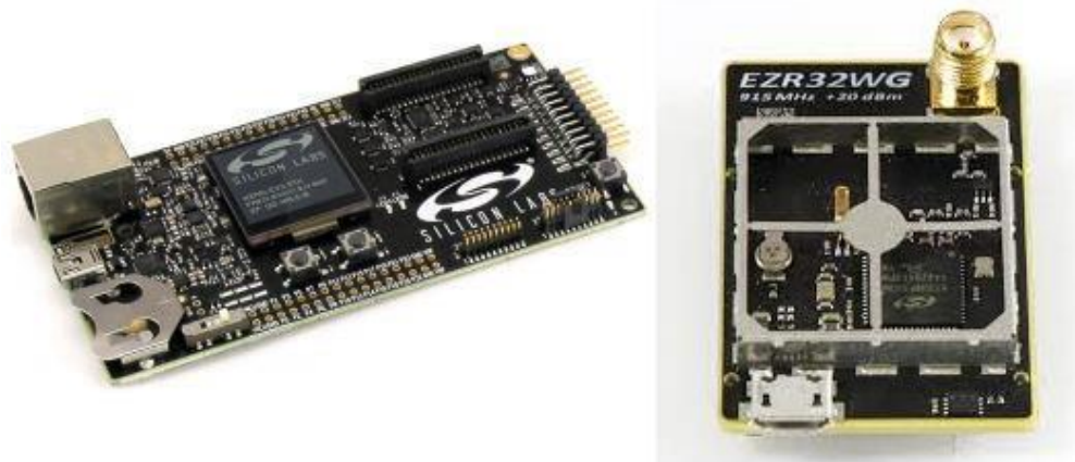
Figure 3.8: The BRD4503B Board (Left) and BRD4001A Board (Right) Combined Make up the SLWSTK6222A Development Kit.
