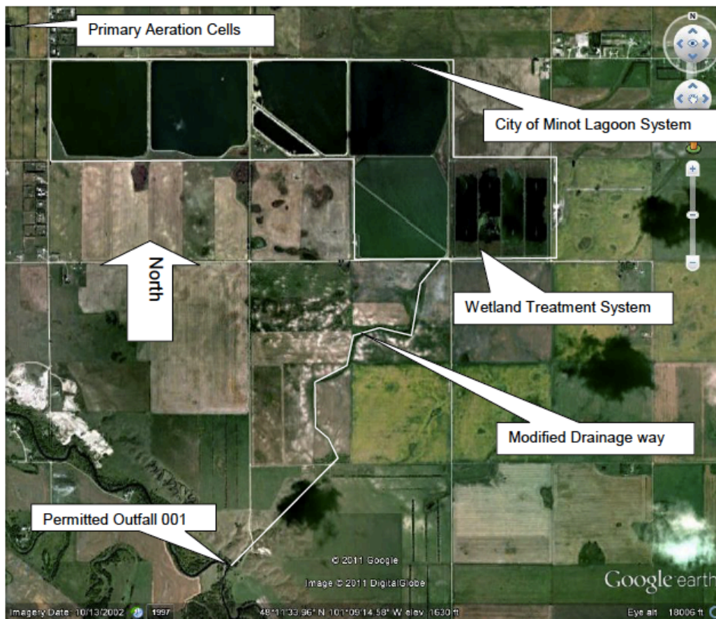
Figure 17. Aerial map of Minot, North Dakota, wastewater treatment works. Google Earth, 2018.
