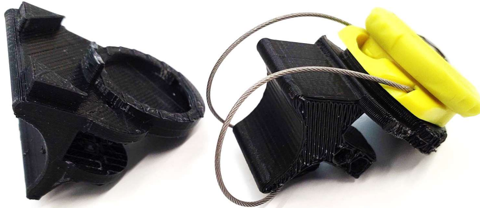
Figure 3.2. Initial middle and proximal cuff prototypes using the BOA ® S2-S dial. The proximal cuff has the BOA ® S2-S dial attached.
