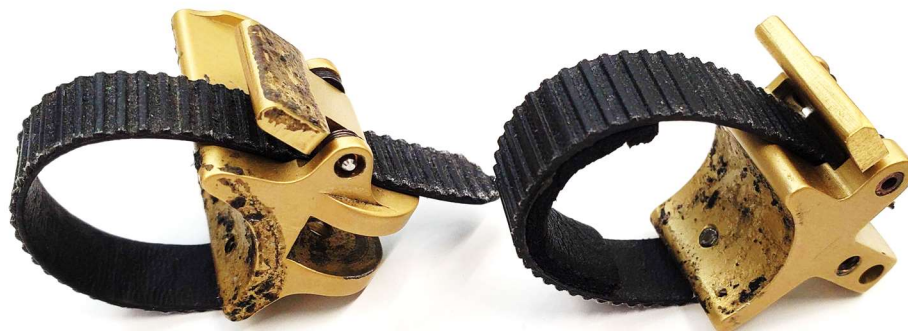
Figure 3.1. Proximal (right) and middle (left) cuffs currently employed on FINGER. The original foam padding has been removed.
