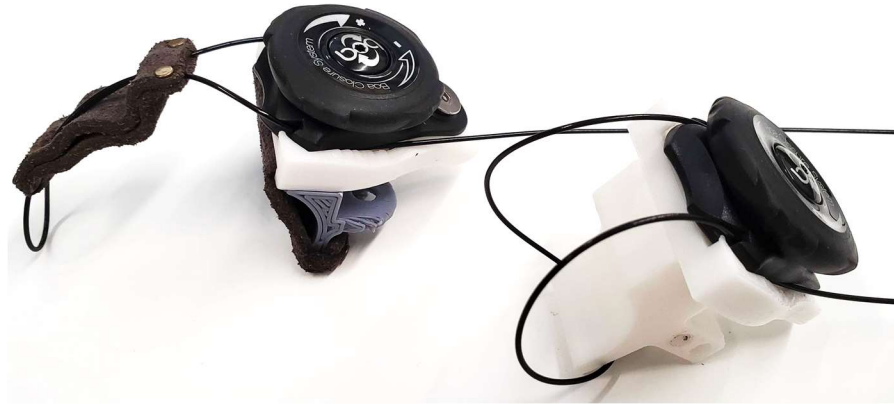
Figure 3.4. Final prototypes using the BOA ® S2 dials. The left cuff has the leather cable cover and leather base cover attached.
