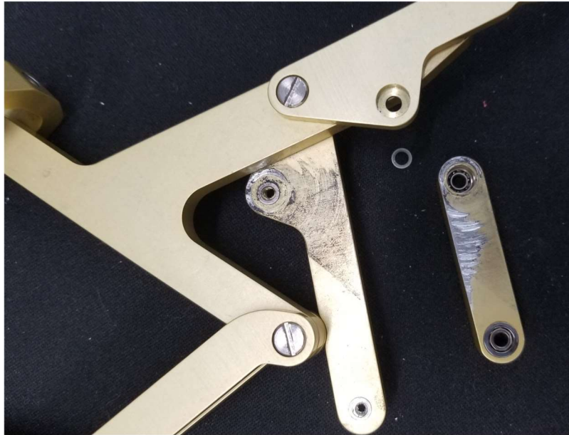
Figure 2.2: Damaged links on the FINGER robot. The link showing wear on the right was missing a shim and the bearing and was rubbing against the nearby links.
