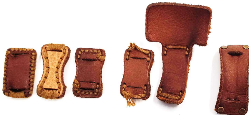
Figure 3.3. Evolution of cable-cover designs. Initial designs (left) of the cable covers used sewn seams, later prototypes used rivets (right). The 2 nd from the right shows the extended leather cover.
